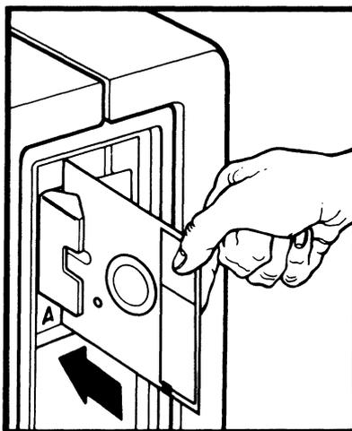
3. With the diskette securely in the drive, close the door by pushing on the outside of the open door. If the door does not close easily, make sure the diskette is fully inserted.
