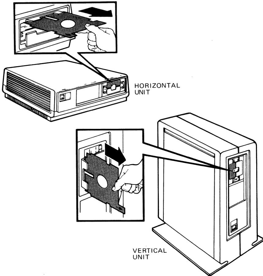
The protective card prevents the drive components from moving during shipment. Be sure to save it to use later if you move the computer.
