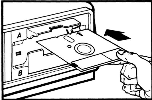
3. With the diskette securely in drive A, close the drive door by pushing on the outside of the open door. If the door does not close easily, make sure the diskette is fully inserted.
