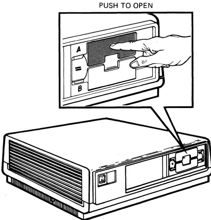
2. Open drive B by pushing on the **bottom** of the drive door.
