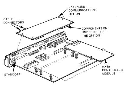
Installing the Extended Communications Module in the Rainbow 100B or Rainbow 100 System Unit
