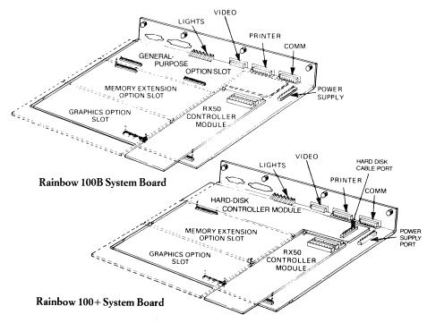
Mounted on the system board is the RX50 controller module, which controls reading and writing on the floppy-diskette drive. The Rainbow 100+ also has a hard-disk controller module, which controls reading and writing on its hard-disk drive. In addition, the system board has areas dedicated for mounting option modules to further extend the capabilities of your Rainbow 100B or Rainbow 100+.
