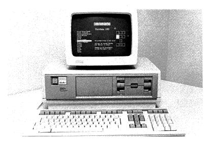
The Rainbow 100+ has all the outstanding features of the Rainbow 100B plus more. It includes an internal 10-Mbyte hard disk as a standard feature. The internal 10-Mbyte hard disk lets you transfer and access files faster and keep your programs on one hard disk. That means no more swapping floppies.
