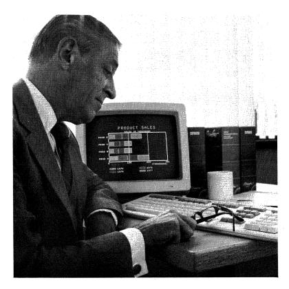
The color monitor combines elegant styling and user-oriented design with advanced video technology. The high bandwidth of the monitor (18-20 MHz) allows the display of either 80 or 132 columns by 24 rows of high-quality text characters, or high-resolution bit-mapped graphics. These precise displays far surpass the video quality of competitive personal computer monitors.
