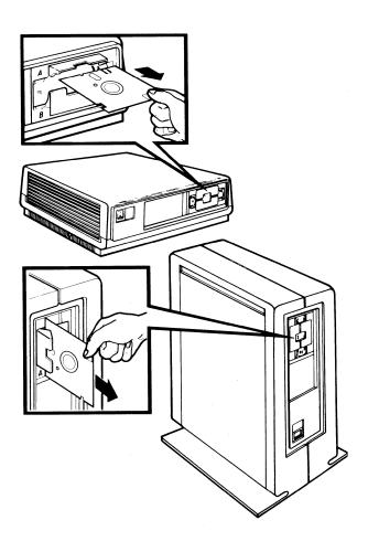
Inserting Diskette into Drive A
