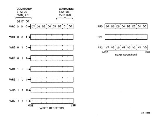
Figure 3-17 MPSC Command/Status Registers (Each Channel)
