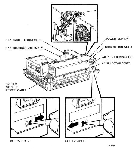
Figure 5-2 Power Supply and Fan Bracket Assembly
