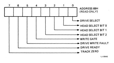
Figure 4-17 Drive Status Register Format
