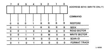
Figure 4-13 Command Register Format
