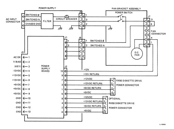
Figure 5-3 Power Supply and Fan Assembly Cabling
