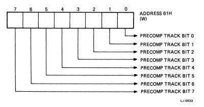
Figure 4-7 Write Precompensation Register Format
