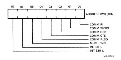
Figure 3-11 Communications Status Register (8088) Format
