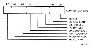
Figure 3-9 Diagnostic Write Register (8088) Format
