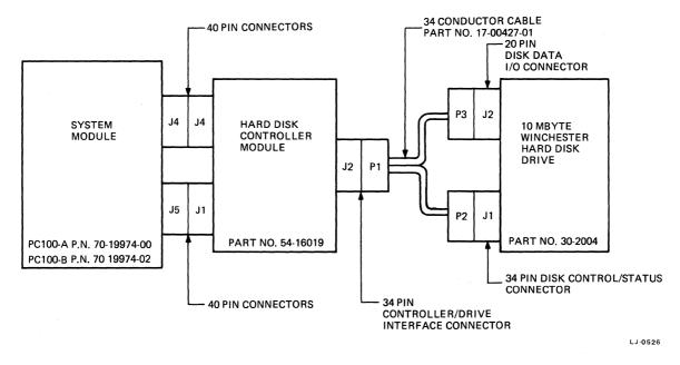
Figure 4-1 Winchester Subsystem Connections
