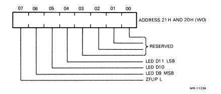
Figure 3-14 General/Diagnostic Control Register (Z80A) Format
