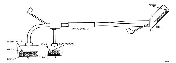
Figure 4-3 Controller/Hard Disk Interconnect Cable
