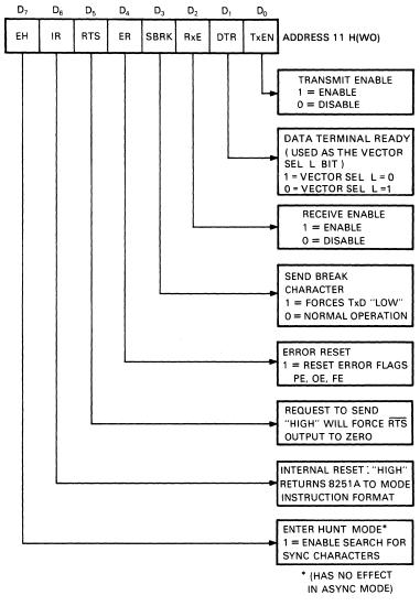
NOTE: ERROR RESET MUST BE PERFORMED WHENEVER RXENABLE AND ENTER HUNT ARE PROGRAMMED.
