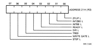
Figure 3-13 General/Diagnostic Status Register (Z80A) Format
