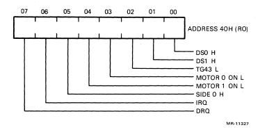
Figure 3-15 Disk Drive Status Register (Z80A) Format
