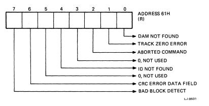
Figure 4-6 Error Register Format
