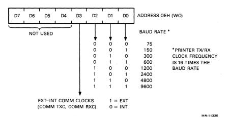
Figure 3-22 Printer Baud Rate Register Format
