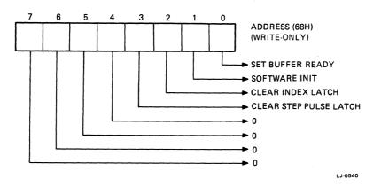
Figure 4-15 Secondary Command Register Format
