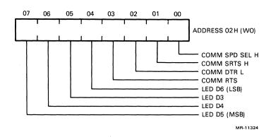
Figure 3-12 Communications Control Register (8088) Format
