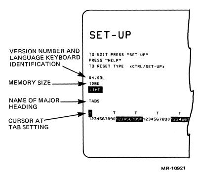
Figure 2-7 Tabs Set-Up Menu
