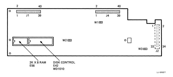
Figure 4-2 RD51 Controller Module Physical Layout
