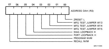
Figure 3-10 Diagnostic Read Register (8088) Format
