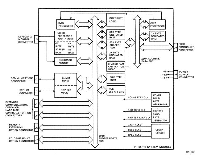
Figure 3-1 PC100-B System Module Block Diagram
