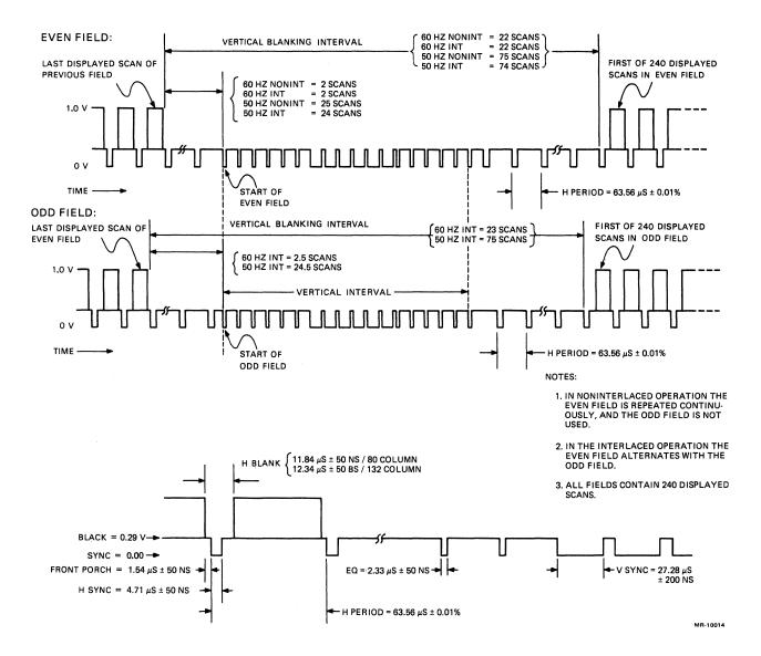
Figure 3-7 Composite Video Synchronous Timing Diagram
