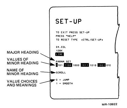
Figure 2-8 Parameter Settings Set-Up Menu
