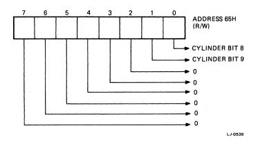
Figure 4-11 Cylinder High Register Format
