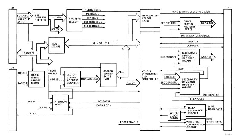
Figure 4-4 Hard Disk Controller Module
