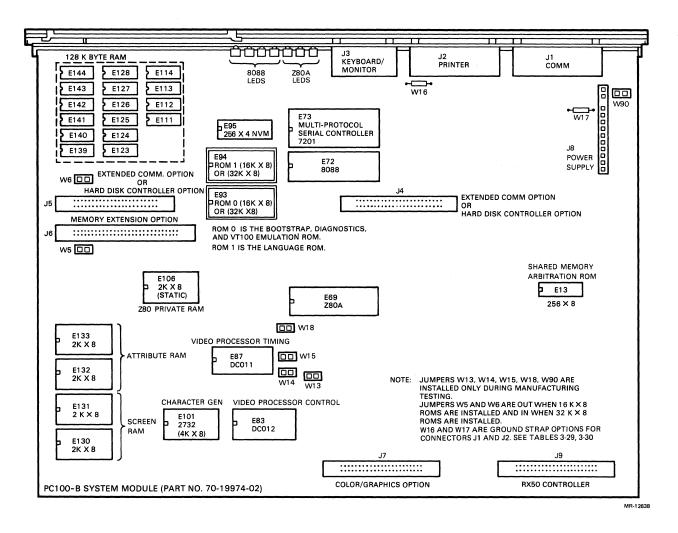
Figure 3-2 PC100-B System Module Physical Layout
