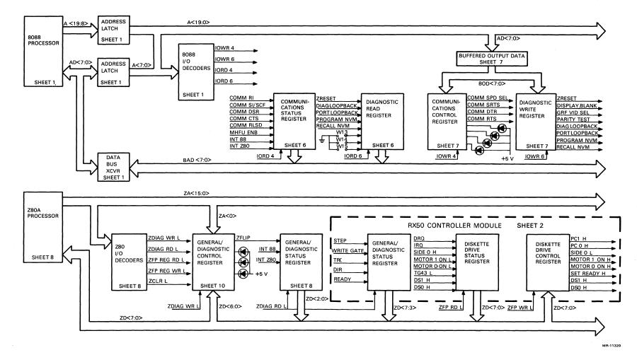
Figure 3-8 System Module Control/Status and Diagnostic Registers
