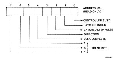
Figure 4-16 Secondary Status Register Format
