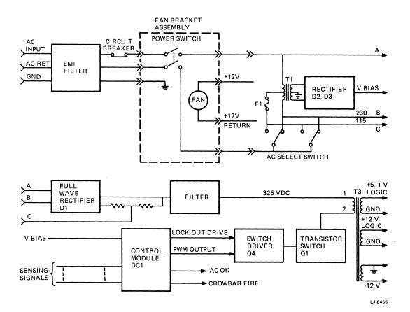
Figure 5-4 Power Supply Functional Diagram
