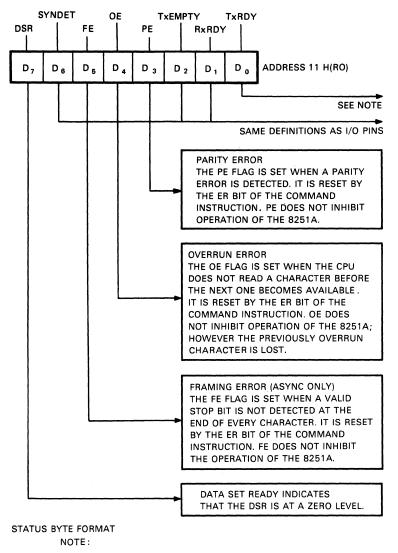
TxRDY STATUS BIT HAS DIFFERENT MEANINGS FROM THE TxRDY OUTPUT PIN. THE FORMER IS NOT CONDITIONED BY CTS AND TXEN; THE LATTER IS CONDITIONED BY BOTH CTS AND TXEN. i.e. TXRDY STATUS BIT = DB BUFFER EMPTY
