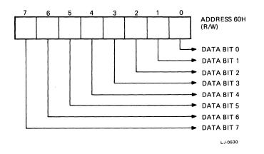
Figure 4-5 Data Buffer Register Format
