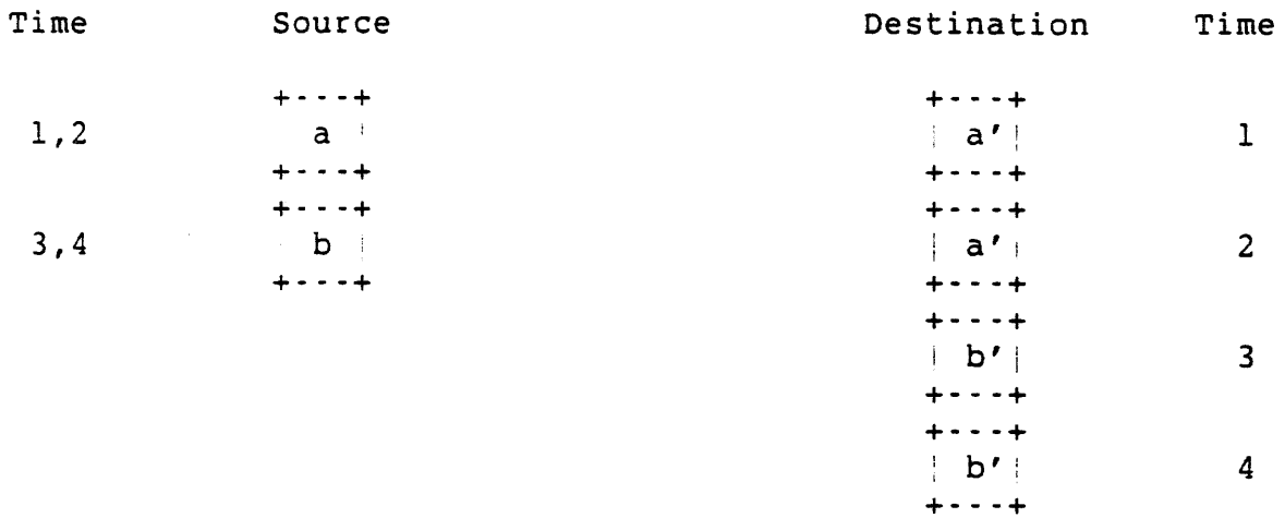
Figure 4-23 Scaling Up The Source By Two
