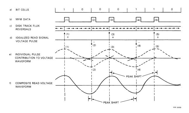
Figure 2-11 Peak Shift Waveform
