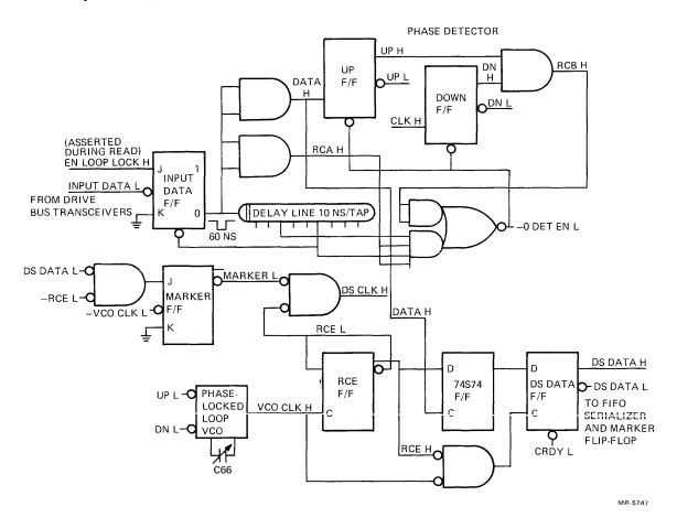
Figure 2-13 Data Separator Read Circuit
