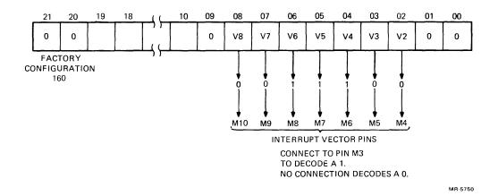
Figure 3-3 RLV12 Interrupt Vector Format
