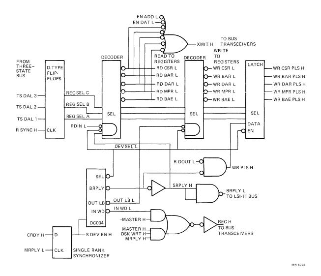
Figure 2-2 Bus Protocol Logic
