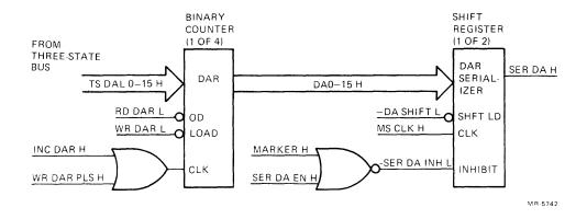
Figure 2-6 Disk Address Register (DAR) Circuit
