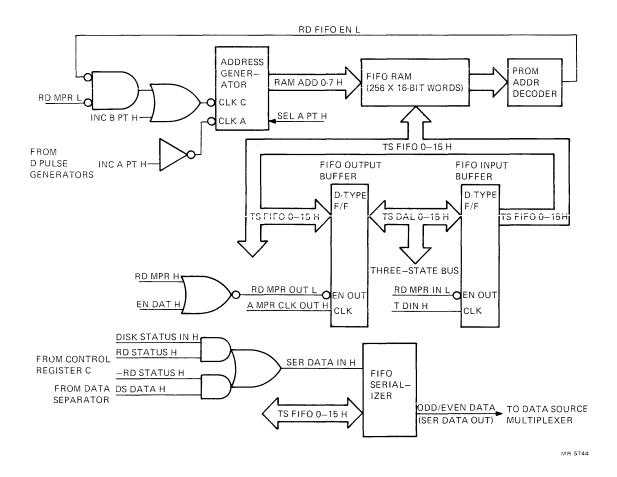
Figure 2-8 FIFO RAM, Buffers, and Serializer
