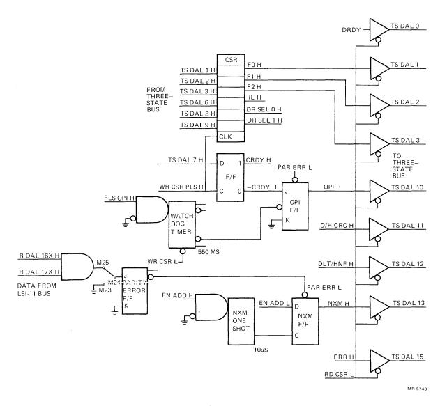
Figure 2-7 Control/Status Register (CSR) Circuit
