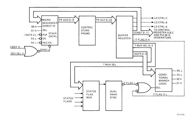
Figure 2-9 Microsequencer, Control Store PROMs, and Buffer Register
