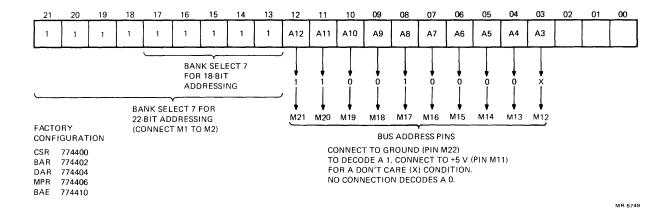
Figure 3-2 RLV12 Device Address Format
