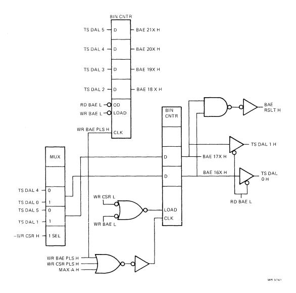
Figure 2-5 Bus Address Extension Register (BAE) Circuit
