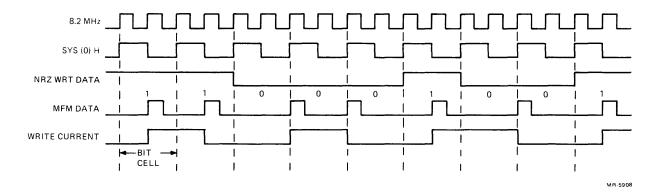
Figure 2-10 MFM Encoding
