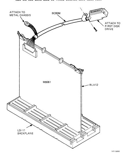
Figure 3-4 RLV12 Installation
