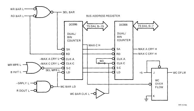
Figure 2-4 Bus Address Register (BAR) Circuit
