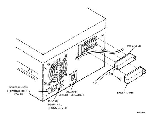
Figure 6-2 RL01/RL02 Disk Drive (Rear View)
