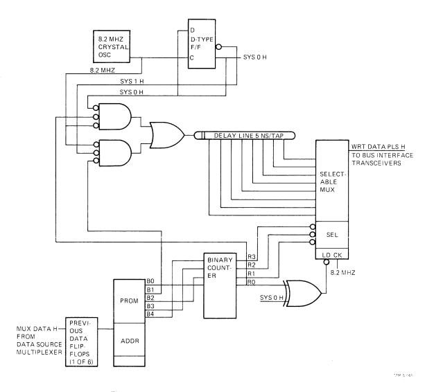
Figure 2-12 Write Encoder and Precompensation Circuit
