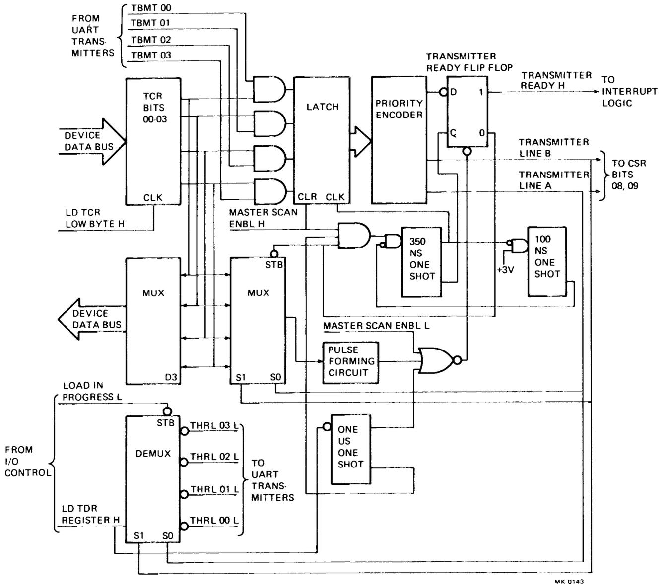
Figure 5-24 Transmitter Control
