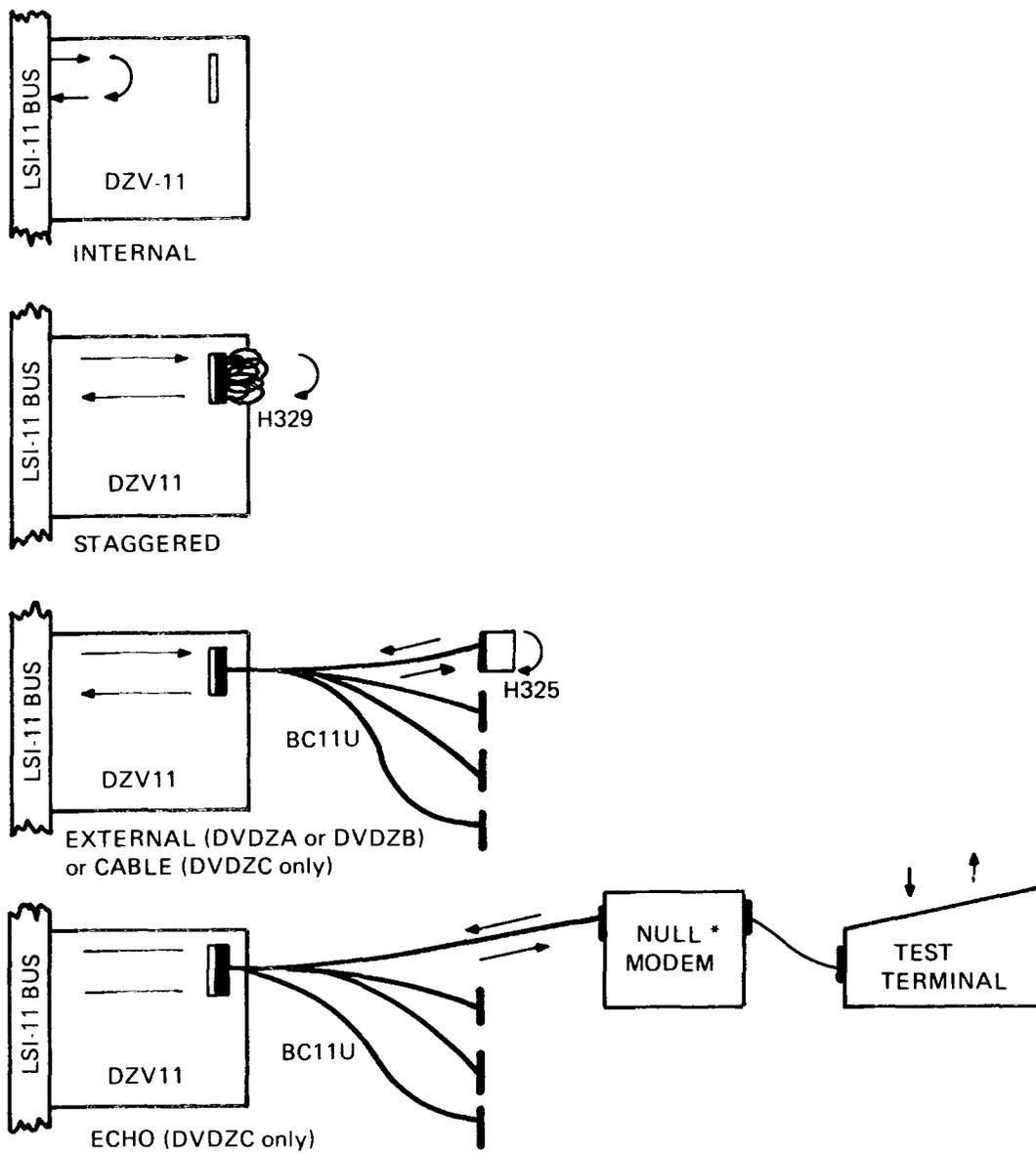
\* A NULL MODEM, SUCH AS AN H312, MAY BE NECESSARY, DEPENDING ON THE TERMINAL USED FOR TEST.
