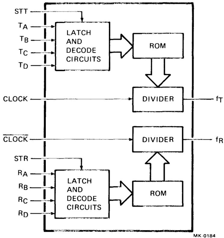
Figure A-13 COM 5016 Simplified Block Diagram
