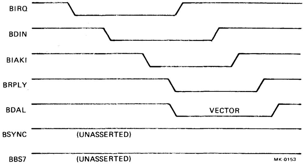
Figure 5-16 Interrupt Timing
