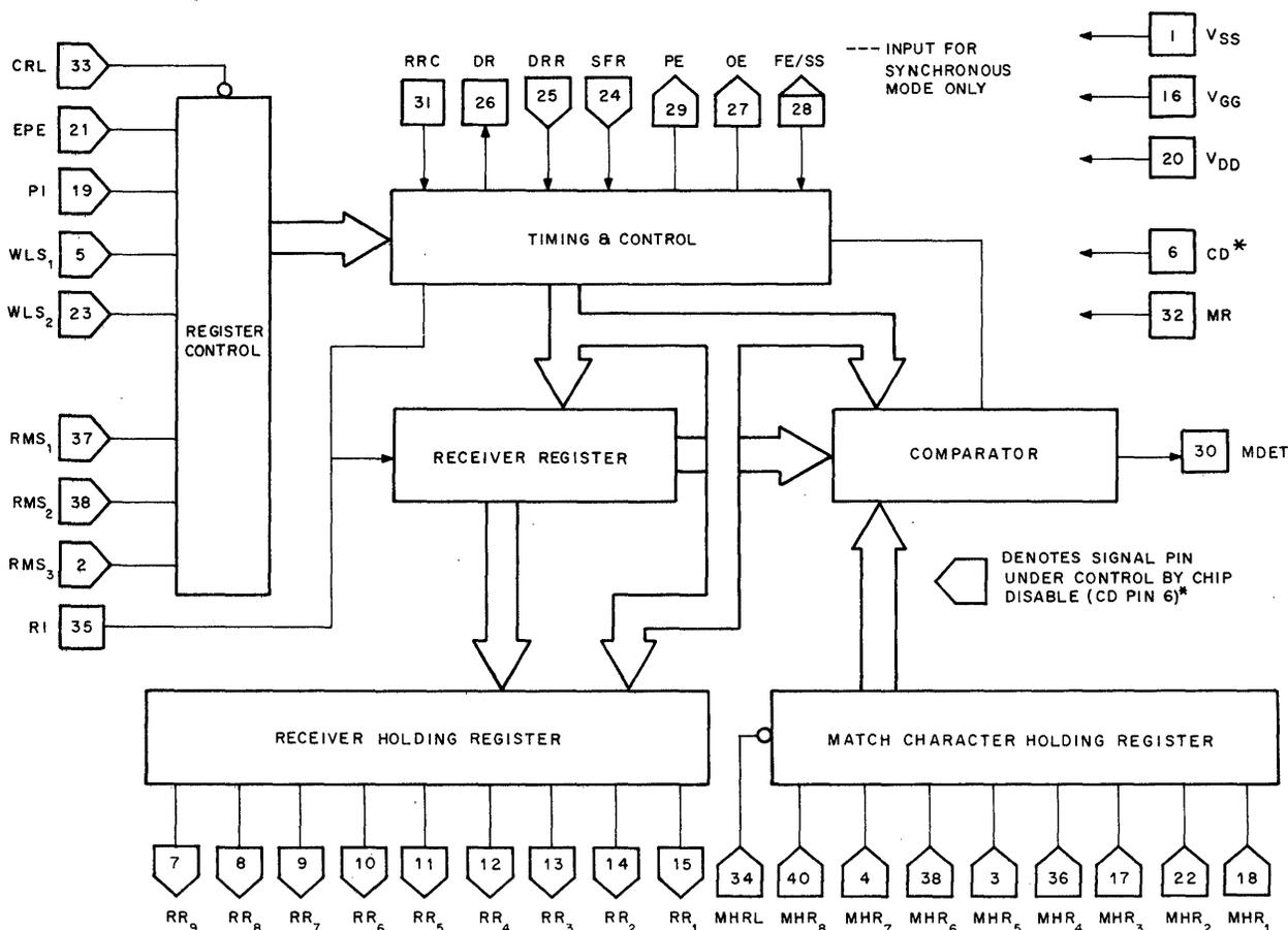
Figure B-1 PR1472B Programmable Synchronous Receiver (P/SAR)
