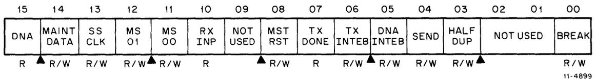
**Figure 3-5 Transmitter Status Register (TXCSR)**
