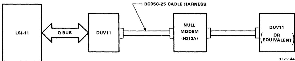
Figure 2-4 DUV11 to Null Modem Connection
