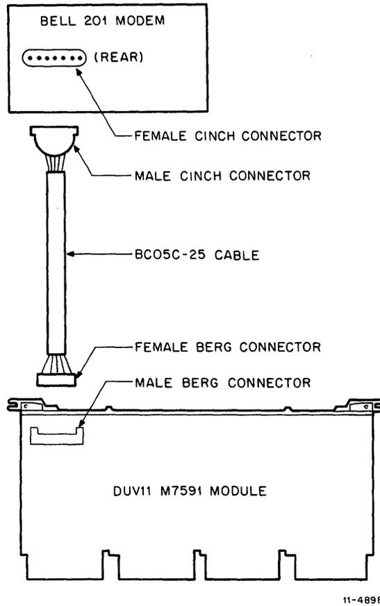
Figure 2-3 DUV11 to Modem Connection
