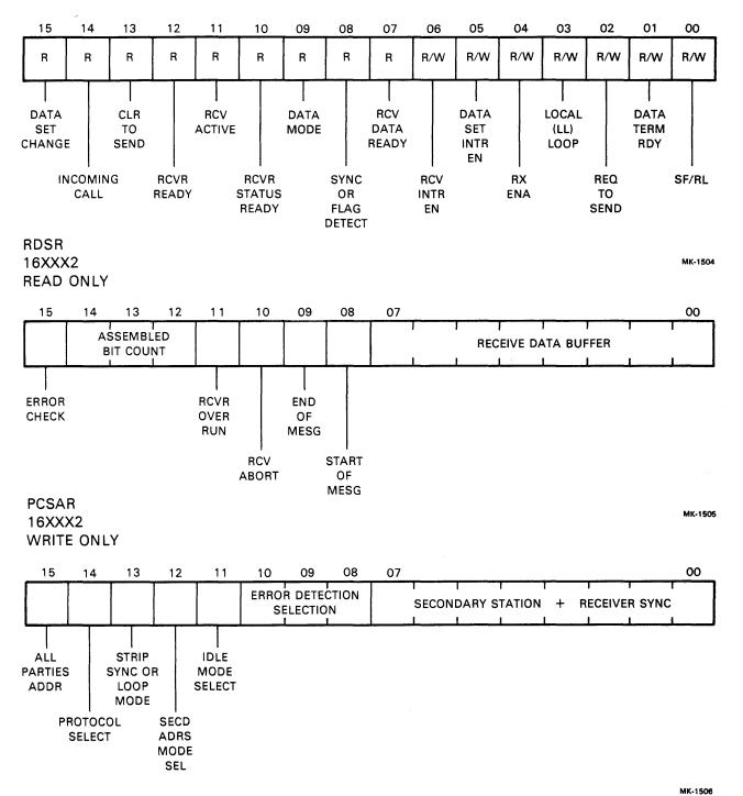
Figure 3-1 DPV11 Register Configurations and Bit Assignments (Sheet 1 of 2)
