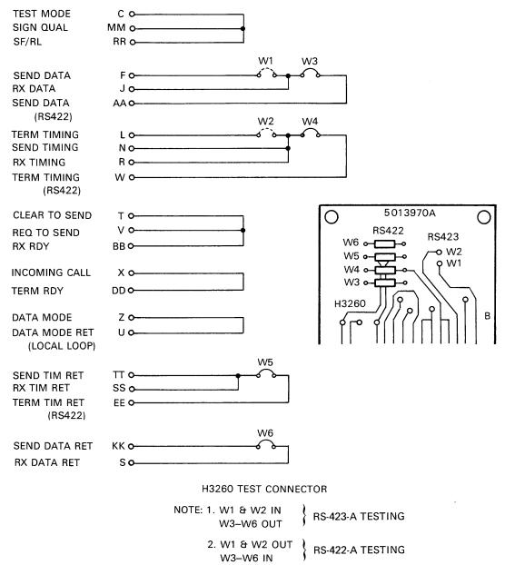
Figure 2-4 H3260 On-Board Test Connector
