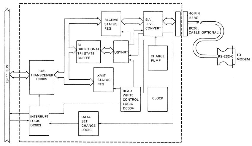
Figure 4-1 DPV11 Block Diagram
