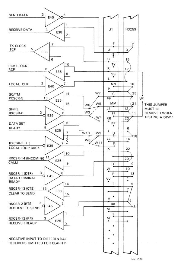
Figure 2-3 RS-423-A with H3259 Test Connector
