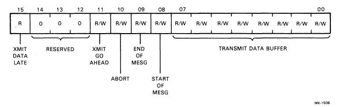
Figure 3-1 DPV11 Register Configurations and Bit Assignments (Sheet 2 of 2)
