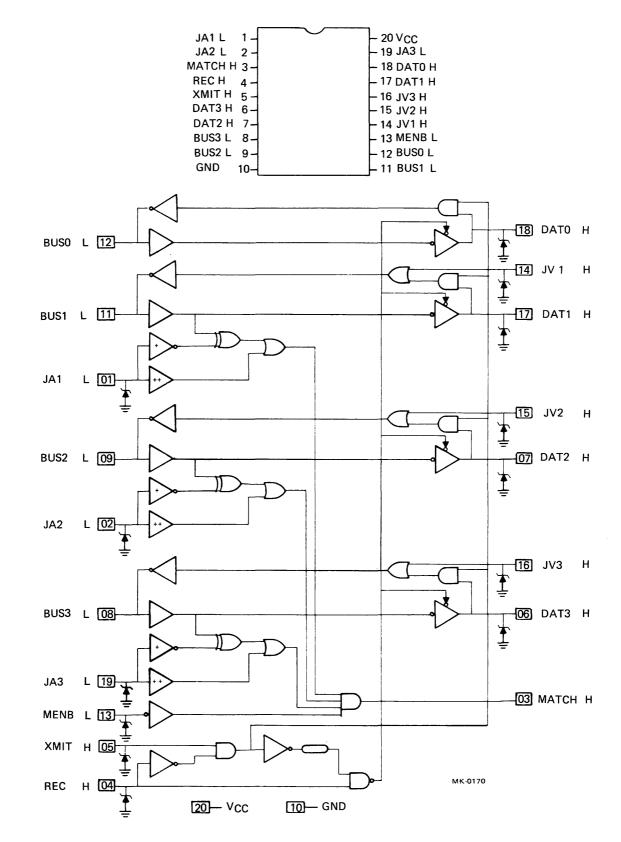
Figure C-3 DC005 Simplified Logic Diagram
