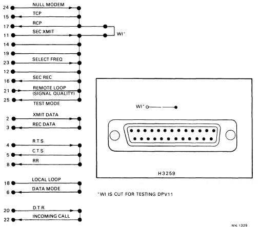
Figure 2-2 H3259 Turn-Around Test Connector
