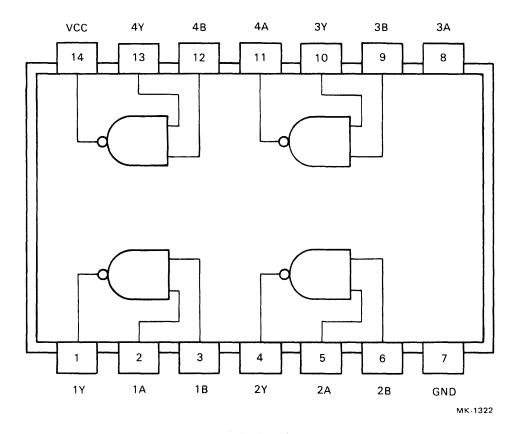
Figure C-6 8881 Pin Identification
