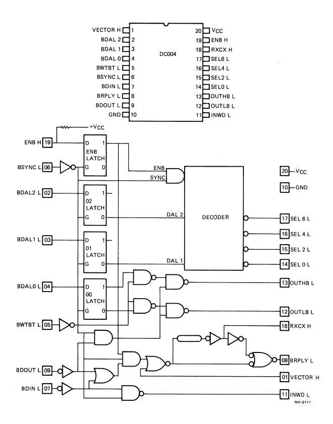
Figure C-2 DC004 Simplified Logic Diagram
