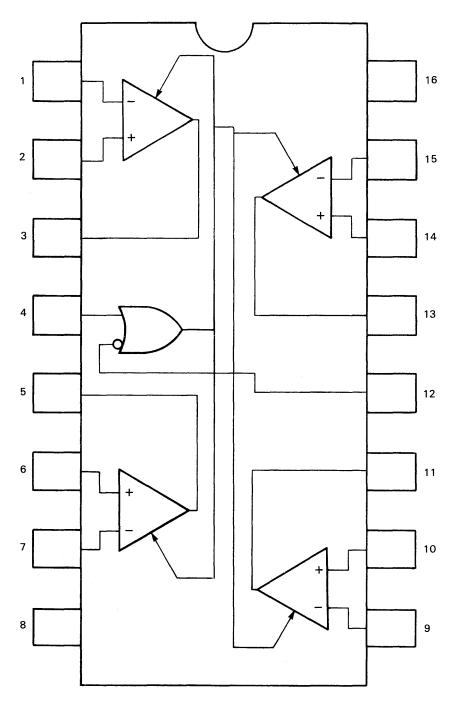
NOTE: PIN 1 IS MARKED FOR ORIENTATION. NUMBERS INDICATED DENOTE TERMINAL NUMBERS. TERMINAL IDENTIFICATION
