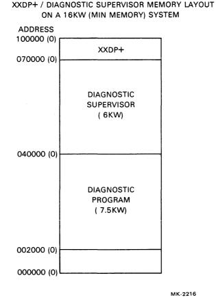
Figure A-1 Typical XXDP+/Diagnostic Supervisor Memory Layout
