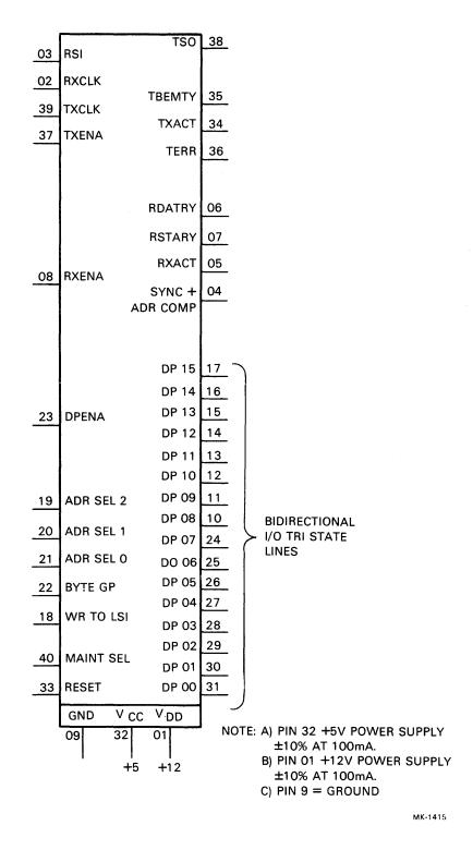
Figure B-1 Terminal Connection Identification Diagram (2112517-0-0 Variation)
