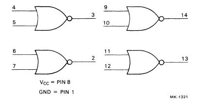
Figure C-5 8640 Equivalent Logic Diagram
