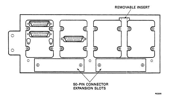
Figure 2-8 I/O Insert Panel (DEC423)
