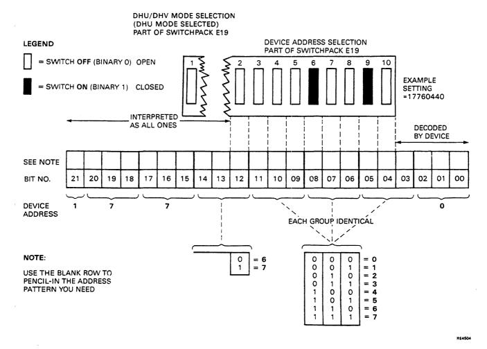
Figure 2-2 Setting the Device Address
