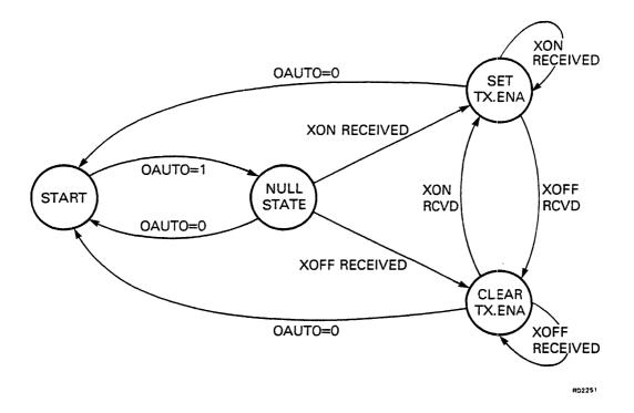
Figure C-1 Transmitted Data Flow Control
