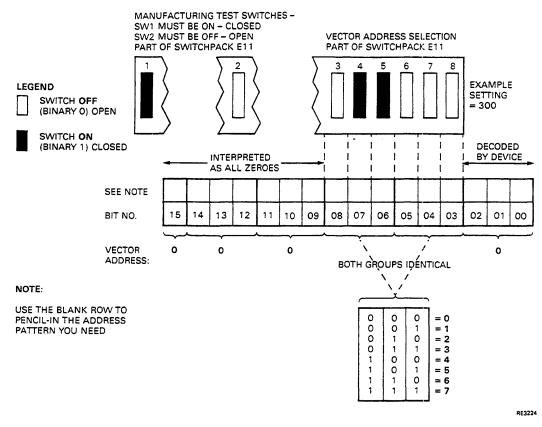
Figure 2-3 Setting the Vector Address
