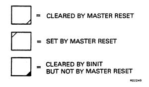
Figure 3-1 Register Coding
