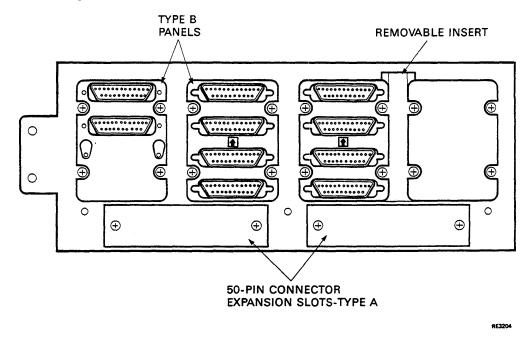
Figure 2-7 I/O Insert Panels and Adapter Plate (EIA-232-D)
