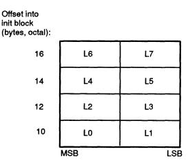
Where: L0 through L7 are the most significant to least significant bytes, respectively, in the logical address filter.
