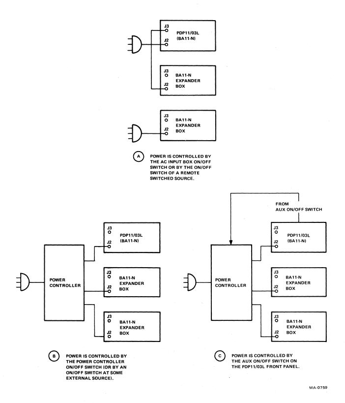
Figure 2-7 Power Connections, PDP-11/03L Systems
