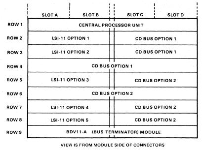
Figure 1-9 Module Installation in the H9273 Backplane
