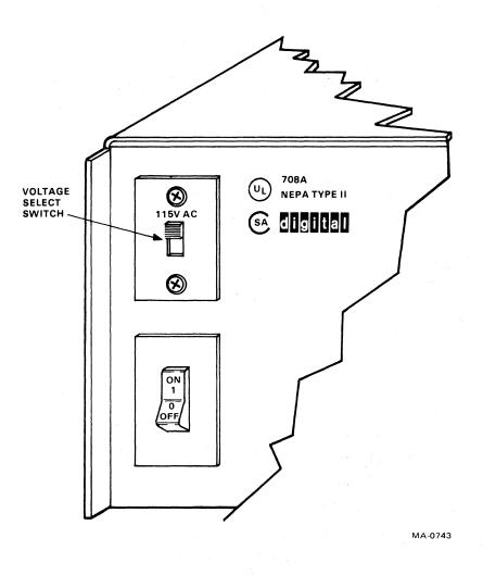
Figure 2-1 BA11-N Voltage Select Switch
