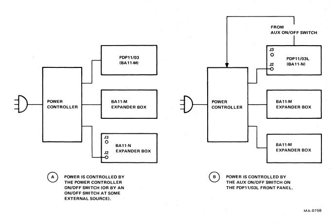
Figure 2-8 Power Connections with BA11-M Expander Boxes
