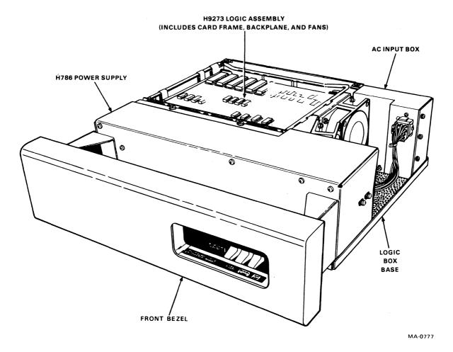
Figure 1-3 BA11-N, Logic Box Cover Removed
