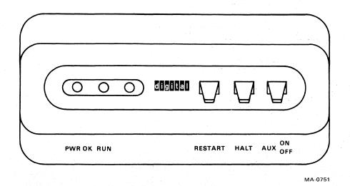
Figure 2-9 Front Panel Switches and Indicators
