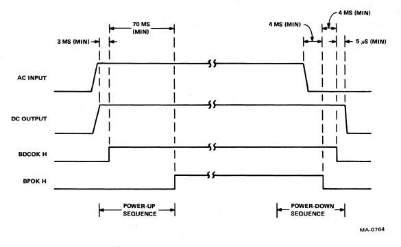
Figure 1-11 Power Up/Power Down Timing
