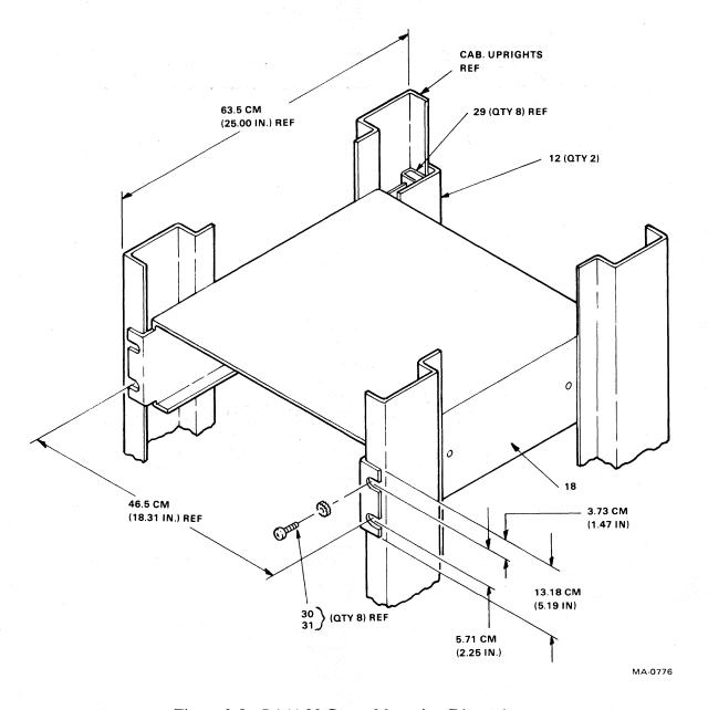
Figure 2-5 BA11-N Cover Mounting Dimensions
