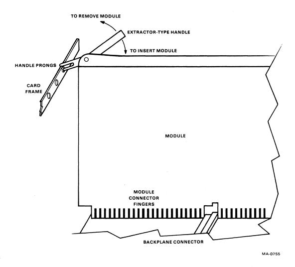
Figure 2-4 Insertion and Removal of Modules Having Extractor-Type Handles
