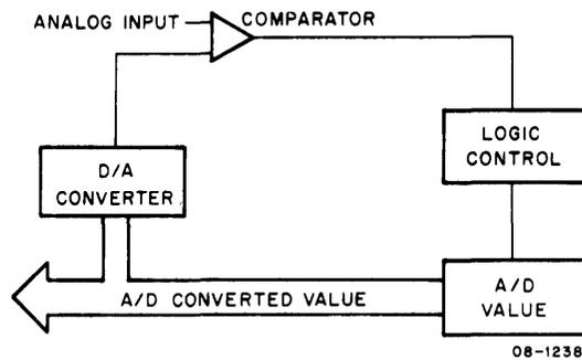
An analog signal is compared to a logic generated signal. The logic always supplies a half range signal initially. For example, the full scale input to an A/D converter system is 10 V and the input to the system is 7 V.
