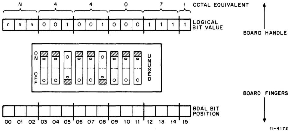
Figure 4-5 AAV11-A Address Switches (set for 17044n)
