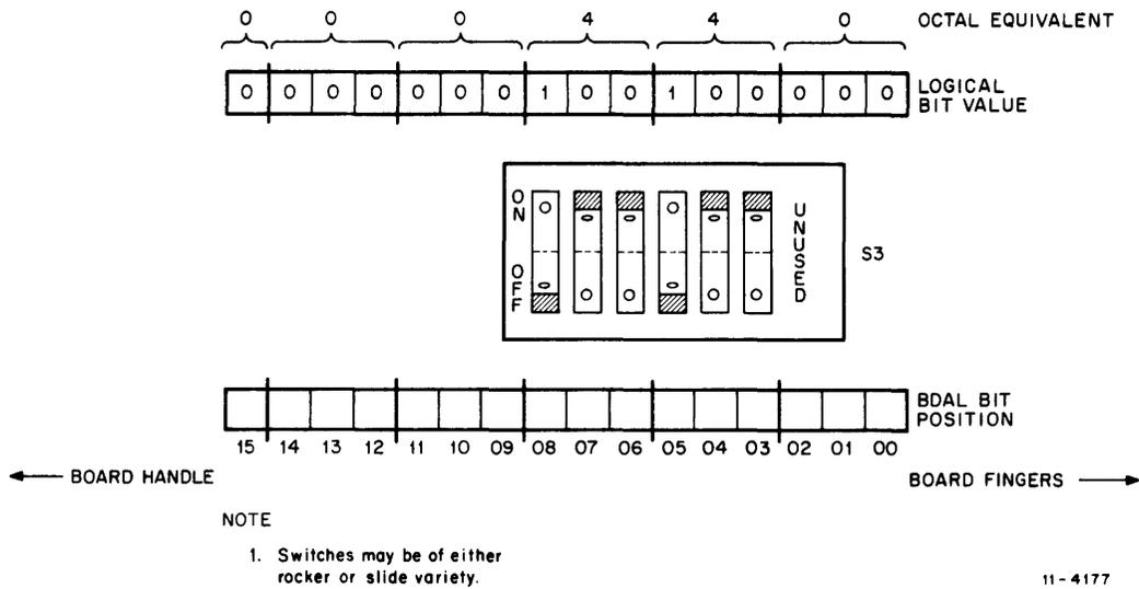
Figure 3-6 KVV11-A Vector Address Switches (Set for 000440)
