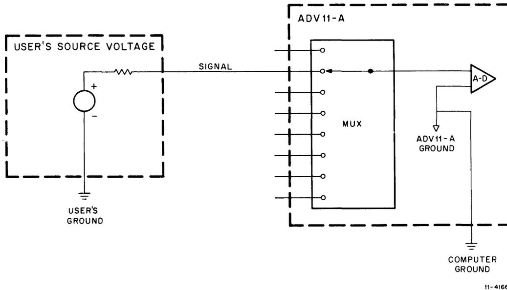
Figure 2-2 Single-Ended Input Referenced to User's Ground
