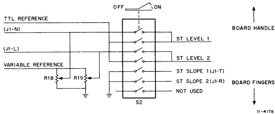
Figure 3-7 KVV11-A Slope/Reference Level Selector Switches and Controls
