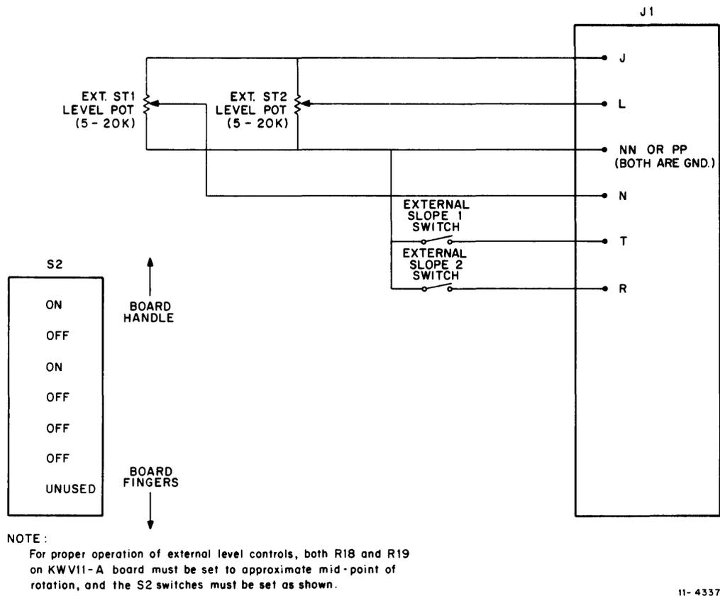
Figure 3-3 Connecting External User-Supplied Slope and Level Controls
