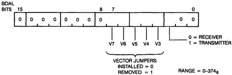
Figure 21-3 ■ DLV11 Interrupt Vector Address Selection
