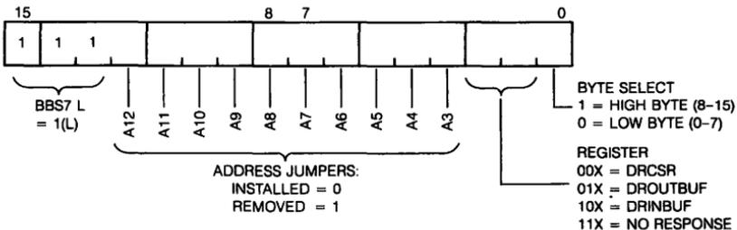
*Figure 38-2 • DRV11 Device Address Selection*
