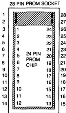
Figure 11-4 ■ Insertion of 24-Pin PROM Chips
