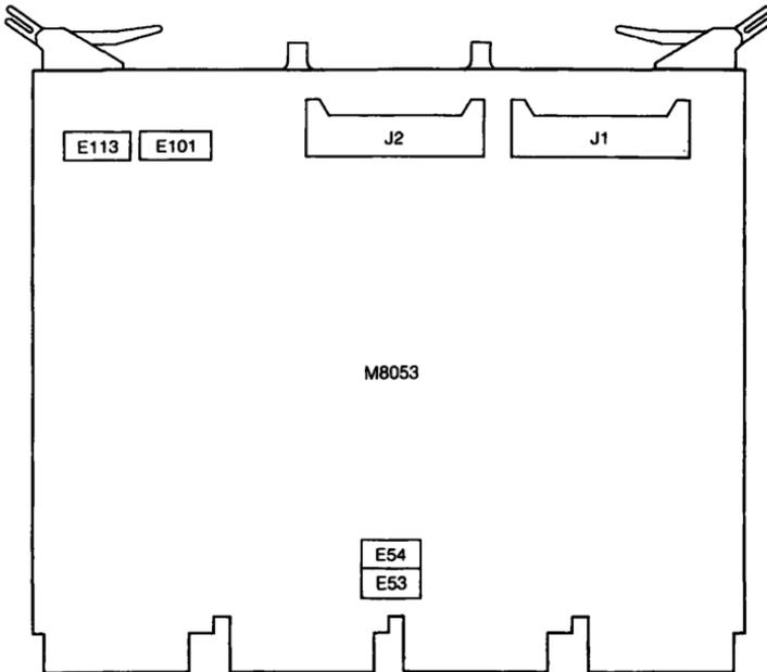
Figure 29-1 ■ DMV11 Switch Locations (M8053 Module)
