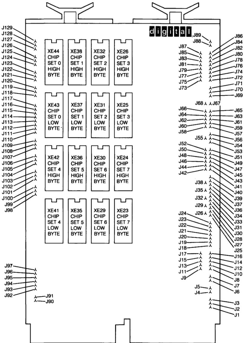
Figure 10-1 ■ MRV11-C Wirewrap Pin Locations
