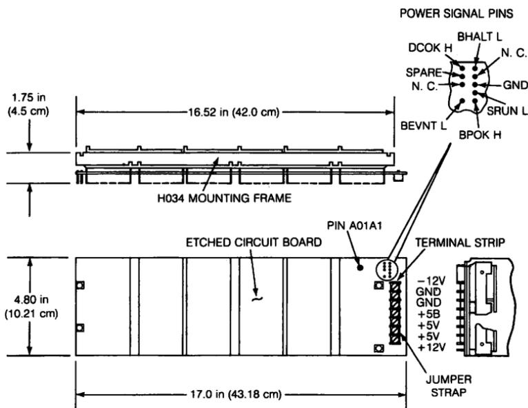
Figure 57-3 ■ DDV11-B Power Wiring
