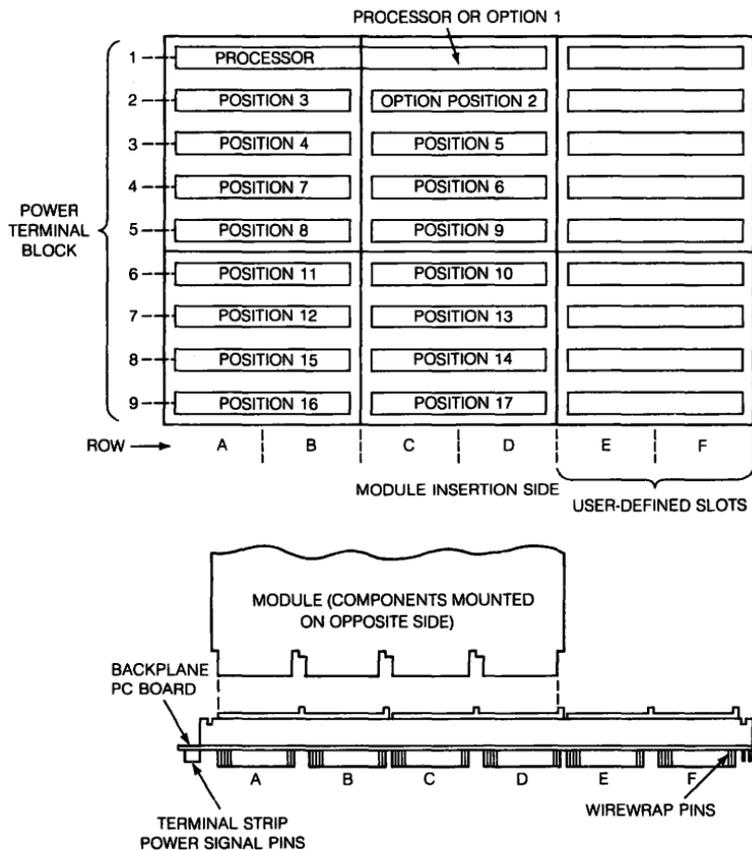
Figure 57-2 ■ DDV11-B Module Installation and Slot Assignments
