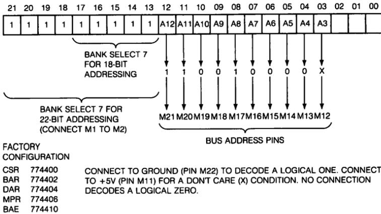
Figure 45-2 ■ RLV12 Device Address Format
