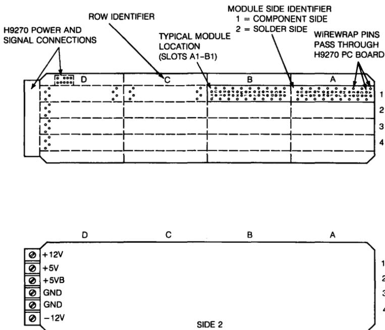
Figure 59-1 ■ H9270-Q Backplane Terminal Block (Pin Side View Shown)
