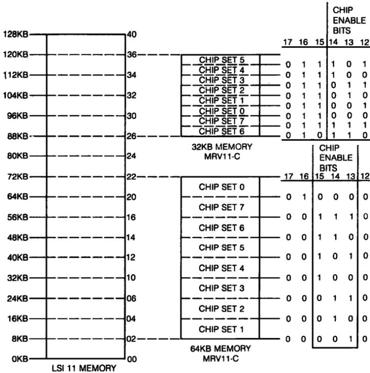
Figure 10-2 ■ Typical MRV11-C Memory Mapping
