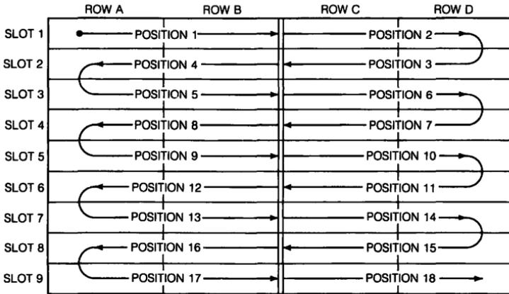
Figure 61-4 ■ Horizontal Position Priority Structure
