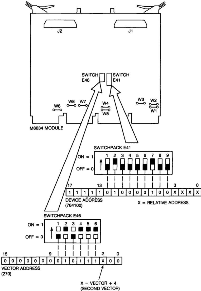
Figure 42-1 ■ M8634 Module Layout
