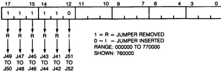
Figure 10-4 ■ MRV11-C Window Starting Address Selection
