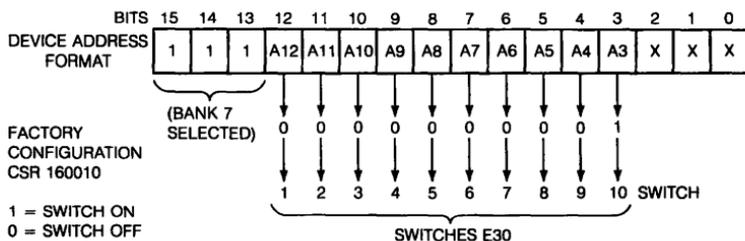
*Figure 25-2 ■ DZV11 Device Address Selection*
