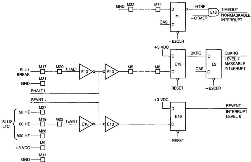
Figure 6-2 ■ SBC-11/21-PLUS Interrupt Configurations
