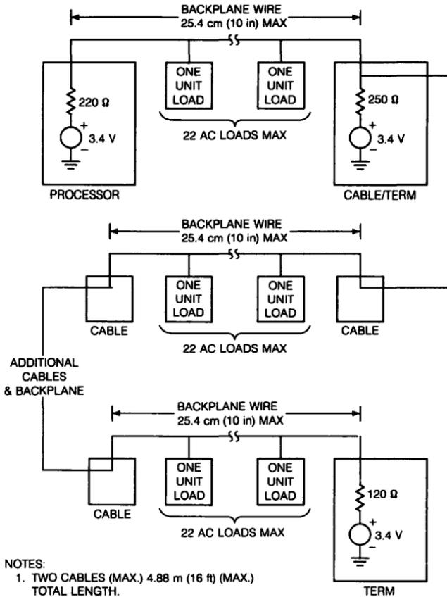
Figure 52-2 ■ Multiple Backplane Configuration
