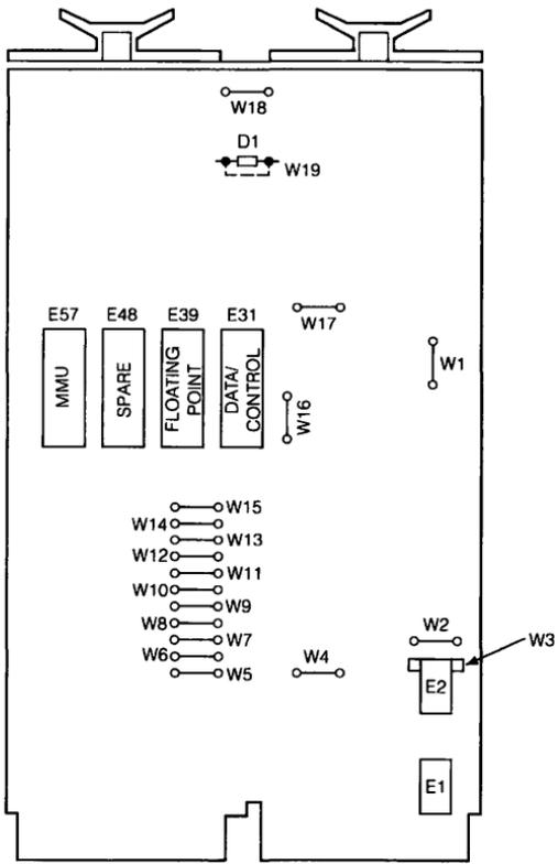
Figure 3-1 ■ LSI-11/23 Jumper Locations (Rev. A)
