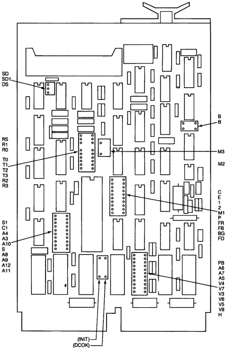
Figure 22-1 ■ DLVE1 Revision D Etch Jumper Locations
