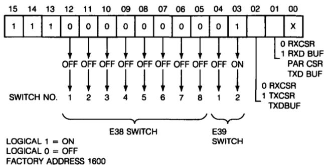
*Figure 31-2 ■ Device Address Selection*
