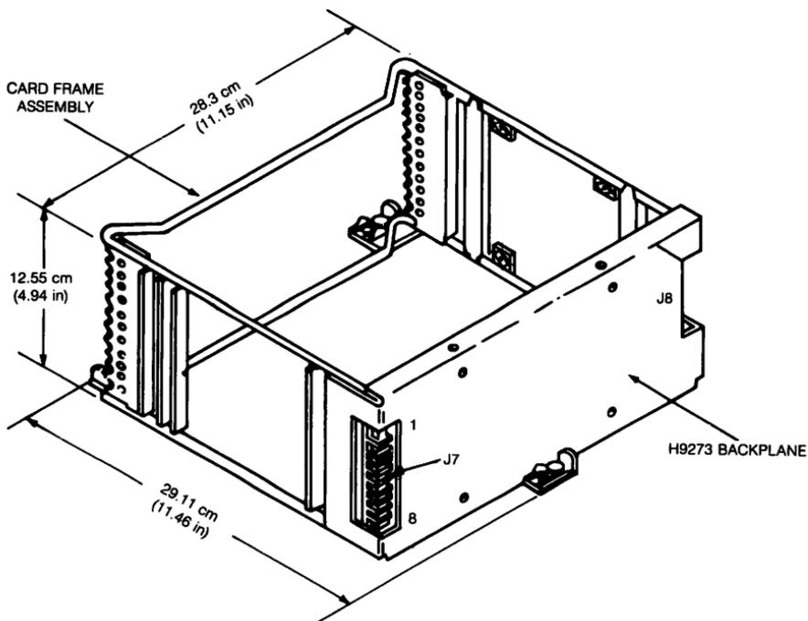
Figure 60-1 ■ H9273-A Backplane Logic Assembly
