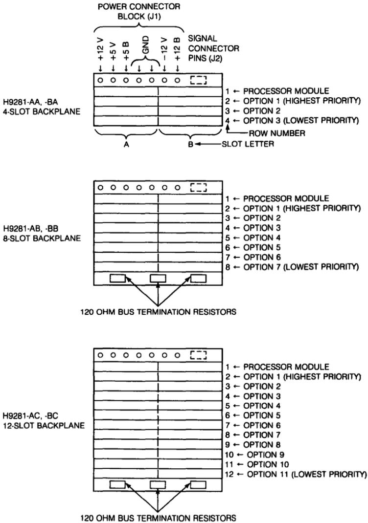
Figure 62-4 ■ H9281-Q Option and Connector Locations (Module Side)
