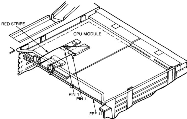
Figure 3-4 ■ FPF11 Cable Layout in LSI-11/23 System
