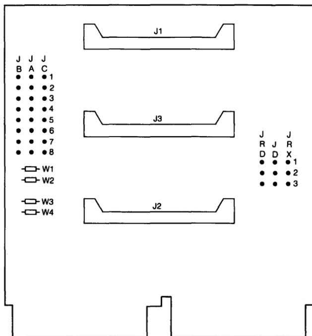
Figure 47-4 ■ RQDX1-E Extender Module Jumper Locations
