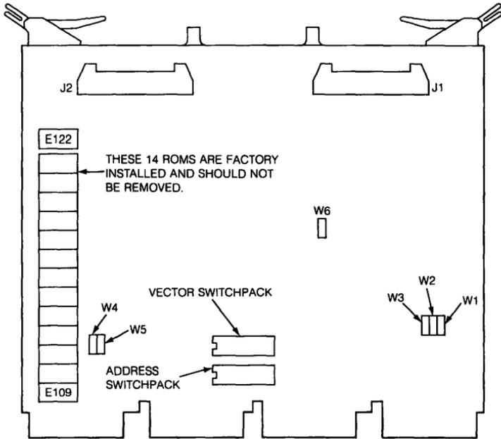
Figure 50-1 ■ TSV05 Interface Module Switch and Jumper Locations
