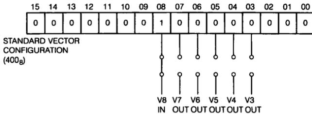
Figure 35-3 ■ Selecting AXV11-C Interrupt Vector Address
