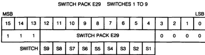
Figure 26-2 ■ KMV11-A Device Address Selection
