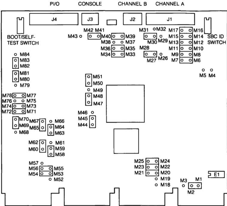
Figure 7-1 ■ KXT11-CA Jumper Layout
