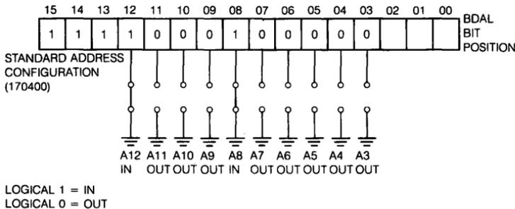
*Figure 35-2 ■ Selecting AXV11-C Device Address*
