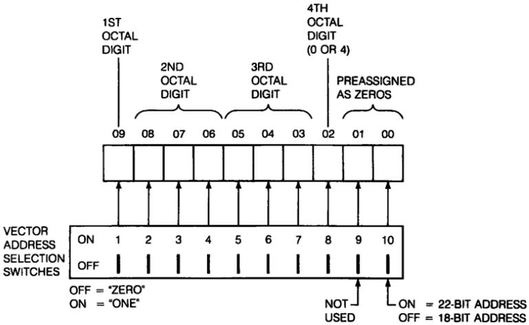
Figure 40-3 ■ DRV11-WA Interrupt Vector Address Selection
