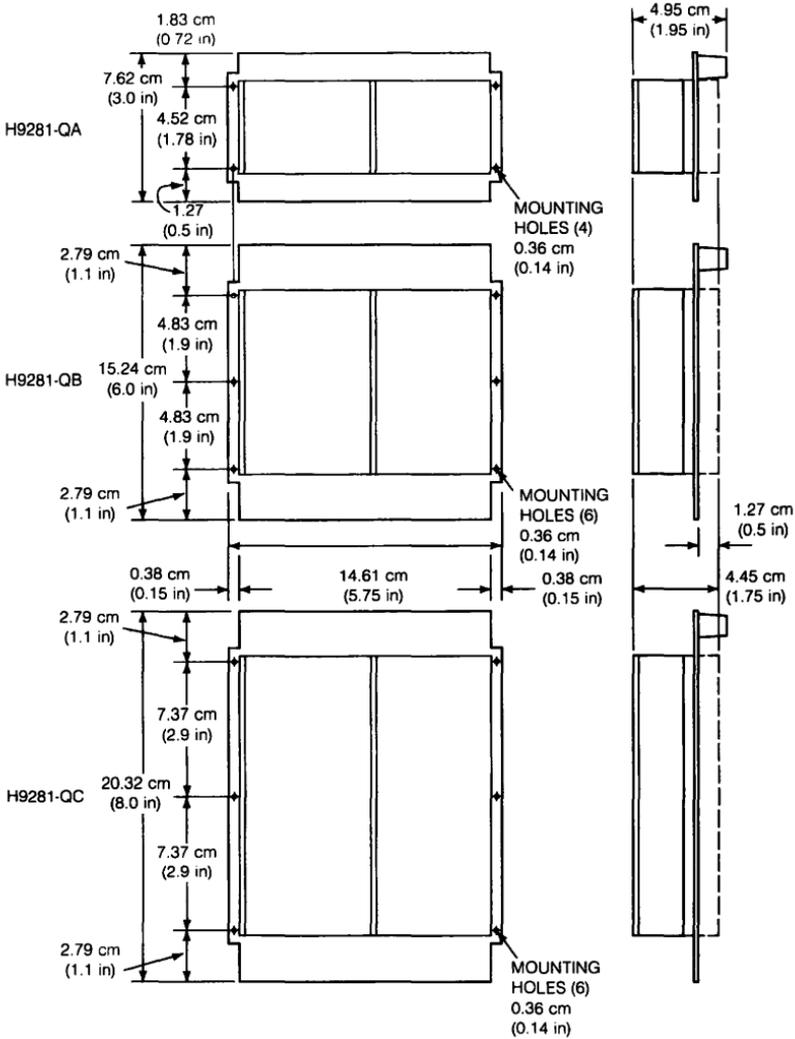
Figure 62-1 ■ H9281-Q Mounting Dimensions
