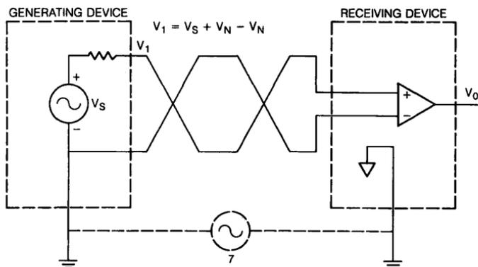
Figure 34-6 ■ Differential Inputs
