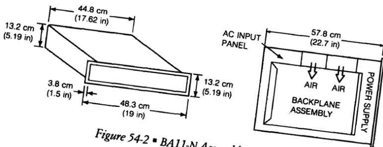
Figure 54-2 ■ BA11-N Assembly Unit
