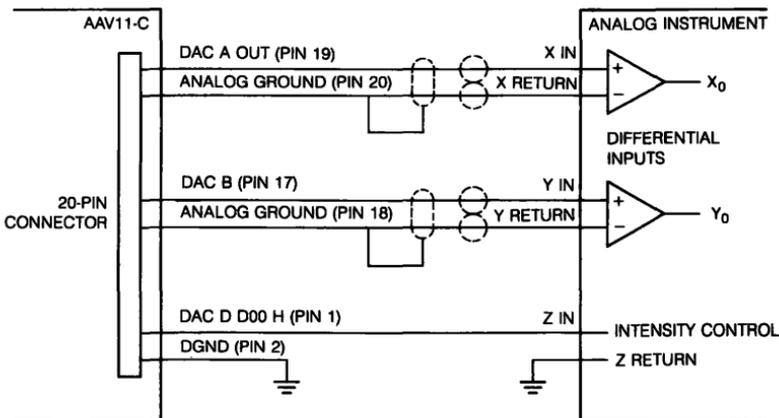
Figure 33-3 ▪ Connecting AAV11-C to a Differential Input Device
