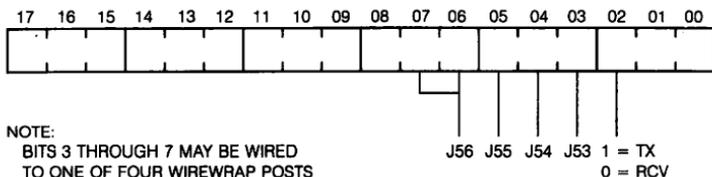
Figure 17-5 ■ MXV11-A Interrupt Vector Format
