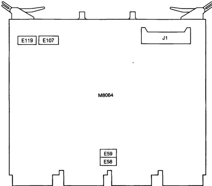
Figure 29-2 ■ DMV11 Switch Locations (M8064 Module)
