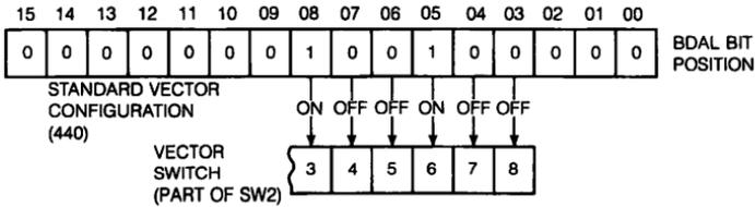
Figure 36-3 ■ Selecting K WV11-C Interrupt Vector Address
