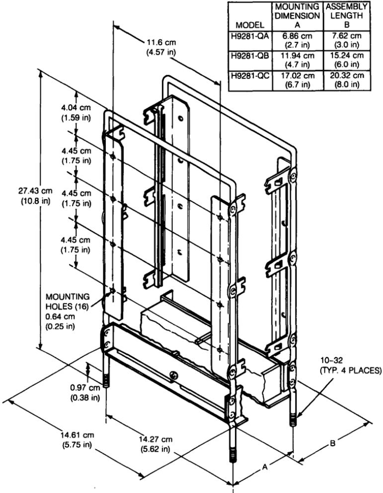
Figure 62-2 ■ H9281-Q Mounting Dimensions
