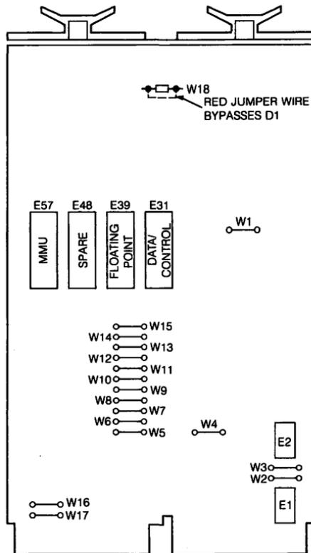
Figure 3-2 ■ LSI-11/23 Jumper Locations (Rev. C)
