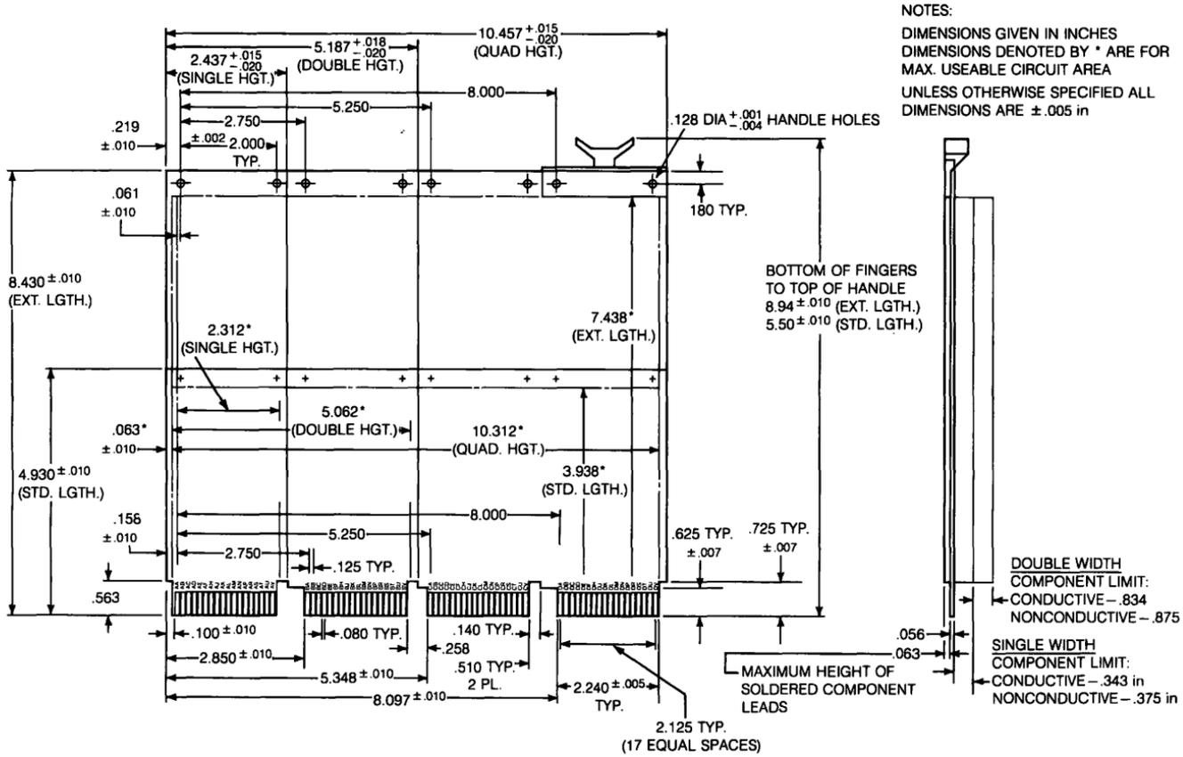
Figure 1-2 ■ Q-bus Module Dimensions
