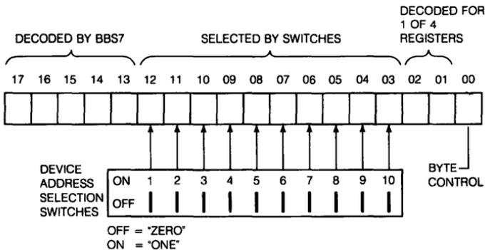
*Figure 40-2 ■ DRV11-WA Device Address Selection*
