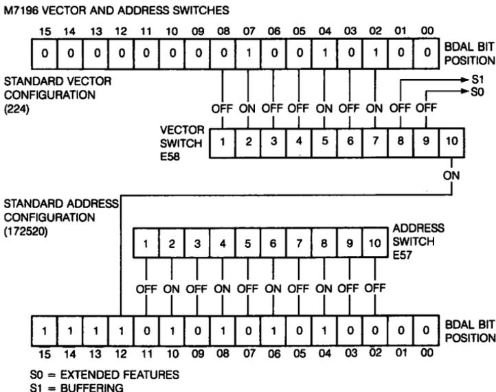
Figure 50-2 ■ TSV05 Vector and Device Address Selection
