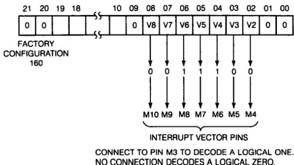
Figure 45-3 ■ RLV12 Interrupt Vector Format
