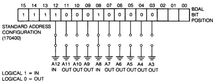
**Figure 34-2 ■ Selecting ADV11-C Device Address**
