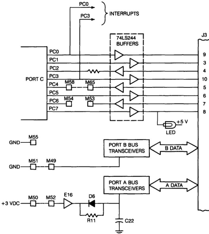
Figure 6-3 • SBC-11/21-PLUS Parallel I/O Configurations
