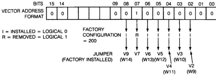
Figure 44-3 ■ LPV11 Interrupt Vector Selection Jumpers
