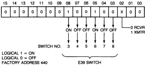
Figure 31-3 ■ DUV11 Interrupt Vector Selection
