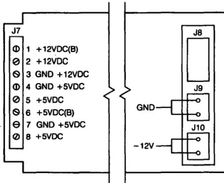
Figure 60-2 ■ H9273-A Power Connections
