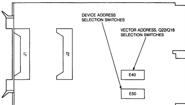
Figure 40-1 ■ DRV11-WA Connector and Switch Locations
