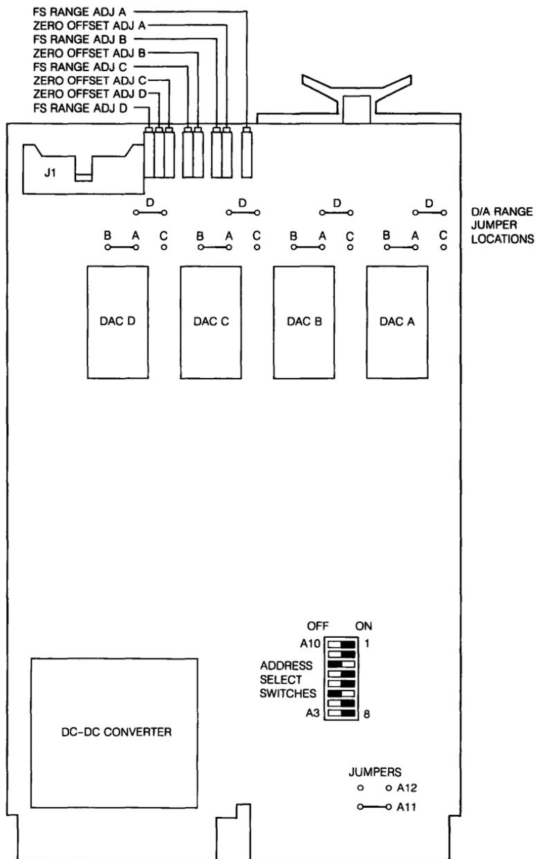
Figure 33-1 ■ AAV11-C Physical Layout
