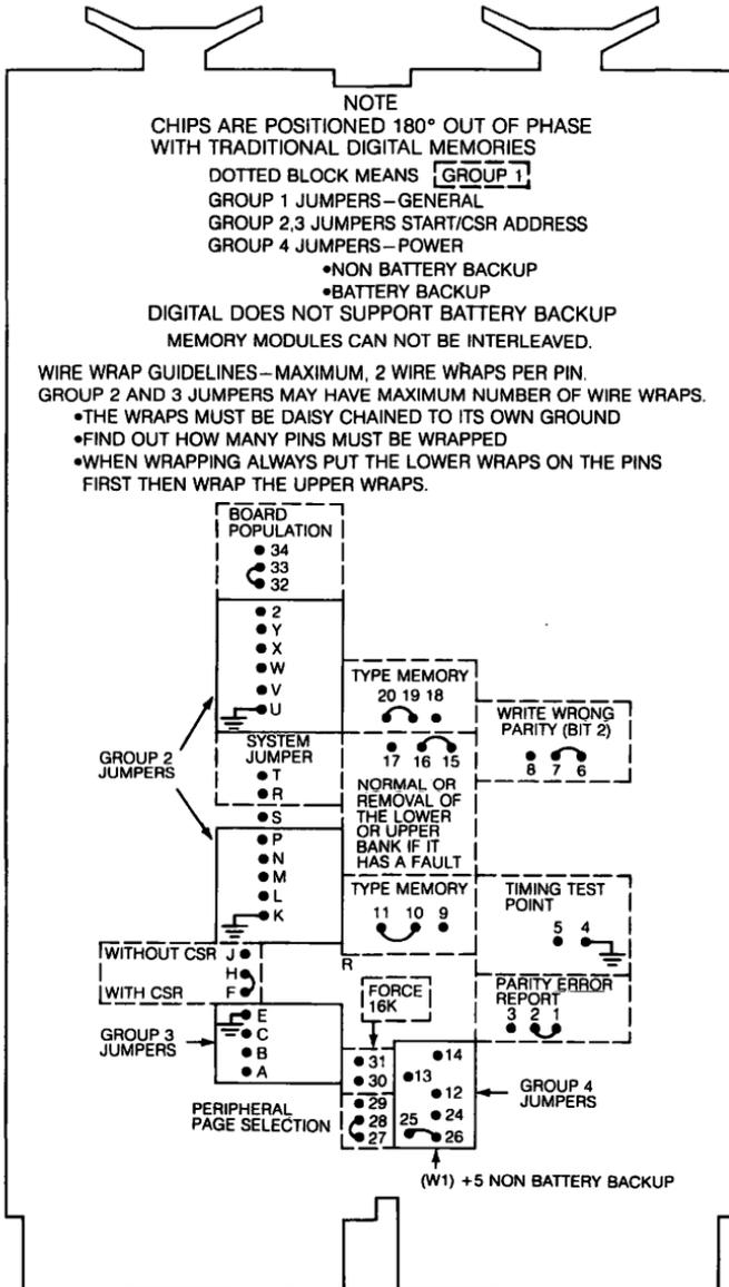
Figure 13-1 ■ MSV11-L Memory Module Jumpers
