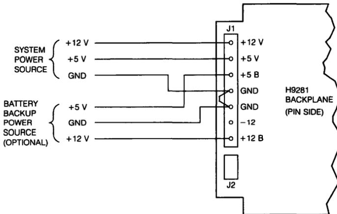
Figure 62-3 ■ H9281 Power Connections
