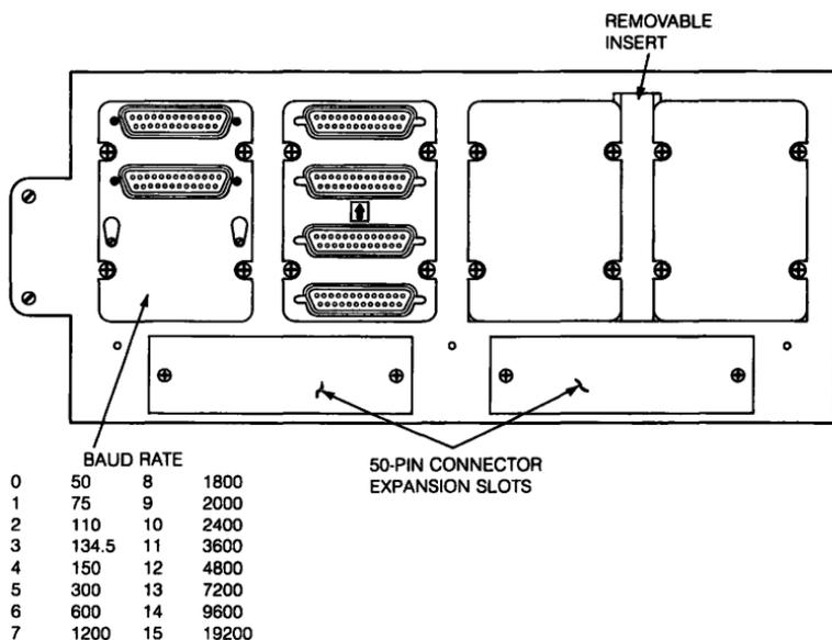
Figure 56-5 ■ Patch and Filter Panel Assembly
