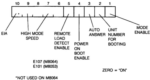
Figure 29-5 ■ DMV11 Switch-selectable Features
