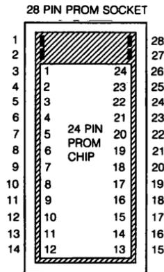
Figure 18-3 ■ Insertion of 24-Pin PROM Chips
