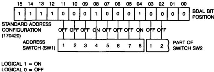
*Figure 36-2 ■ Selecting KVV11-C Device Address*
