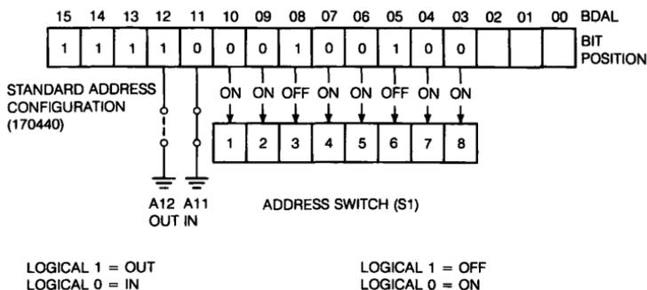
Figure 33-2 ■ Selecting AAV11-C Device Address
