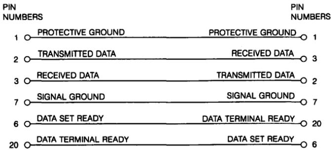
*Figure 20-5 ■ Null Modem Cable Connections*
