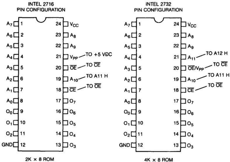
Figure 10-5 ■  $2K \times 8$  and  $4K \times 8$  Pin Configurations
