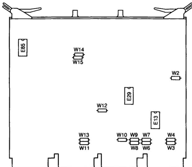
Figure 26-1 ■ KMV11-A Jumper and Switch Locations
