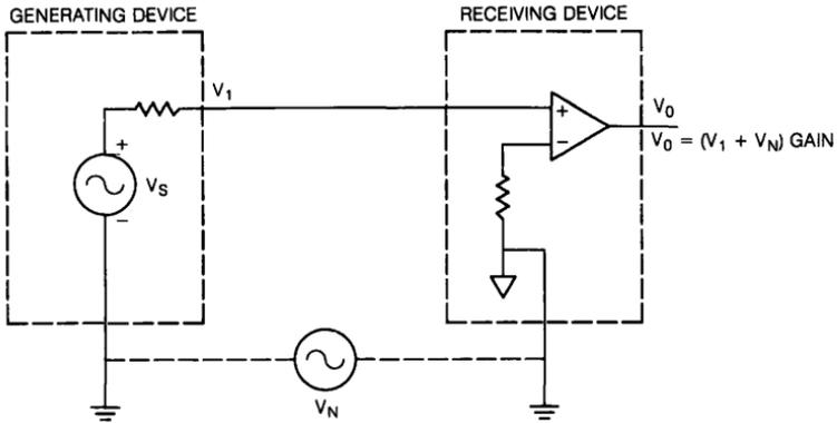
Figure 34-4 ■ Single-Ended Analog Input
