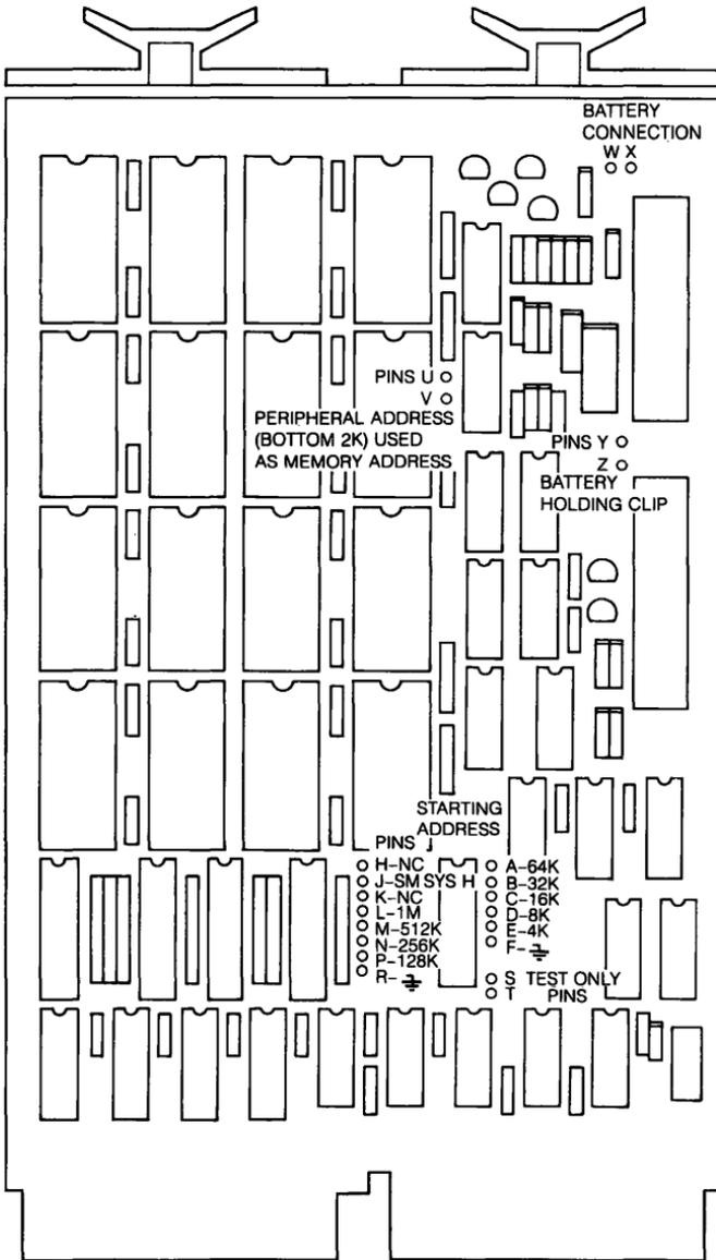
Figure 9-1 ■ MCV11-D Module Layout
