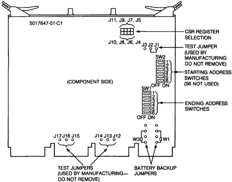
Figure 15-2 ■ MSV11-Q Switches and Jumpers
