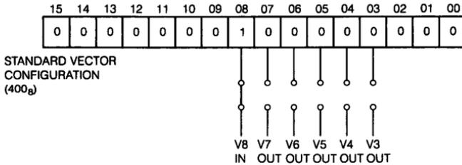
Figure 34-3 ■ Selecting ADV11-C Interrupt Vector Address
