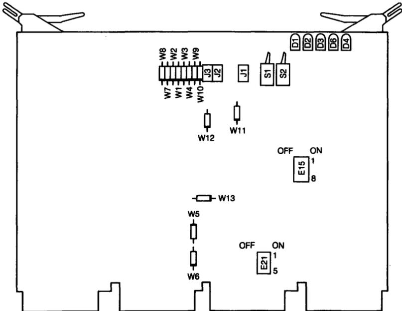
Figure C-1 ■ BDV11 Switch and Jumper Locations
