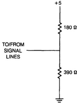
Figure 63-2 ■ Typical 120-Ohm Bus Termination
