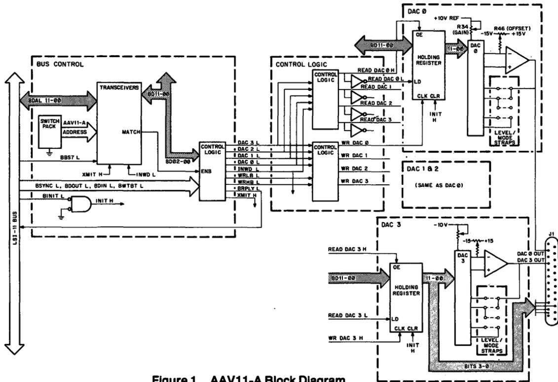
Figure 1 AAV11-A Block Diagram
