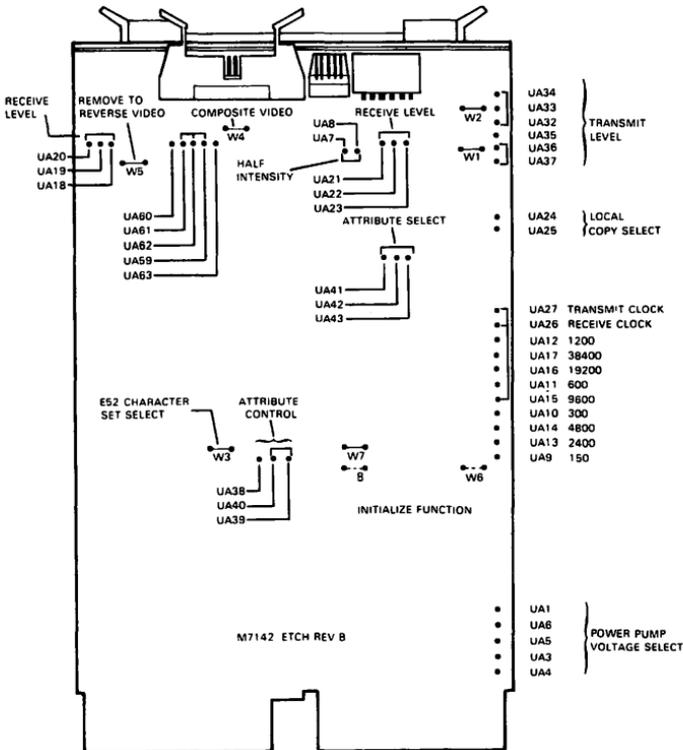
Figure 6 Jumper and Wire Wrap Post Locations
