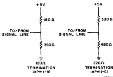
Figure 5 KPV11-B and KPV11-C Bus Terminations
