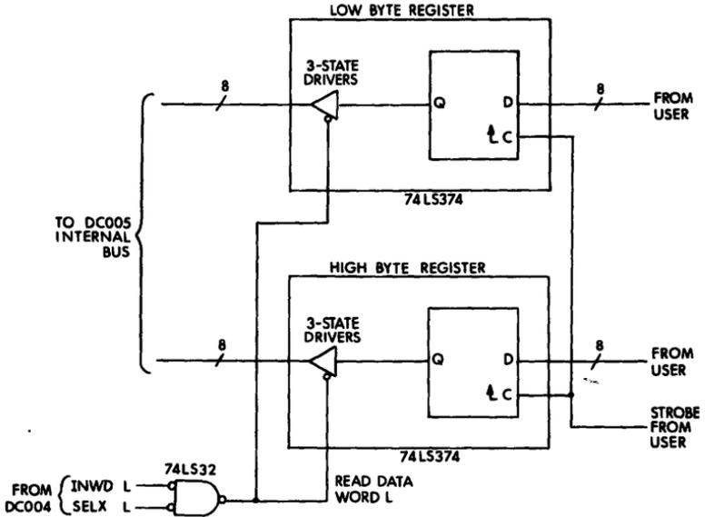
Figure 8 Example of Input Register (WORD)
