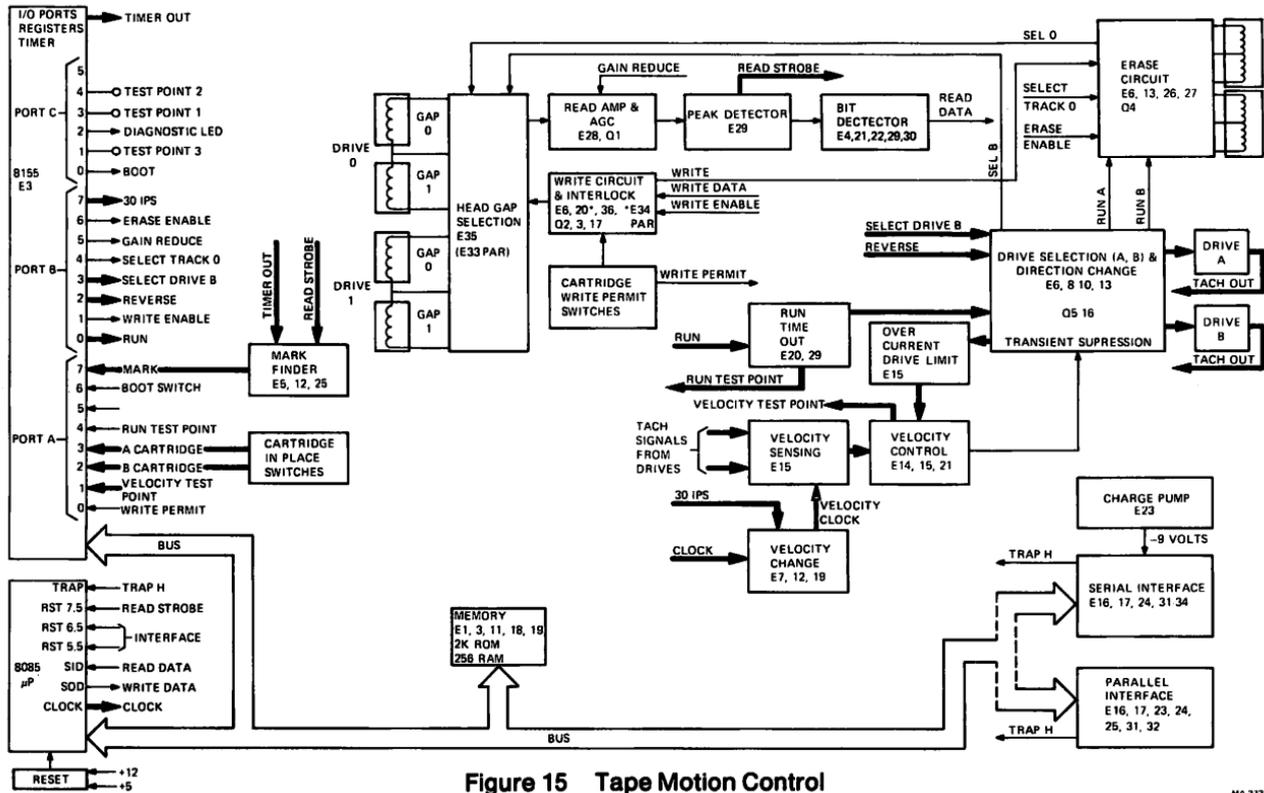
Figure 15 Tape Motion Control
