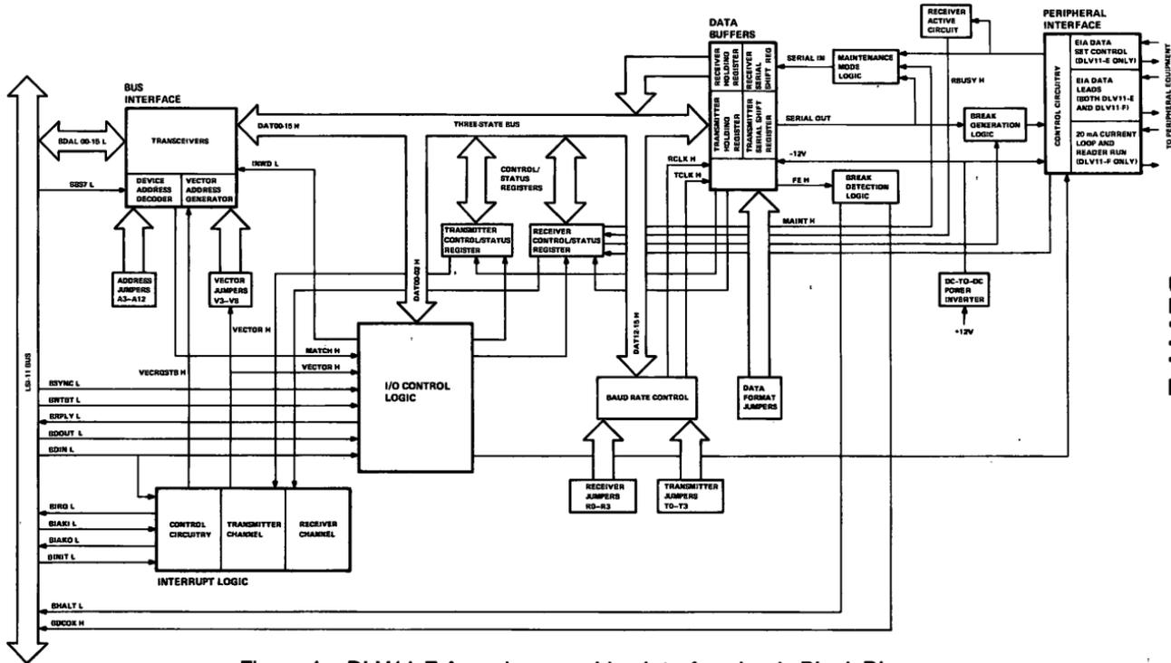
Figure 1 DLV11-E Asynchronous Line Interface Logic Block Diagram
