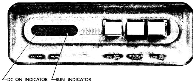
Figure 12 Console Panel Controls and Indicators
