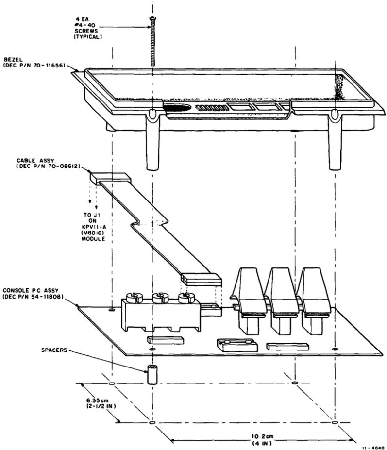
Figure 11 Console Panel Installation
