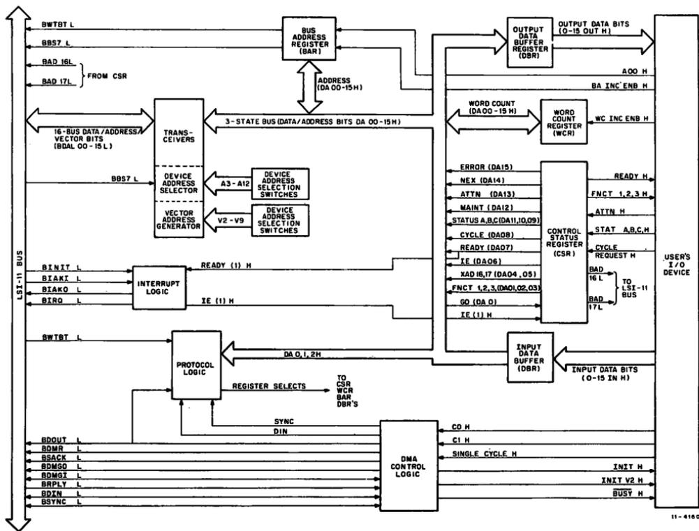
Figure 1 DRV11-B Logic Block Diagram
