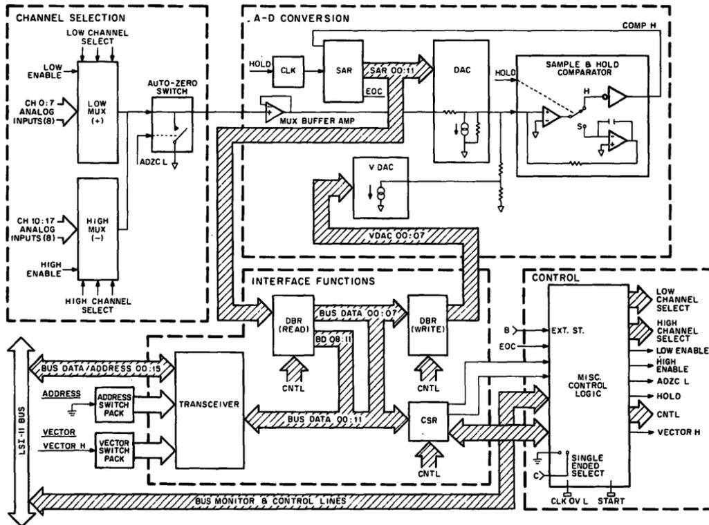
Figure 1 ADV11-A Functional Block Diagram
