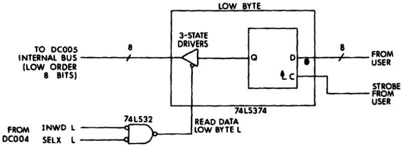
Figure 7. Example of Input Register (BYTE)
