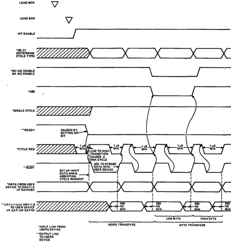
**Figure 4 DRV11-B Timing: Single Cycle, Asynchronous, User-Initiated**
