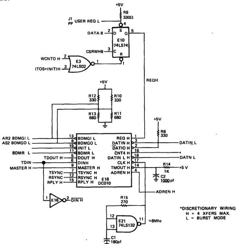
Figure 4 Typical Application (DC006, DC010, Output Delay, and Input Drives)
