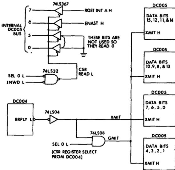
WHEN THE CSR IS READ (SEL 0 L = 0) THE SIGNAL GMIT WILL BE 0 CAUSING THE UNUSED DC005 BITS TO BE READ AS ZEROS. (HIGH ON BDAL LINES) FOR ANY OTHER REGISTER GMIT = XMIT.
