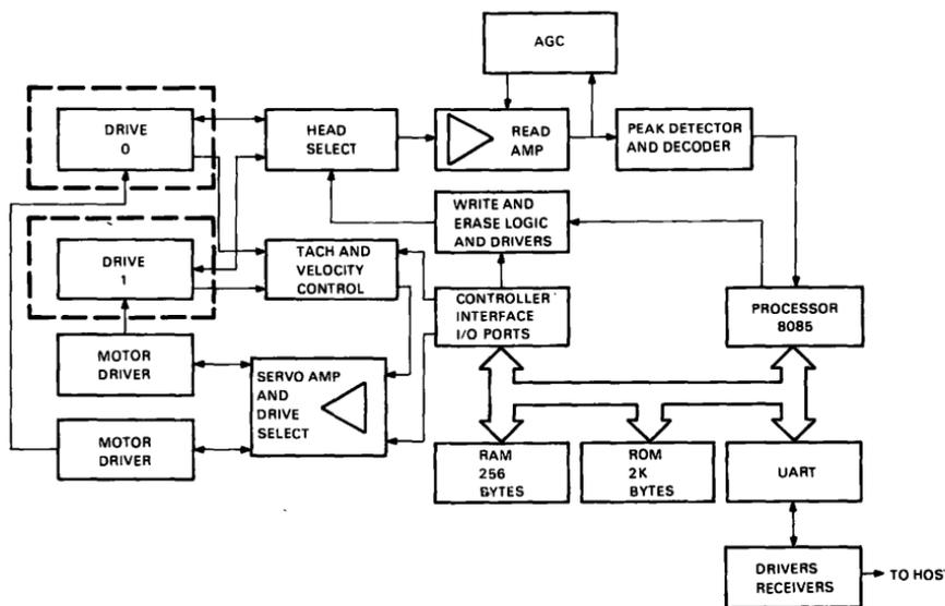
Figure 3 TU58 Block Diagram
