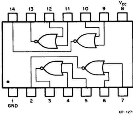
**Figure 3 8640 Quad 2-Input NOR Gates (Bus Receiver)**
