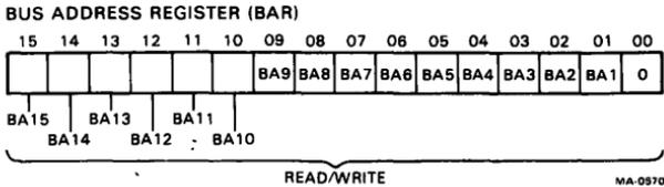
Figure 7 Bus Address Register
