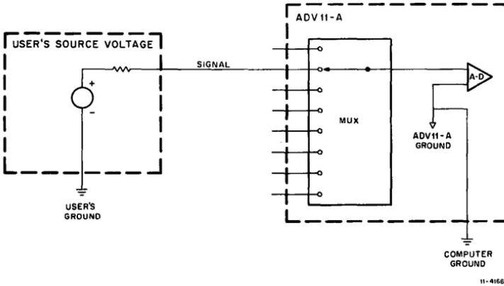
Figure 7 Single-Ended Input Referenced to User's Ground
