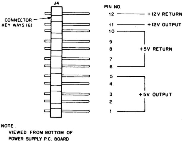
Figure 21 Pinning for H780 DC Output Connector (J4)
