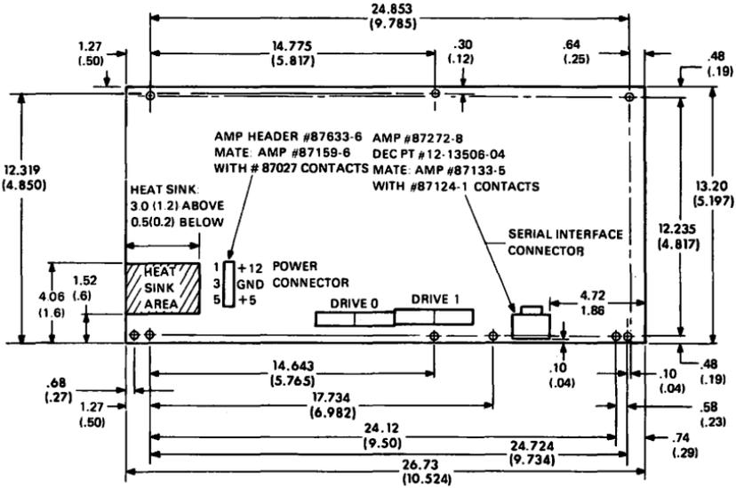
MEASUREMENTS ARE IN CENTIMETERS EXCEPT VALUES IN PARENTHESES ARE IN INCHES MEASUREMENTS ARE  $\pm .013$  (.005) CENTER TO CENTER
