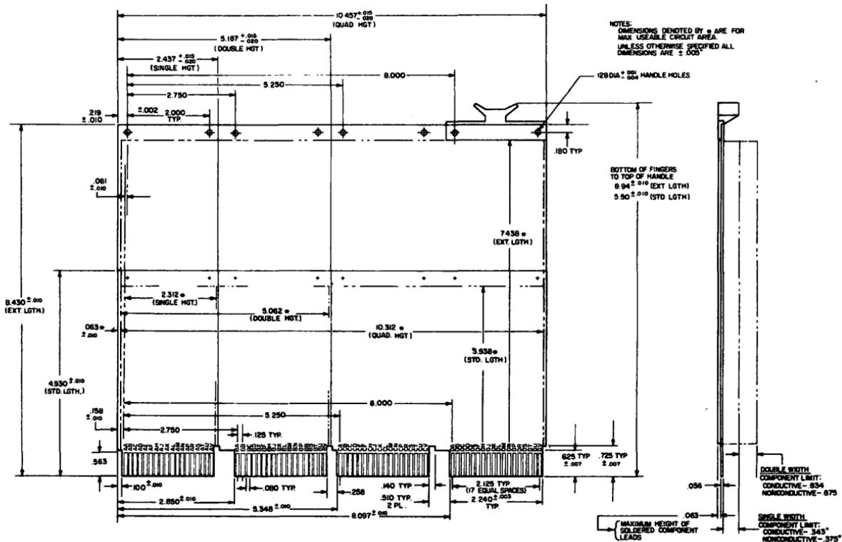
Figure 1 Module Dimensions
