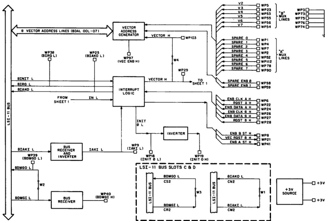
Figure 1 DRV11-P Block Diagram (Sheet 2 of 2)
