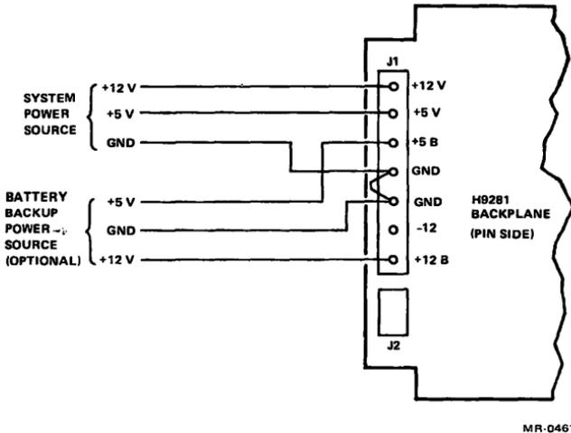
Figure 3 H9281 Power Connections
