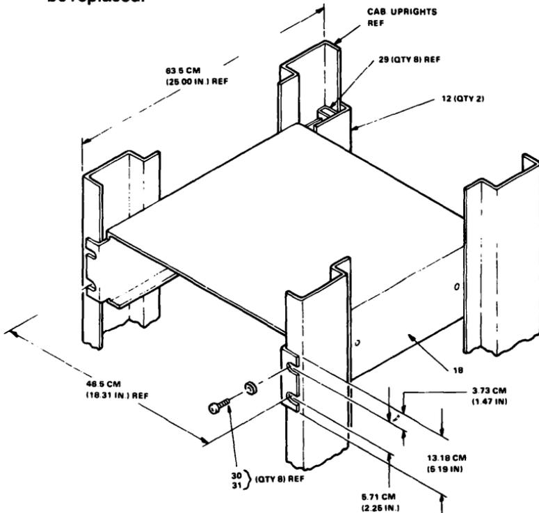
Figure 3 BA11-NE and BA11-NF Cover Mounting Dimensions
