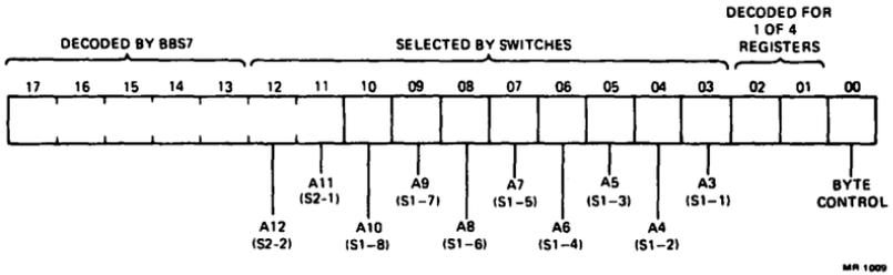
**Figure 2 Device Address Select Format**
