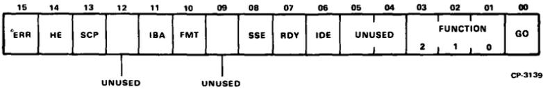
Figure 9 Control/Status Register (RKCS)—Address 177404
