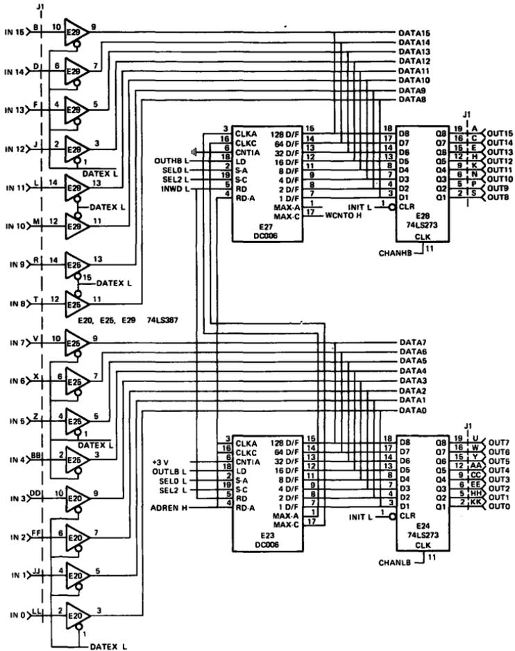
Figure 4 Typical Application (DC006, DC010, Output Delay, and Input Drives)
