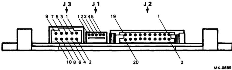
Figure 4 Connector Pin Number Location Diagram
