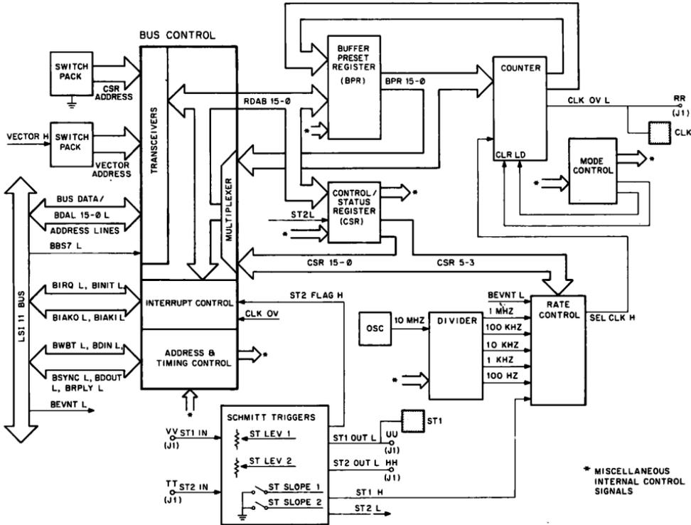
Figure 1 KWV11-A Real-Time Clock Block Diagram
