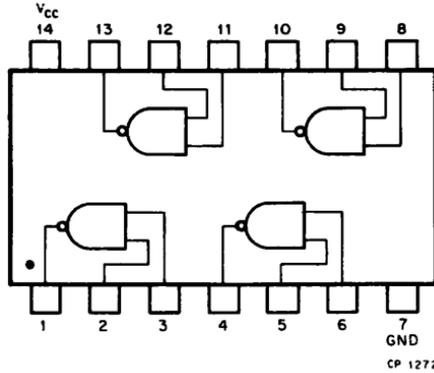
**Figure 4 8881 Quad 2-Input NAND Gate (Bus Driver)**
