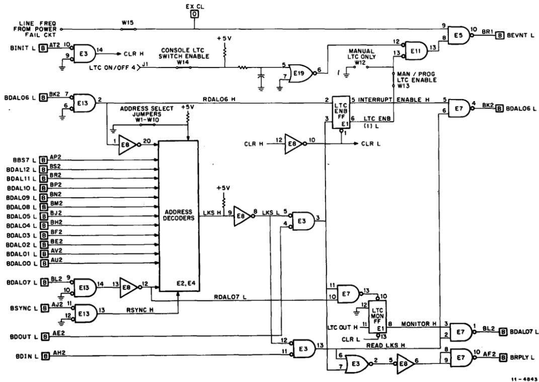
Figure 4 Programmable Line-Time Clock Circuits
