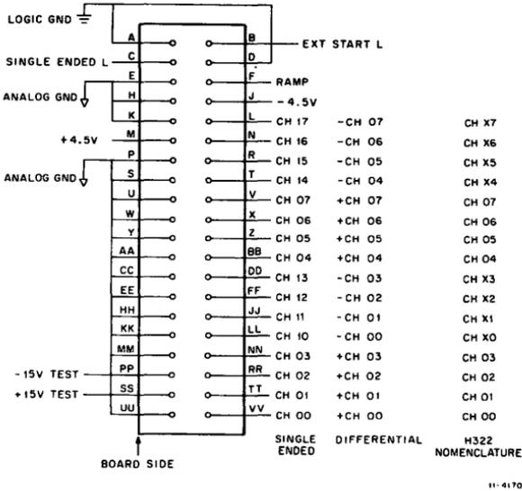
Figure 11 ADV11-A 40-Pin Connector Pin Assignments
