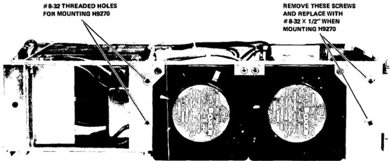
Figure 17 Left Side of H780 Showing H9270 Mounting Holes
