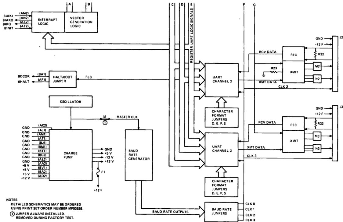
Figure 1 DLV11-J Block Diagram (Sheet 2 of 2)
