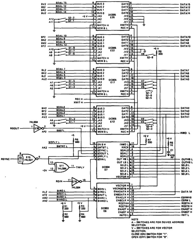
Figure 1 Typical DMA CHIPKIT Application
