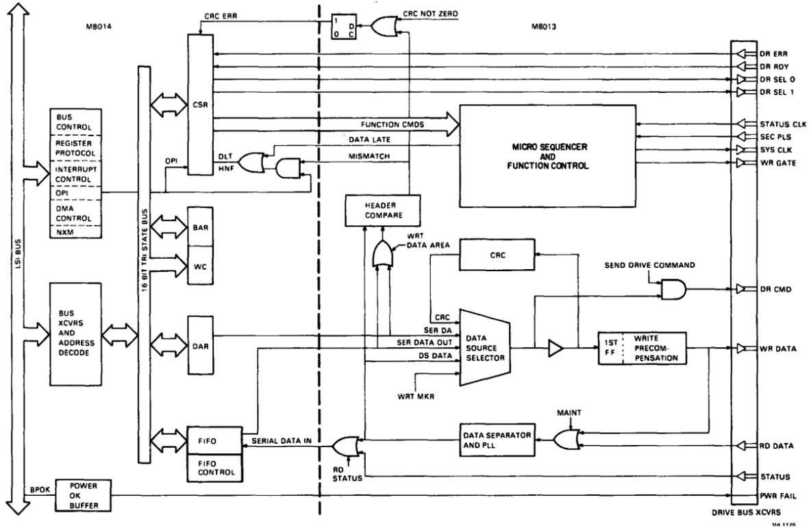
Figure 1 RLV11 Controller Simplified Block Diagram
