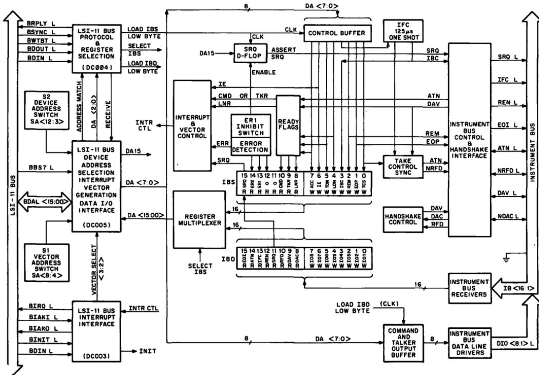
Figure 1 IBV11-A Functional Block Diagram
