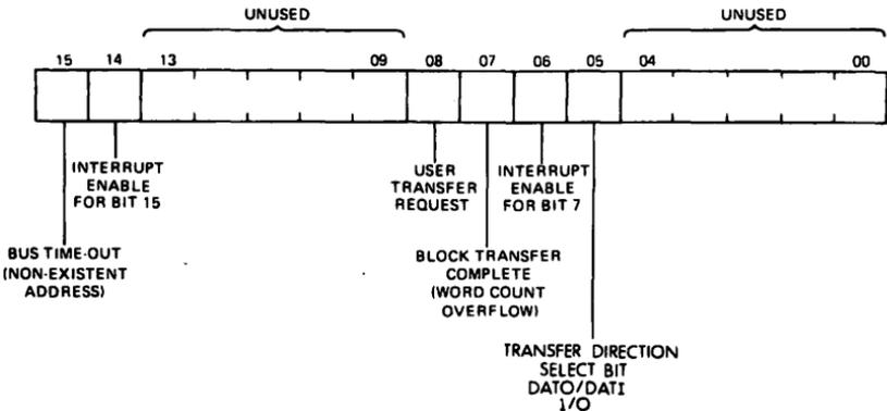
Figure 6 Control/Status Register (CSR) Format
