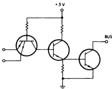
Figure 2 Typical Bus Driver Circuit
