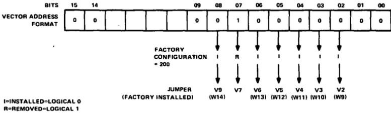
Figure 6 LPV11 Interrupt Vector Format and Jumpers
