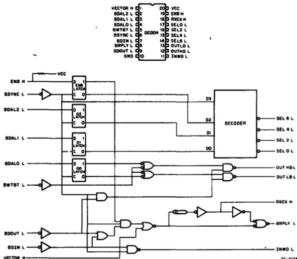
Figure 3 DC004 Simplified Logic Diagram
