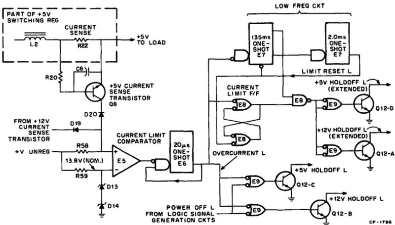
Figure 7 Overload and Short-Circuit Protection Circuits
