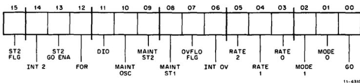
Figure 7. CSR Bit Assignments
