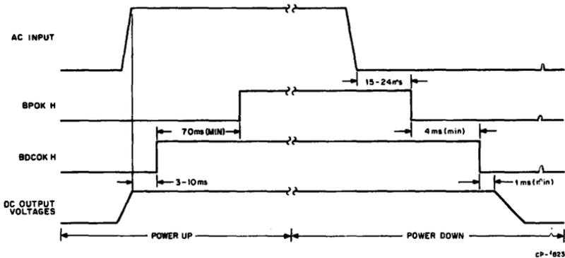
Figure 10 Power-Up/Power-Down Sequence
