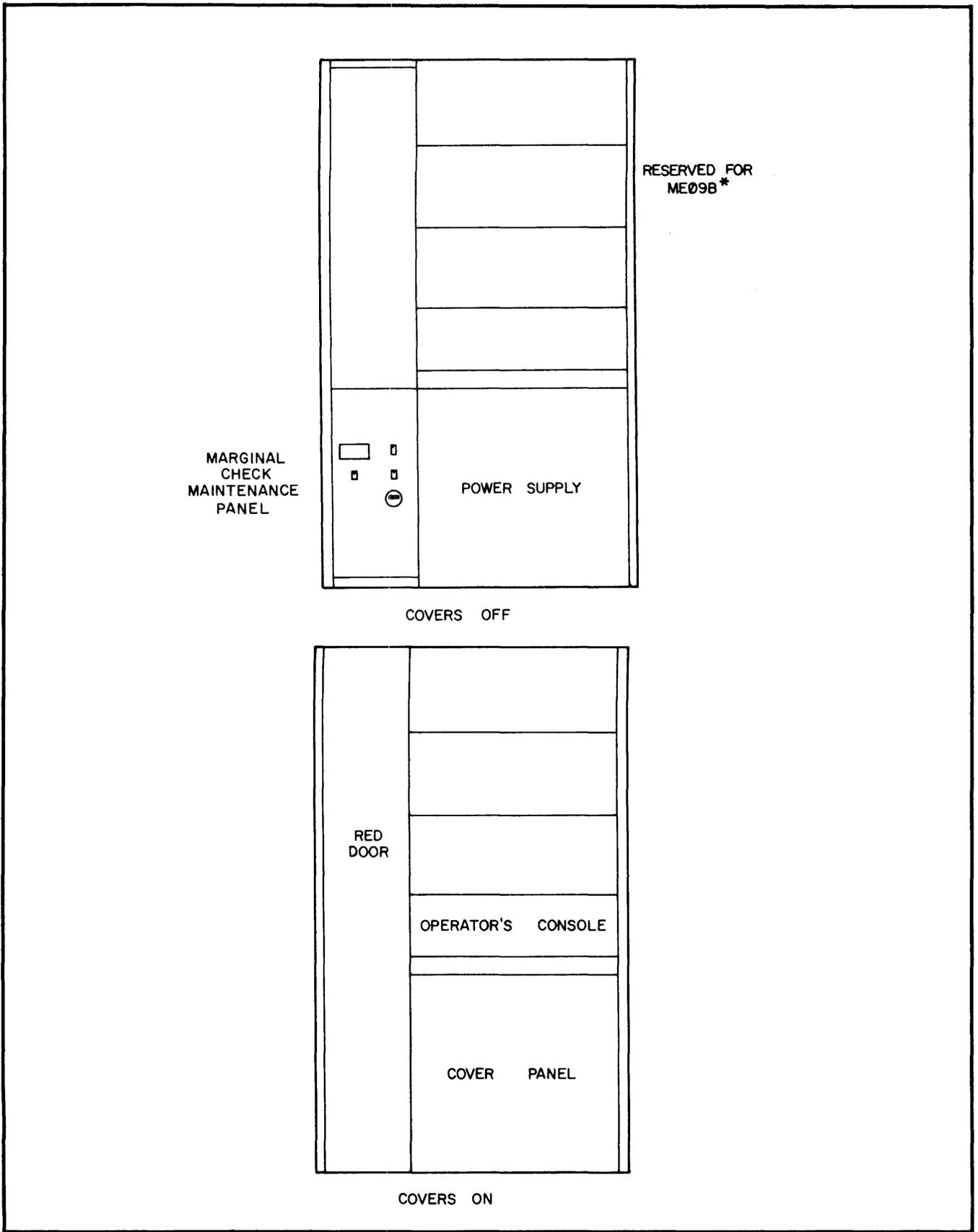
Figure 15-2(A). Basic PDP-9/L (Front)
