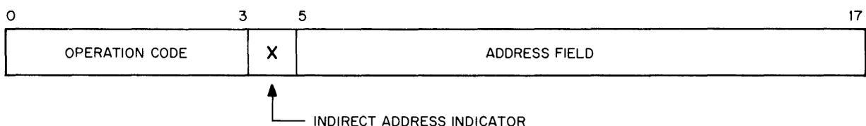
however, would not enter 000077 in the AC but the contents of location 00077 (considering the address field limitation of 15 bits for addressing up to 32,768 locations).
