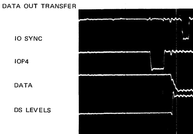
DATA IS READ INTO DEVICE BUFFER AT LEADING EDGE OF IOP4
