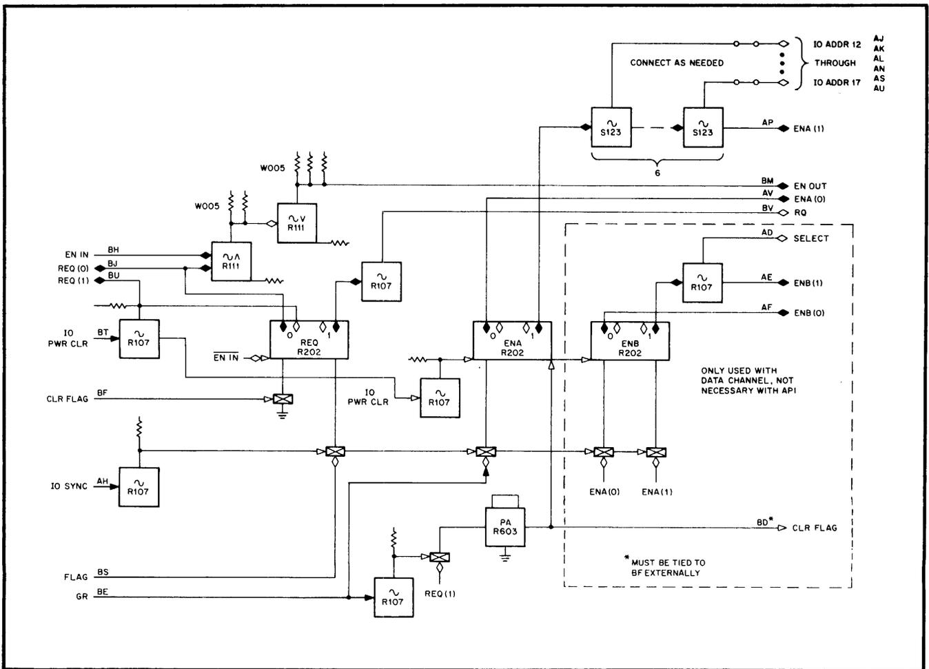
Figure 14-2 Type W104 Bus Multiplexer
