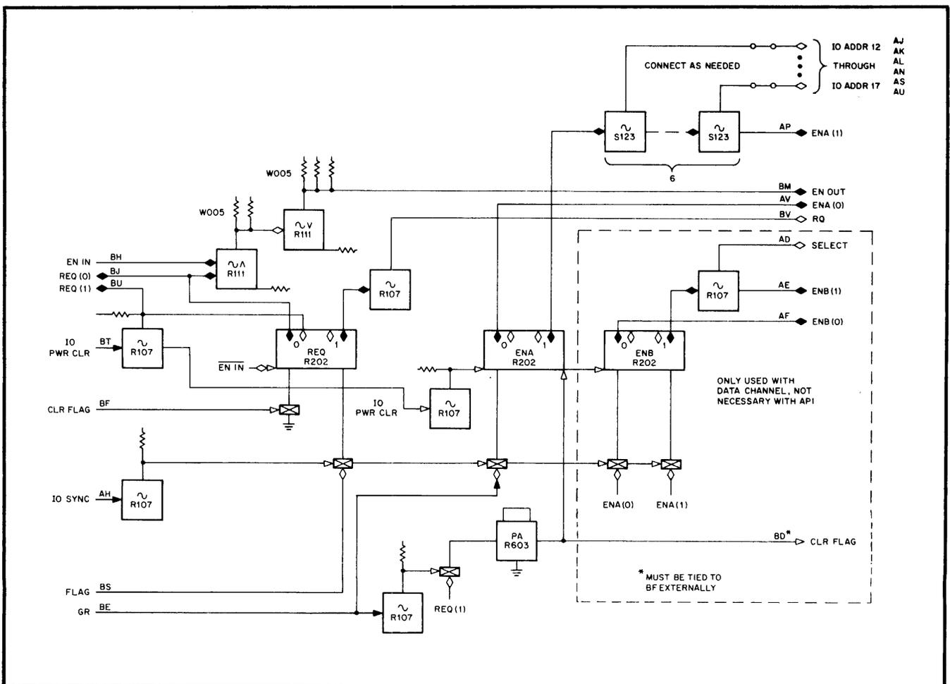
Figure 14-2 Type W104 Bus Multiplexer
