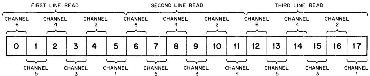
\*Note: In hardware readin mode, channel 7 must be punched in line 3 of last data word or read will not stop (refer to chapter 10 for description of READ IN key).
