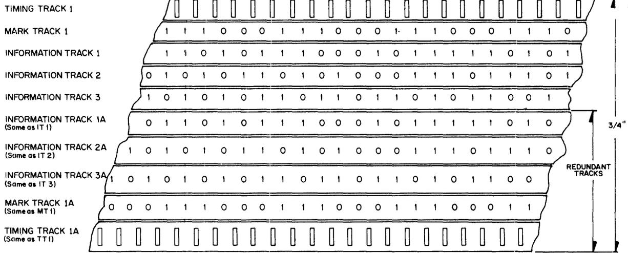
Track Allocation Showing Redundantly Paired Tracks
