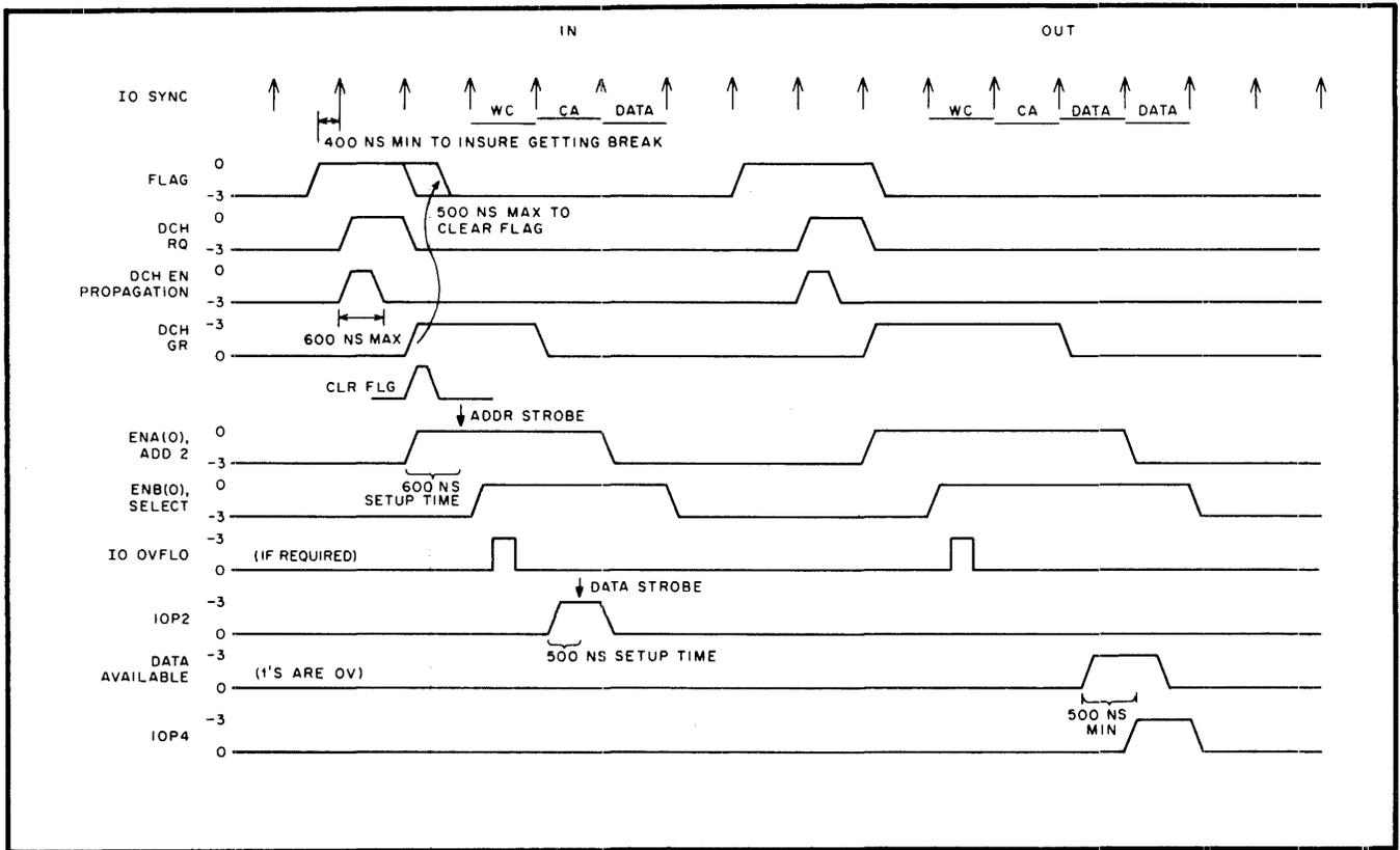
Figure 14-5 DCH Timing
