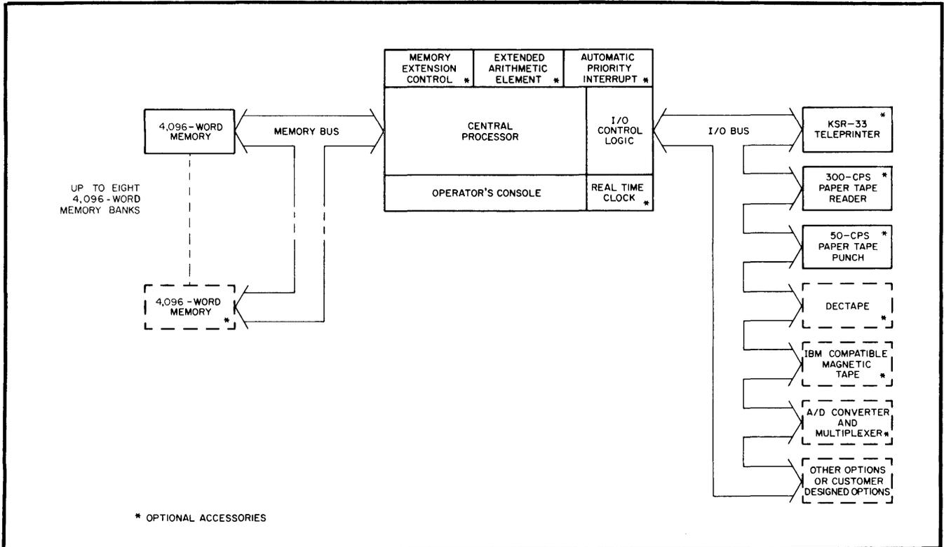
Figure 1-2. Expanded PDP-9/L System Configuration, Block Diagram
