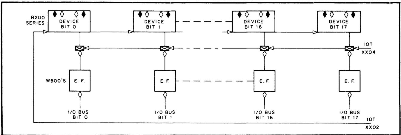
Figure 13-7 Loading a Device Buffer from AC
