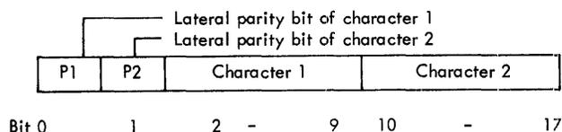
*Read/Compare* - A direct comparison of the characters on tape is made with those in memory. The parity bits are ignored, as are bits 0 and 1 of each memory word.
