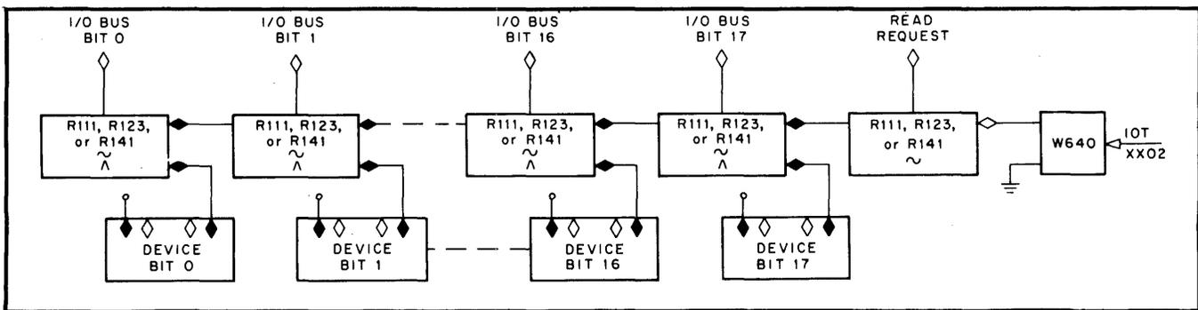
Figure 13-5 Loading the AC from a Device Buffer
