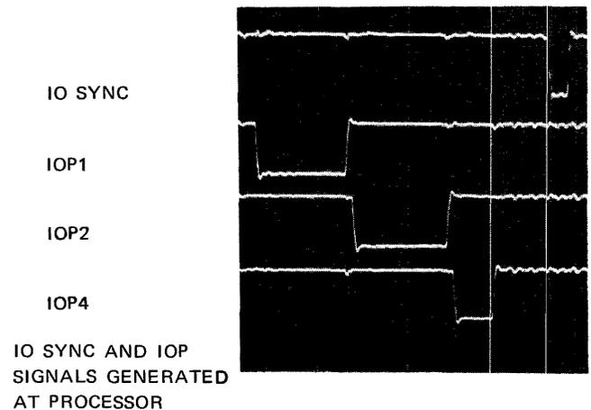
Figure 13-3 IOT Pulse Waveforms
