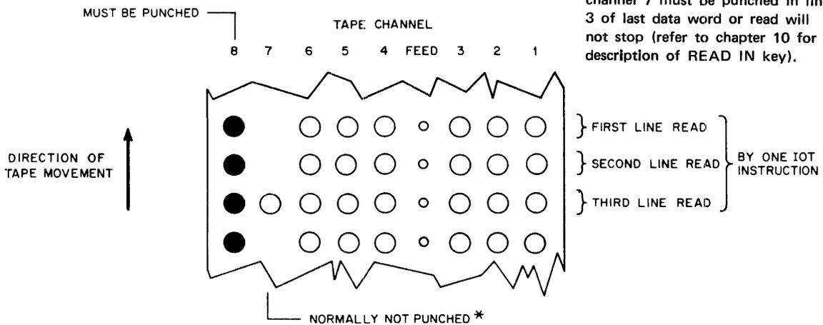
b. Tape Format and Reader Buffer Register Bit Assignments in Binary Mode
