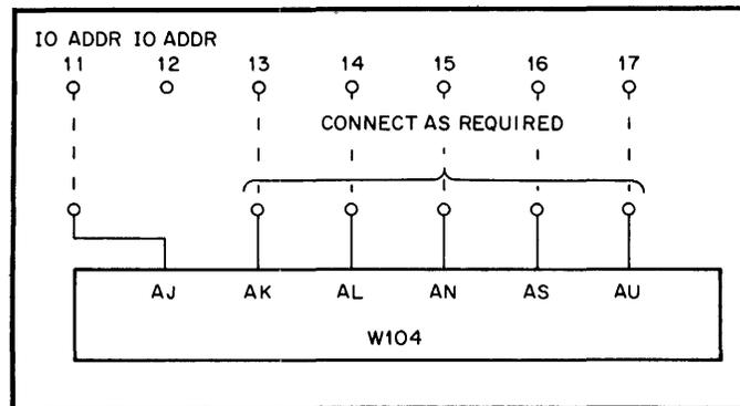
Figure 13-13 Connections for Trap Addresses Between  $100_8$  and  $137_8$
