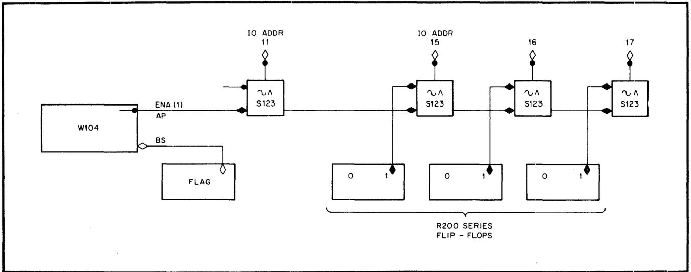
Figure 13-14 Gating Flip-Flop Register onto I/O Address Lines
