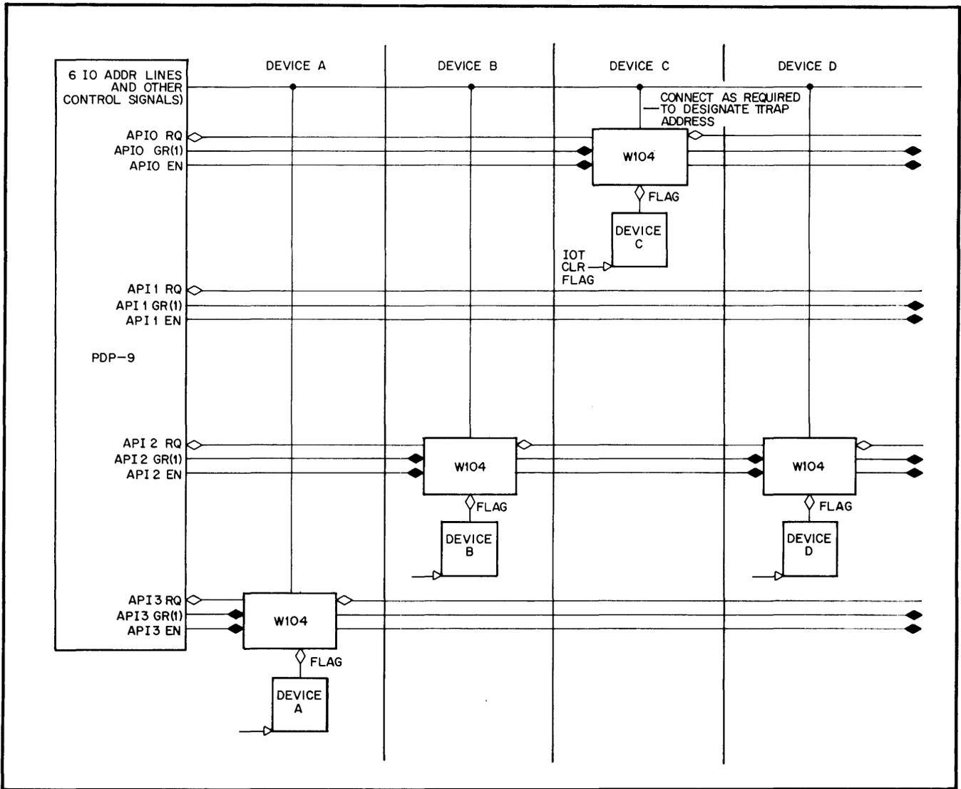
Figure 13-12 Devices on the Automatic Priority Interrupt
