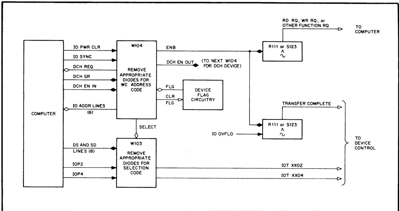
Figure 14-1 Data Channel Configuration
