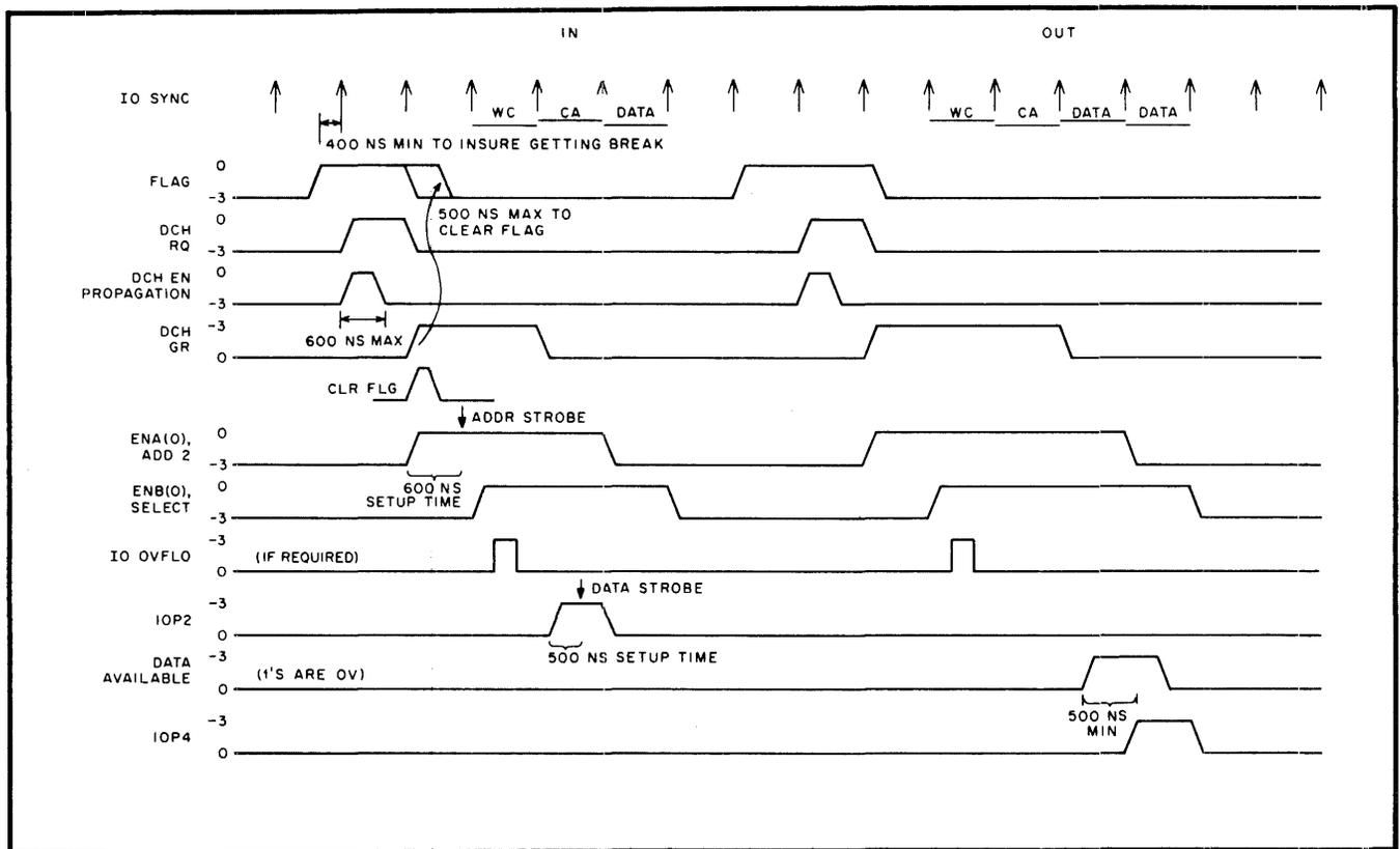
Figure 14-5 DCH Timing
