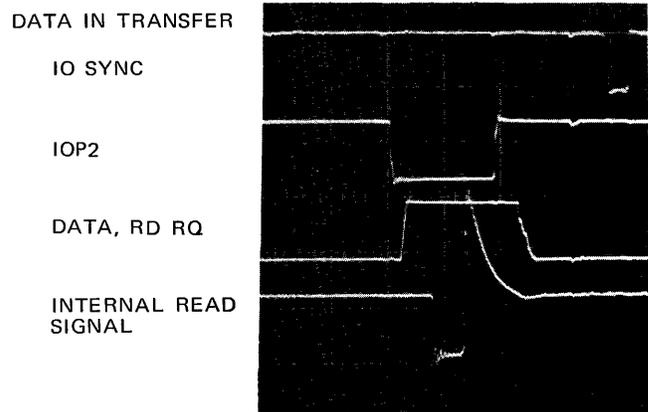
DATA IS READ INTO AC ON TRAILING EDGE OF INTERNAL READ SIGNAL
