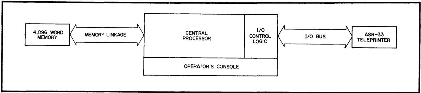
Figure 1-1. Basic PDP-9/L
