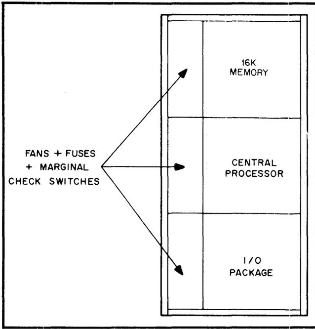
Figure 15-2 (B). Basic PDP-9/L (Rear, Back Door Removed)
