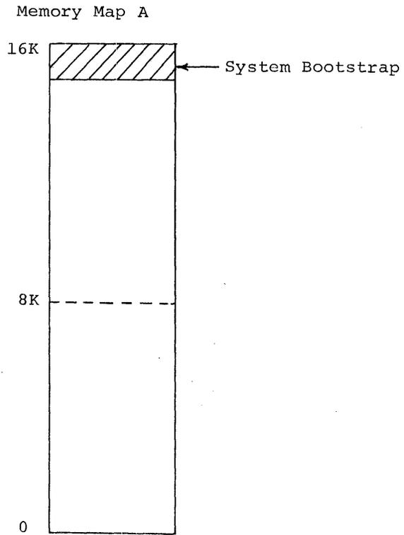
The System Bootstrap is loaded at the top of core via the paper tape reader in HRM format.
