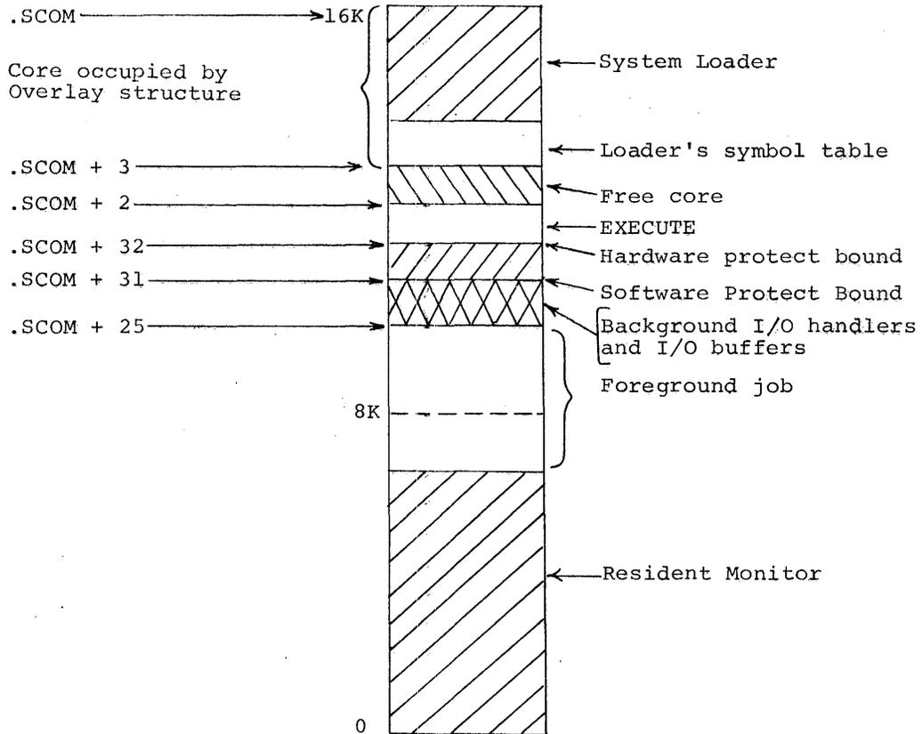
The System Loader loads EXECUTE's I/O handler (if not in core) in order to read the XCT file. The core limits of the overlay structure and the I/O requests in the .IODEV bit map are read from the XCT file. The user's I/O handlers and I/O buffers are then loaded above EXECUTE's handler, and the hardware protect bound is established above them. EXECUTE is loaded above the bound and Background free core is set up from the top of EXECUTE to the bottom of the overlay area.
