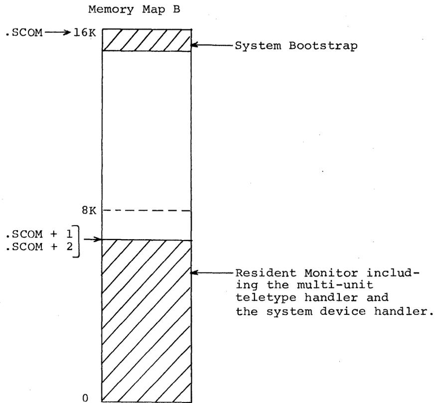
The System Bootstrap automatically loads the Resident Monitor from the system device into lower core.
