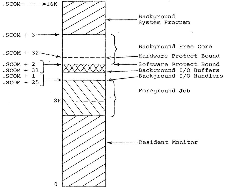
If the BACKGROUND request is for a system program, the System Loader loads the system program I/O handlers up from the top of the FOREGROUND job, allocates I/O buffer space, and loads the system program at the top of core (overlying the System Loader). Control is returned to the Resident Monitor, which sets the memory protect bound above the buffer space and given control to the system program.
