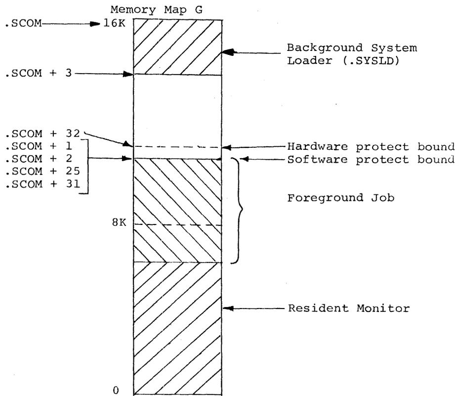
When a BACKGROUND keyboard command requests loading of a system or user program, the Non-resident Monitor brings in the System Loader, overlaying itself. Note that the BACKGROUND System Loader and the FOREGROUND Linking Loader are physically the same program.
