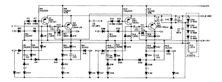
UNLESS OTHERWISE INDICATED: RESISTORS ARE 1/4W, 5% CAPACITORS ARE MMFD DIODES ARE D-664
