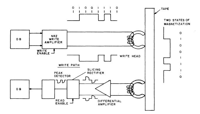
Figure 3-2 Tape Write and Read Signal Flow
