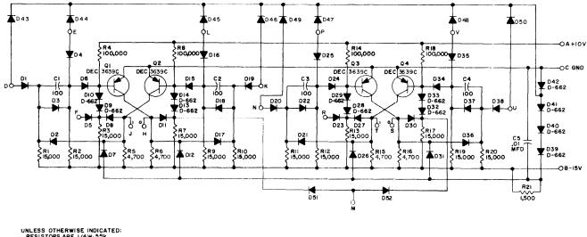
UNLESS OTHERWISE INDICATED: RESISTORS ARE 1/4W;5% CAPACITORS ARE MMFD DIODES ARE D-664
