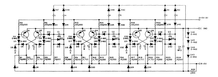
UNLESS OTHERWISE INDICATED: RESISTORS ARE 1/4 W15% CAPACITORS ARE MMFD DIODES ARE D-664 TRANSISTORS ARE DEC 3639C
