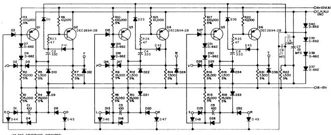
UNLESS OTHERWISE INDICATED: RESISTORS ARE 1/4W;10% CAPACITORS ARE MMFD DIDDES ARE D-664 TRANSISTORS ARE DEC 3639-0
