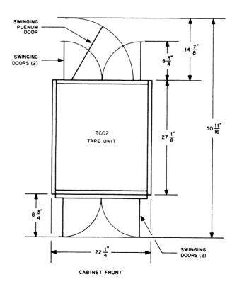
Figure 4-1 TC02 Unit Single Cabinet Installation Dimensions
