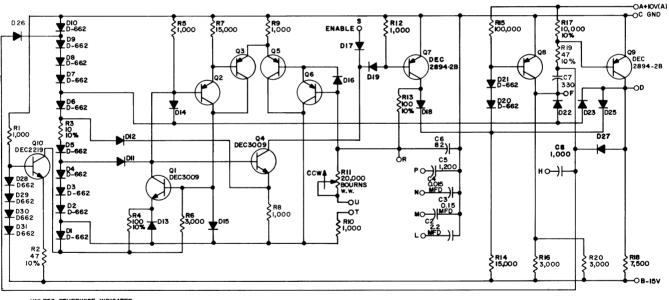
UNLESS OTHERWISE INDICATED: RESISTORS ARE 1/4 W; 5% CAPACITORS ARE MHED DODDES ARE 0-664 TRANSISTORS ARE DEC 3639-0 RII IS A #275P
