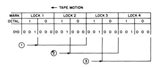
Figure 3-7 Mark-Track Decoding (MK BLK START-010)
