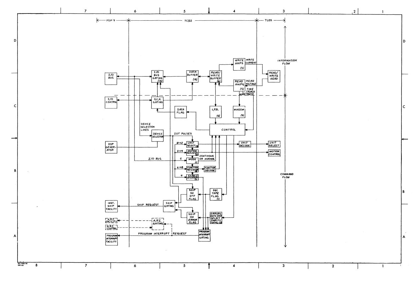
Figure 3–2 Type TC01 DECtape Control Functional Block Diagram
