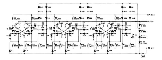
UNLESS OTHERWISE INDICATED: RESISTORS ARE 1/4 W;5% CAPACITORS ARE MMFD DIODES ARE D-664 TRANSISTORS ARE DEC 3639C
