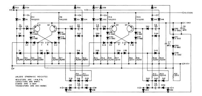
Figure 5-16 S205 Dual Flip-Flop
