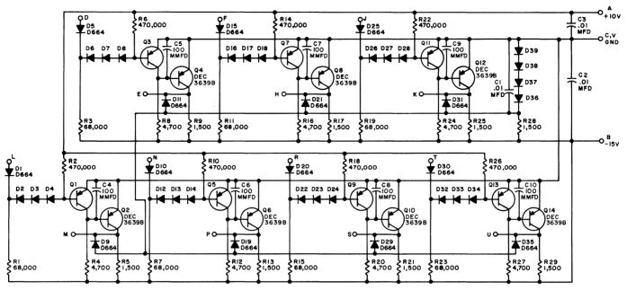
UNLESS OTHERWISE INDICATED: RESISTORS ARE 1/4W; 5% DIODES ARE D662 TRANSISTORS ARE DEC3639C
