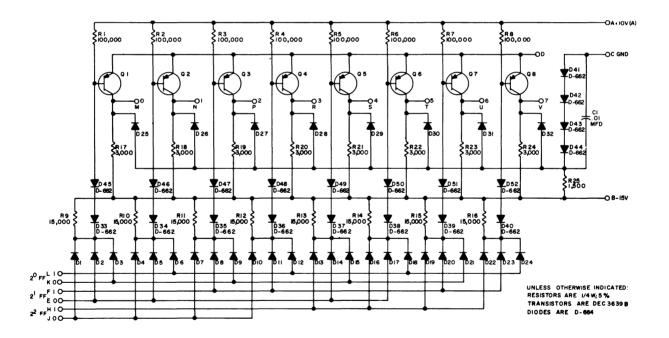
Figure 5–13 S151 Binary-to-Octal Decoder
