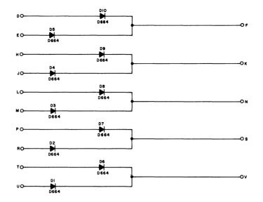
Figure 5-4 R002 Diode Network
