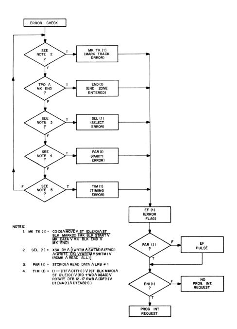
Figure 3-10 Error Check Flow Diagram
