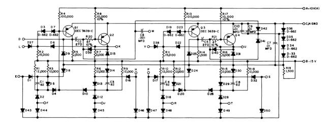
UNLESS OTHERWISE INDICATED: RESISTORS ARE 1/4W; 5% CAPACITORS ARE MMFD DIODES ARE D-664 TRANSISTORS ARE DEC2894-2B
