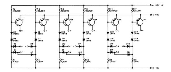
UNLESS OTHERWISE INDICATED: TRANSISTORS ARE DEC3639 RESISTORS ARE 1/4W, 5% DIODES ARE D664
