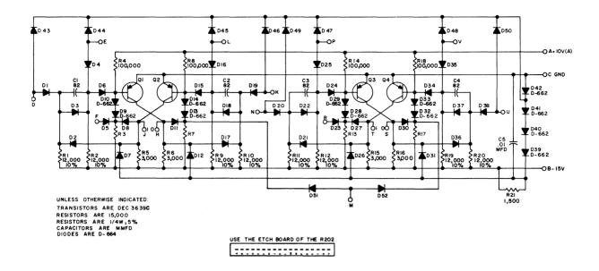
Figure 5-14 S202 Dual Flip-Flop
