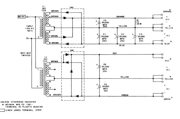
Figure 5-25 Power Supply Type 779, Schematic Diagram
