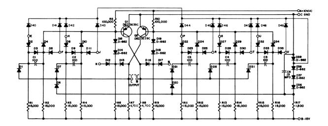
UNLESS OTHERWISE INDICATED: RESISTORS ARE 1/4W; 5 % CAPACITORS ARE MMFD DIODES ARE D-664
