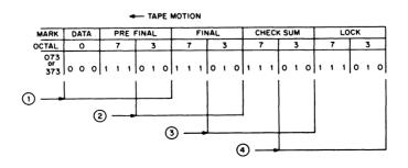
Figure 3-9 Mark-Track Decoding (MK BLK END)
