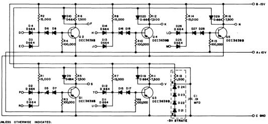
UNLESS OTHERWISE INDICATED: RESISTORS ARE 1/4 W, 5% DIODES ARE D 662
