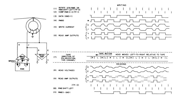
Figure 3-3 Read/Write Logic and Waveforms
