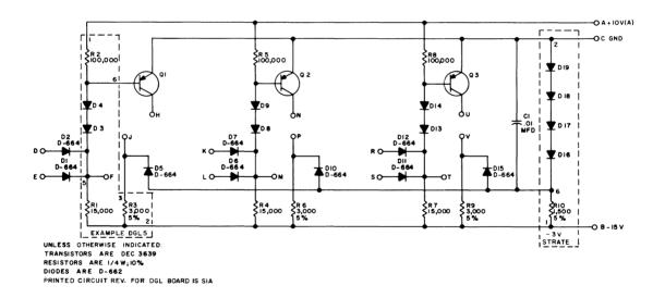
Figure 5-11 S111 Diode Gate
