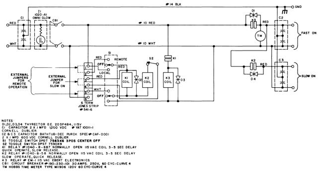
Figure 5-26 Power Control Panel Type 832F
