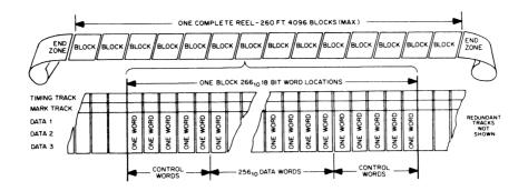
Figure 2-3 Control and Data Word Assignments
