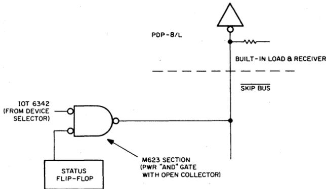
Figure 27. Use of IOS to Test the Status of an External Device
