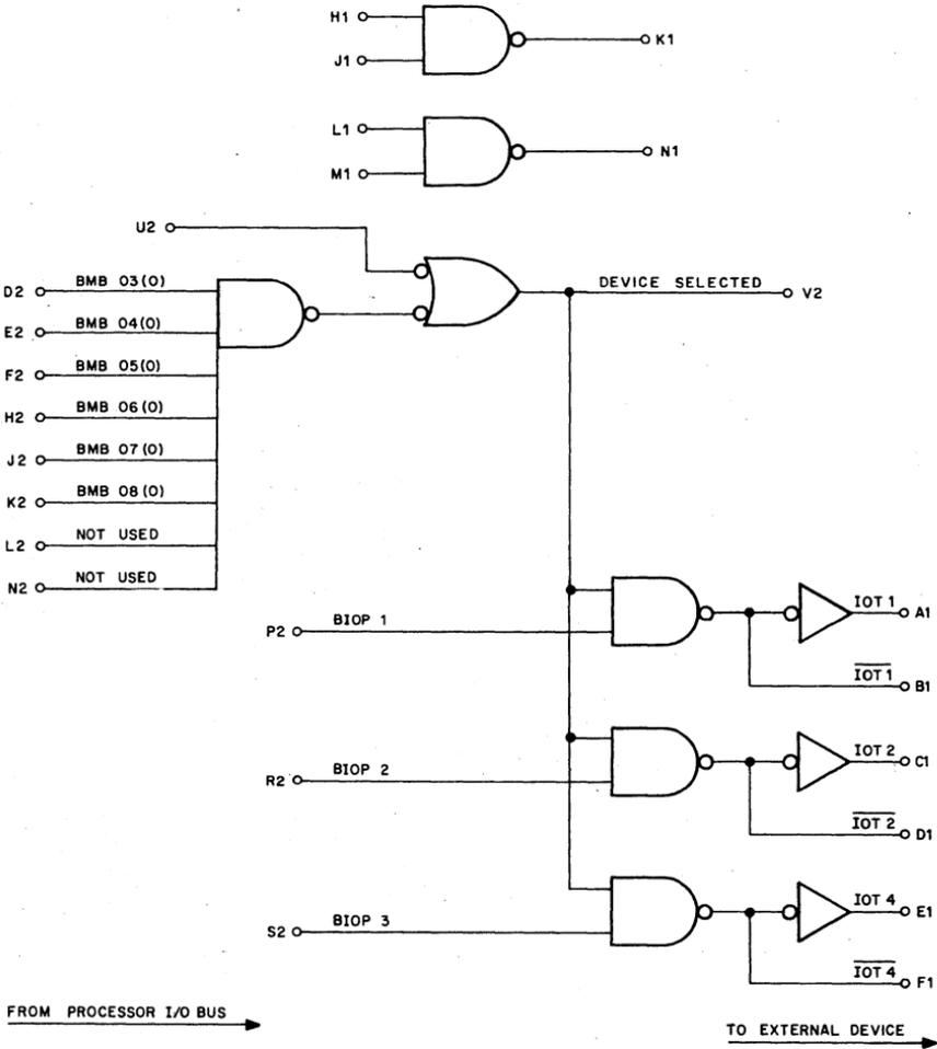
Fig. 47 M103 Device Selector Logic Circuit
