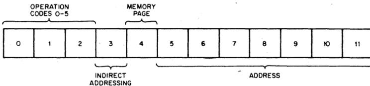
Figure 6. Memory Reference Instruction Bit Assignments
