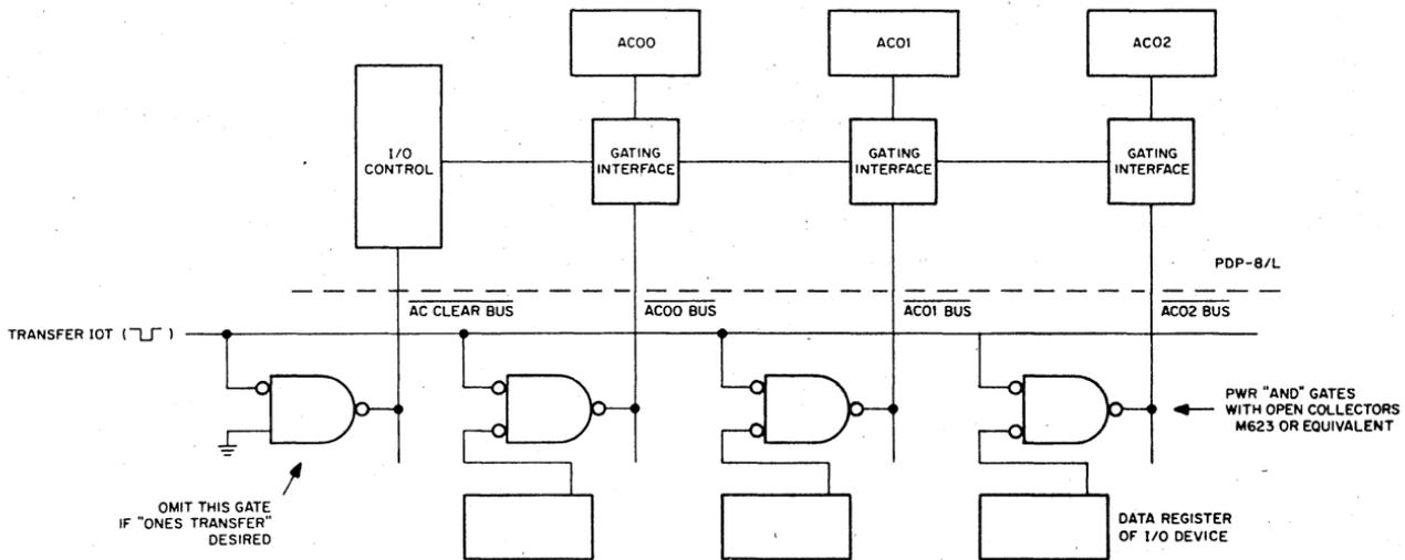
Figure 29. Loading Data into the Accumulator from an External Device
