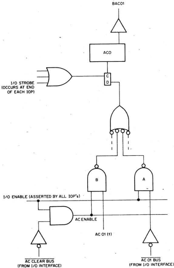
Figure 28. Accumulator Input and Output
