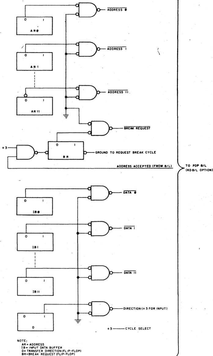
Figure 36. Device Interface Logic for Single-Cycle Data Break Input Transfer
