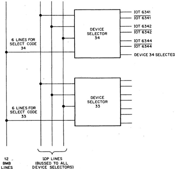
Figure 25. Generation of IOT Command Pulses by Device Selectors
