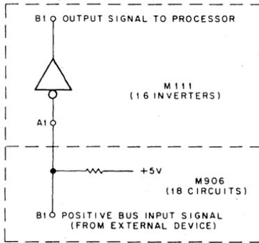
Fig. 43 Typical M111/M906 Positive Input Circuit
