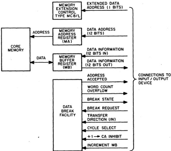
Figure 34. Data Break Transfer Interface Block Diagram
