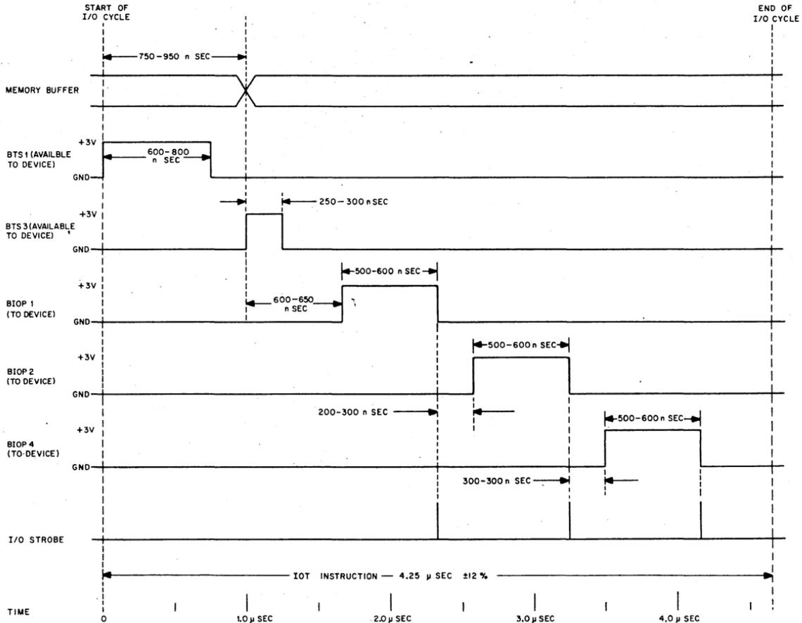
Figure 22. Programmed Data Transfer Timing
