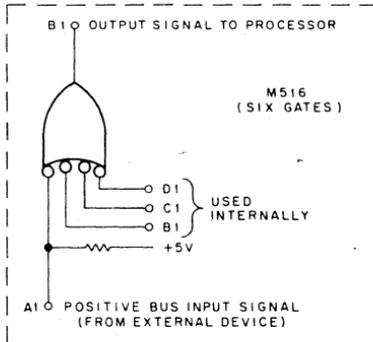
Fig. 44 Typical M516 Positive Bus Receiver Input Circuit
