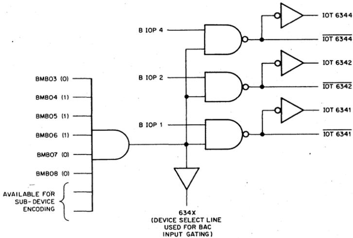
Figure 26. Typical Device Selector (Device 34)
