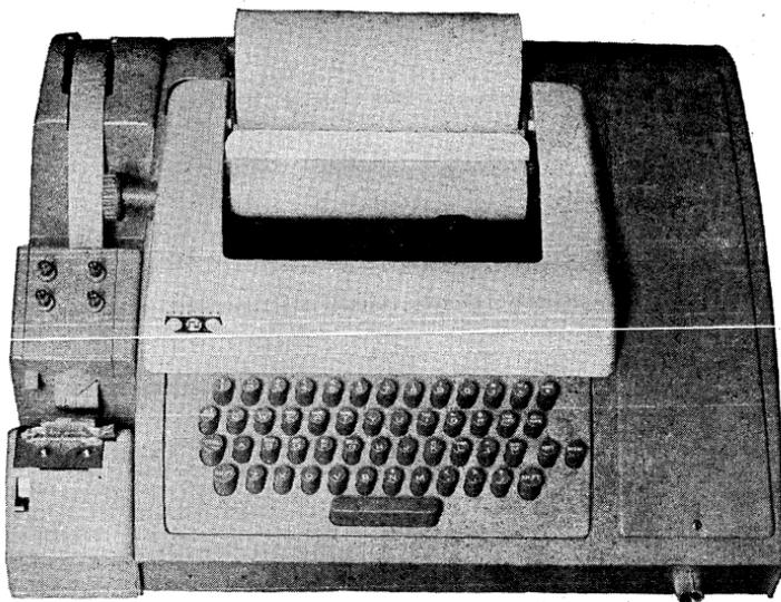
Figure 5. Teletype Model 33 ASR Console
