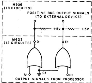
Fig. 45 Typical M623/M906 Positive Output Circuit
