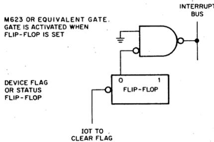
Figure 32. Program Interrupt Request Signal Origin
