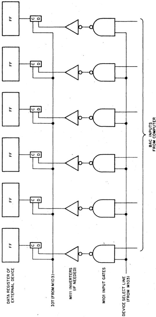
Figure 30. Loading a 6-Bit Word into an External Device from the Accumulator
