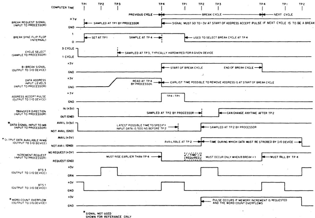
Figure 40. Memory Increment Data Break Timing Diagram
