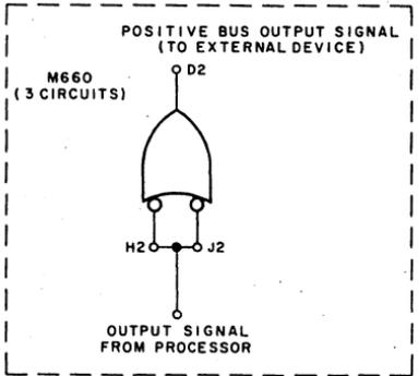
Fig. 46 Typical M660 Bus Driver Output Circuit
