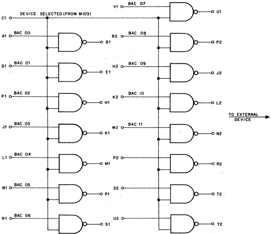
Fig. 48 M101 — Bus Data Interface Logic Circuit
