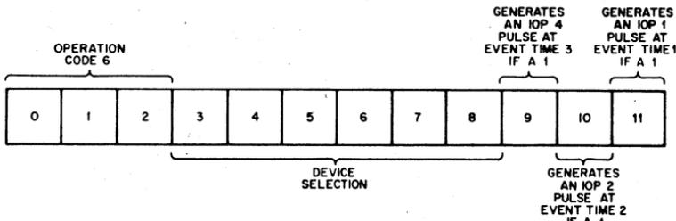
Figure 7. IOT Instruction Bit Assignments
