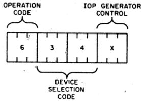
Figure 23. Typical IOT Instruction Decoding
