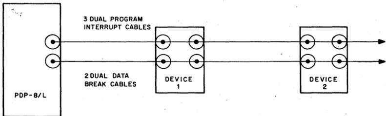
Fig. 49 I/O Bus Configuration
