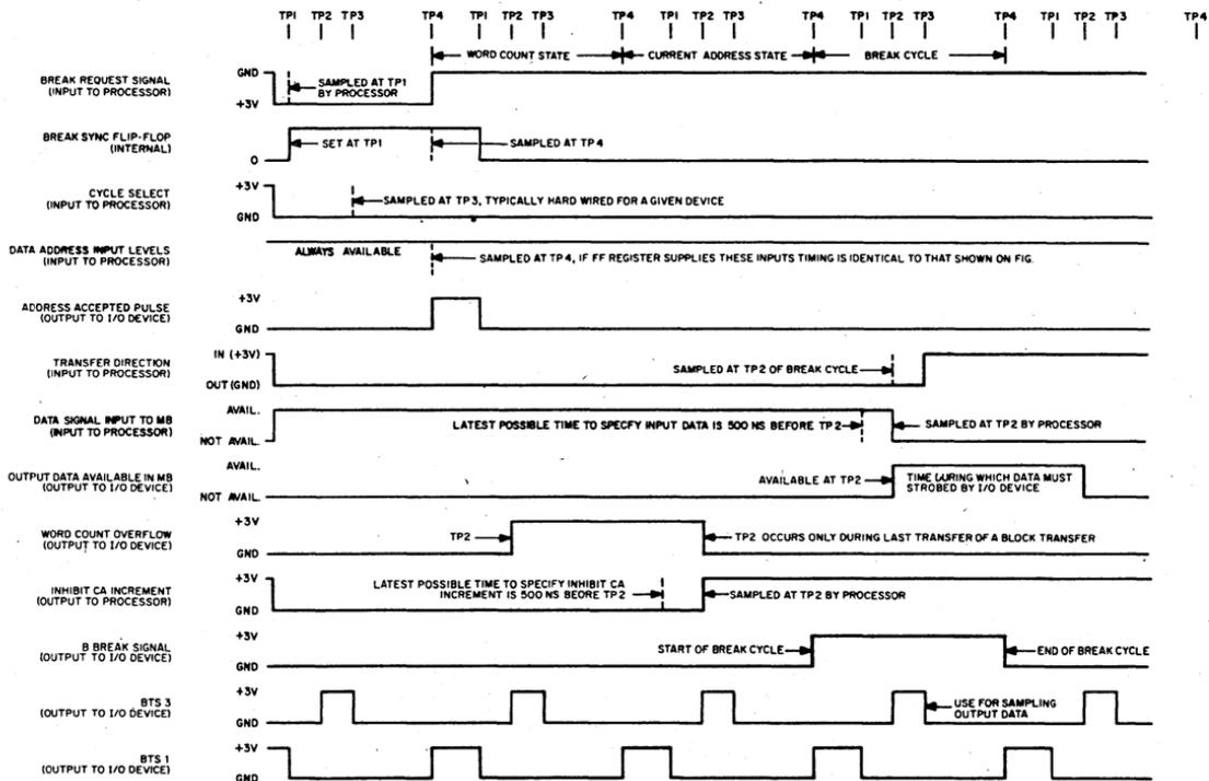
Figure 42. Three-Cycle Data Break Timing Diagram
