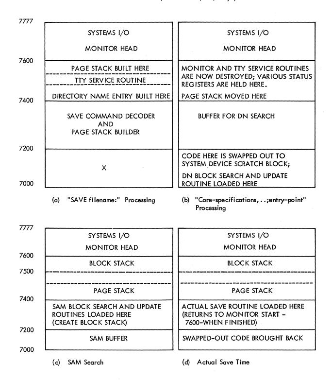
Figure B-9 Core Usage During SAVE Command Execution
