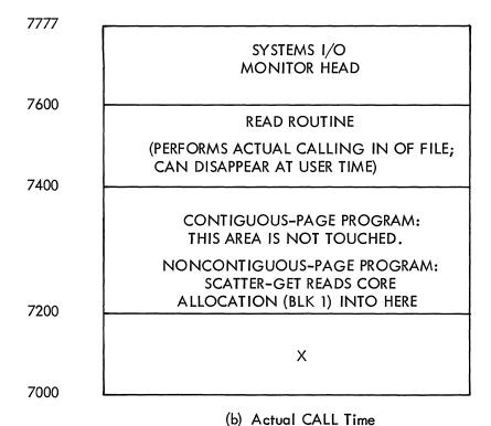
Figure B-10 Core Usage During CALL Command Execution
