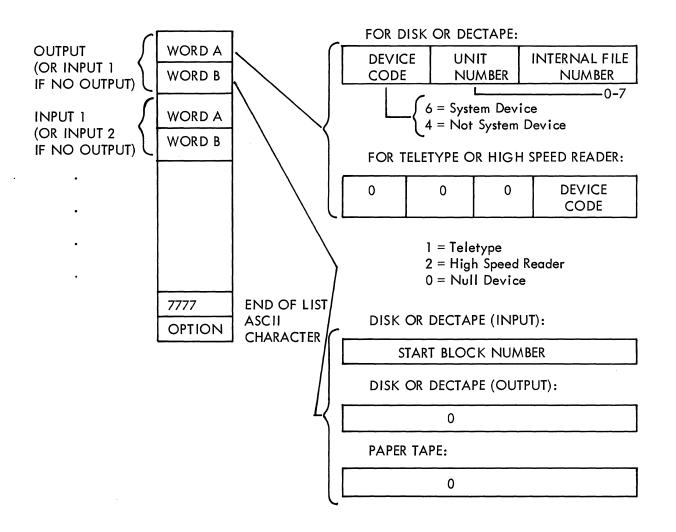
Figure C-1 Output List Produced by Command Decoder
