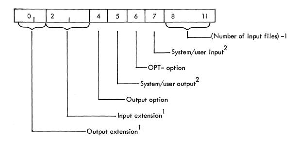
This option word must be set up by the system program before calling Command Decoder.
