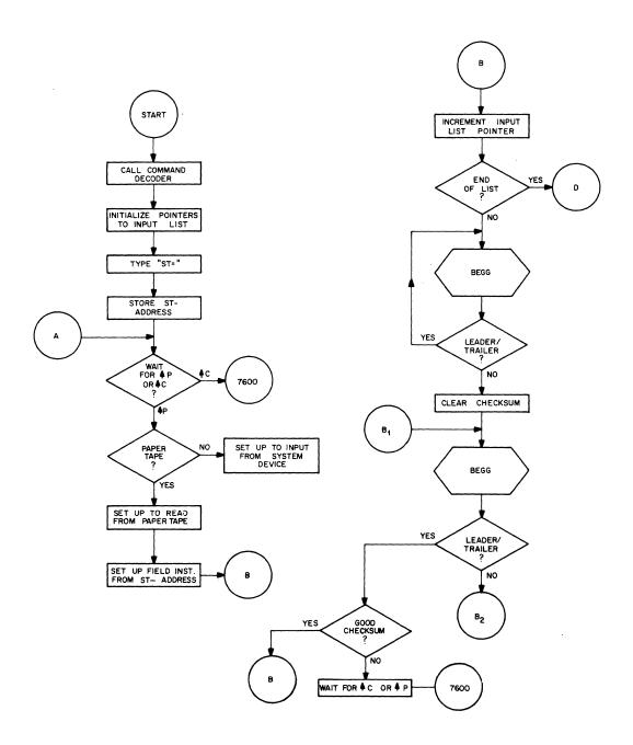
Figure D-1 Binary Loader Flow Chart (Part 1)
