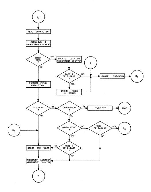
Figure D-1 Binary Loader Flow Chart (Part 2)
