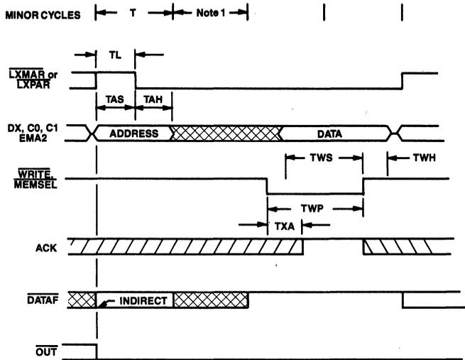
NOTE 1: This cycle is deleted on PAC1, PAC2, PPC1, PPC2 and control panel Interrupt writes.
