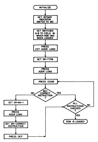
Figure A-2. Checking the RIM Loader
