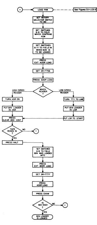
Figure A-3 Loading the BIN Loader
