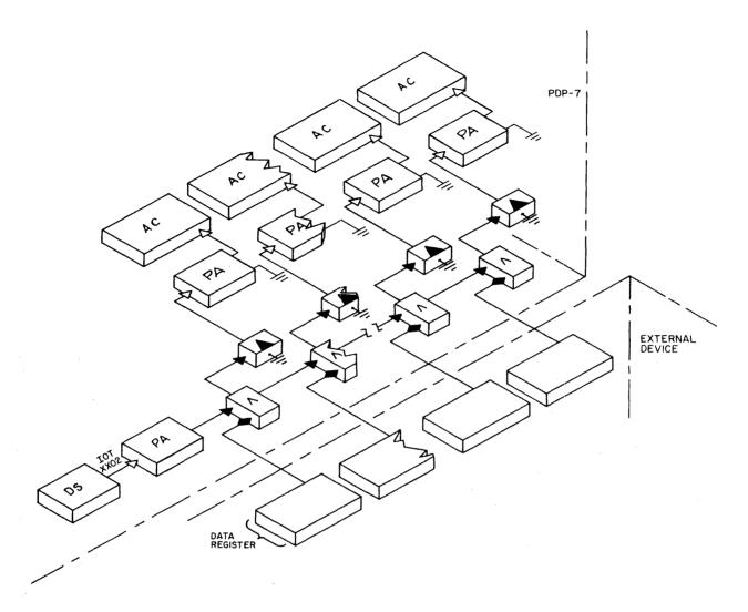
Figure 12 Programmed Data Input Transfer
