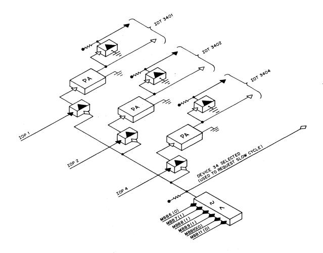
Figure 8 Typical Device Selector (Device 34)
