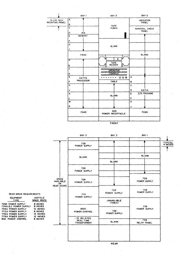
Figure 29 Basic PDP-7 Component Locations
