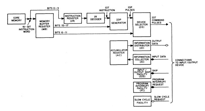
Figure 3 Programmed Data Transfer Interface Block Diagram
