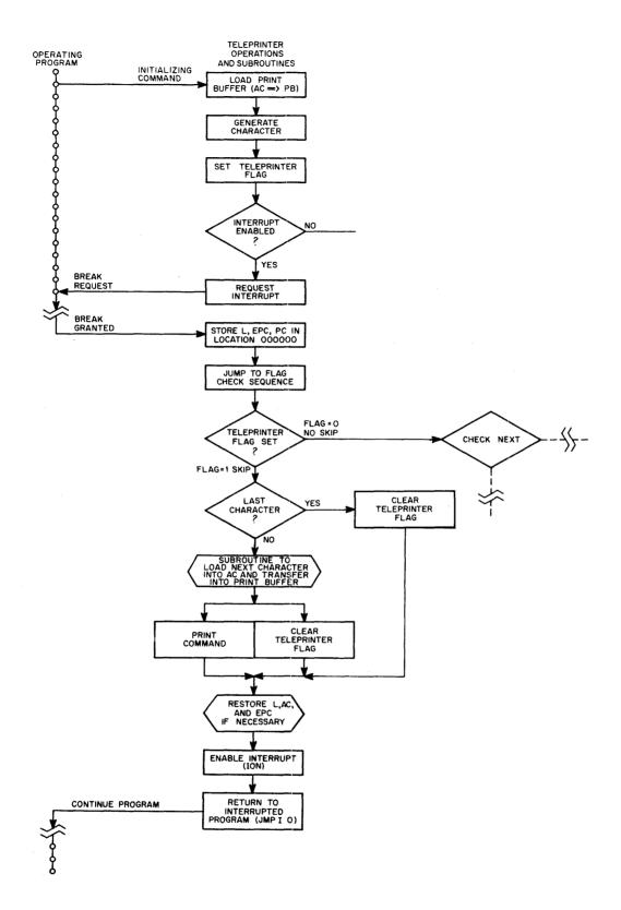
Figure 17 Programmed Data Output Flow Diagram
