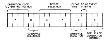
Figure 4 Decoding of IOT Instructions
