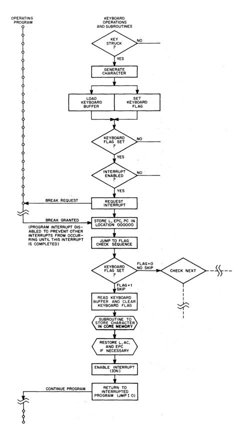
Figure 16 Programmed Data Input Flow Diagram
