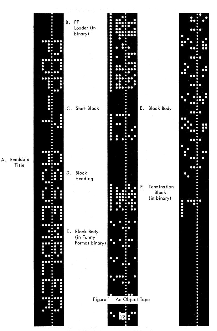
If the FF Loader is expected to be in memory when the object tape is loaded, the pseudo-instruction NOINPUT can be used to instruct the Assembler to suppress punching of the loader and punch instead a JMP 17600, the starting address of the FF Loader. A tape in this form may be loaded by the loading commands in DDT-7 as well as through a FF Loader already in memory.
