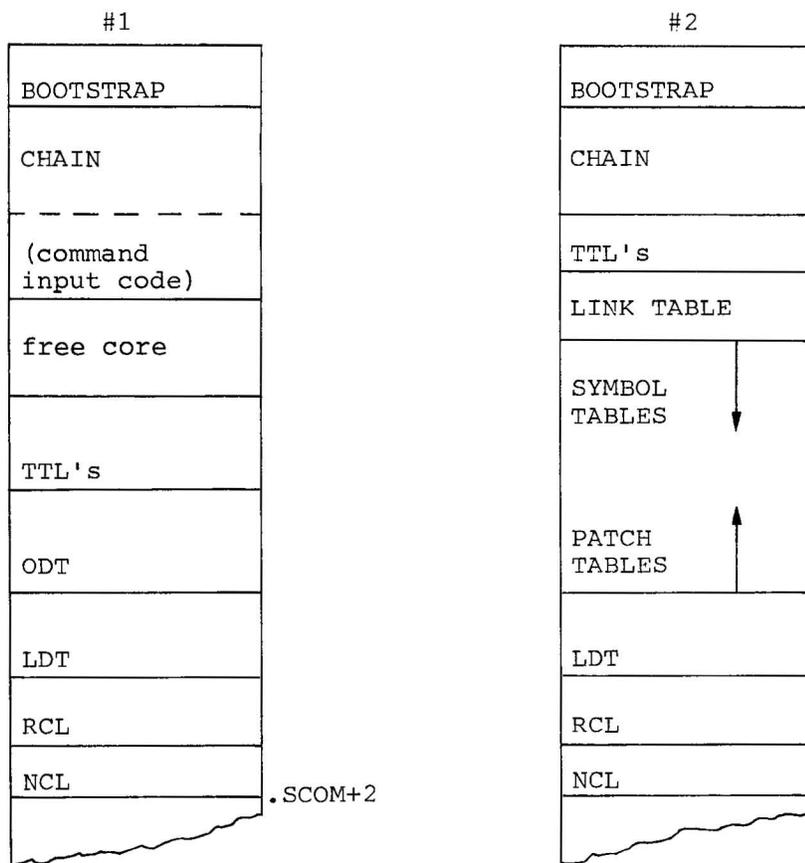
The core used the NCL (Named Common List, generated by the use of the VTC and RES options), the RCL (Resident Code List), and the LDT (Link Definition Table), and ODT (Overlay Description Table), and the TTL's (Trunk-to-Twig Lists) is shown here to help when reading the program listing. This information is not necessary for the proper usage of CHAIN.
