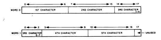
Figure 1-7. 5/7 ASCII Packing Scheme
