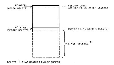
Figure 2-11. Line Buffer After DELETE Command
