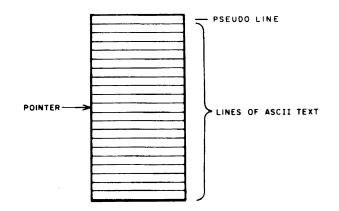
Figure 2-1. Line Buffer and Software Pointer
