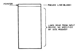
Figure 2-3. Line Buffer After READ Command
