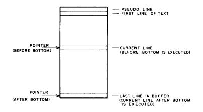
Figure 2-9. Line Buffer After BOTTOM Command
