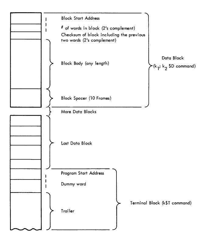
Figure 3-1. PDP-15/10 Loader Format (cont)
