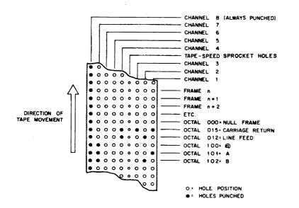
Figure 2-2. PDP-15/10 ASCII Tape Format
