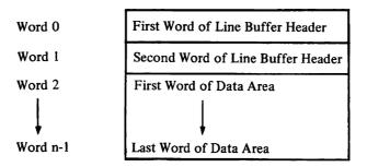
Figure 1-4. Line Buffer Structure
