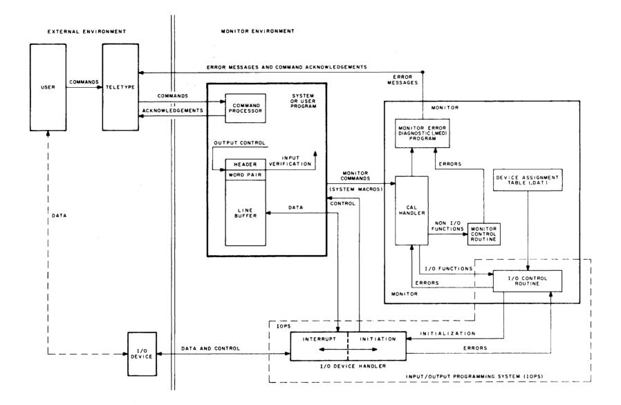
Figure 1-2. Command, Control, and Data Flow in the Basic I/O Monitor Environment
