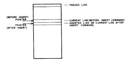
Figure 2-10. Line Buffer After INSERT Command
