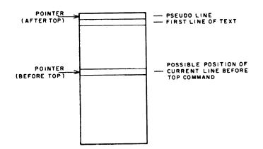
Figure 2-5. Line Buffer After TOP Command
