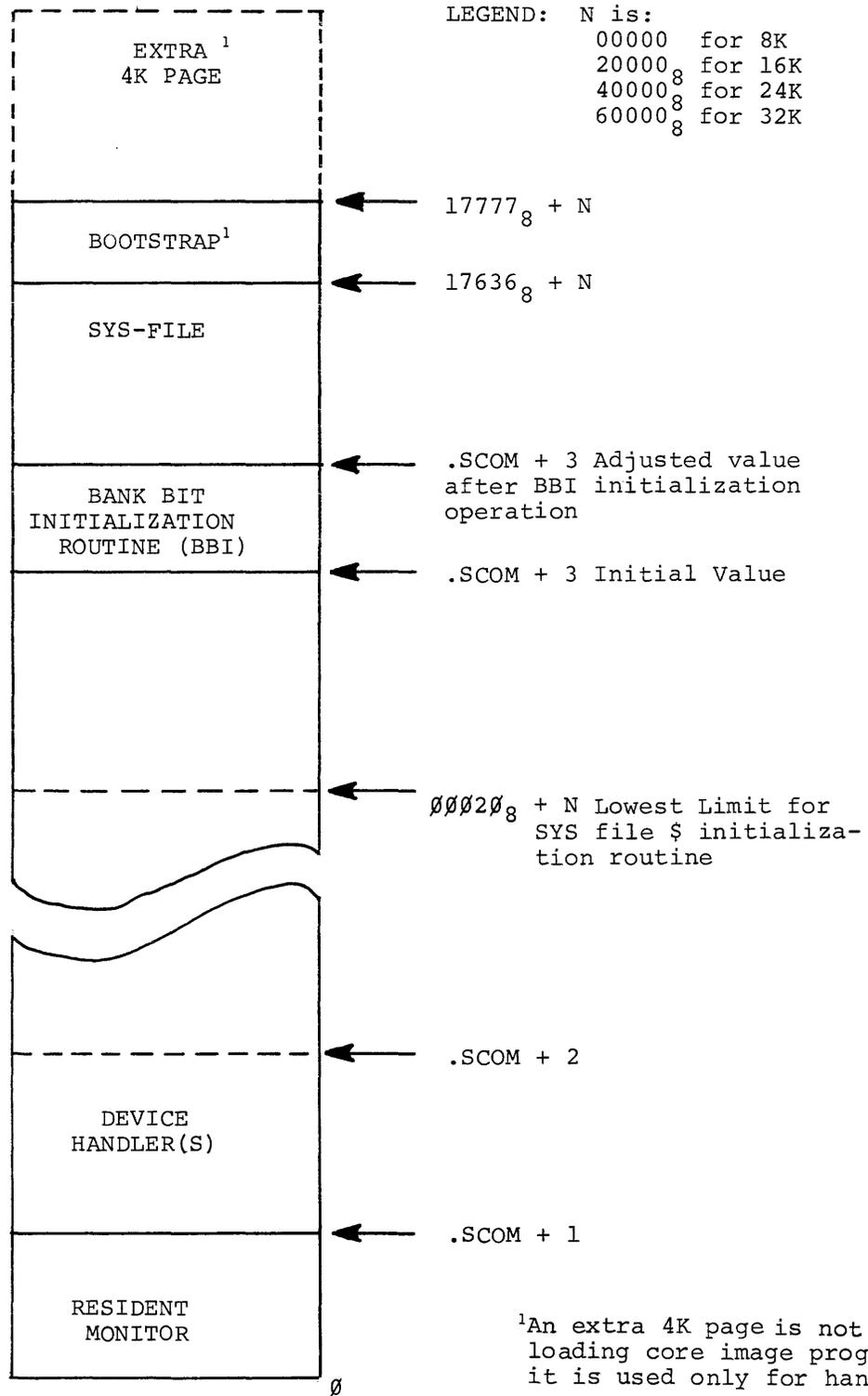
Figure 3-1, Memory Map, Loading a READR-Installed SYS-file on the ADSS Monitor
