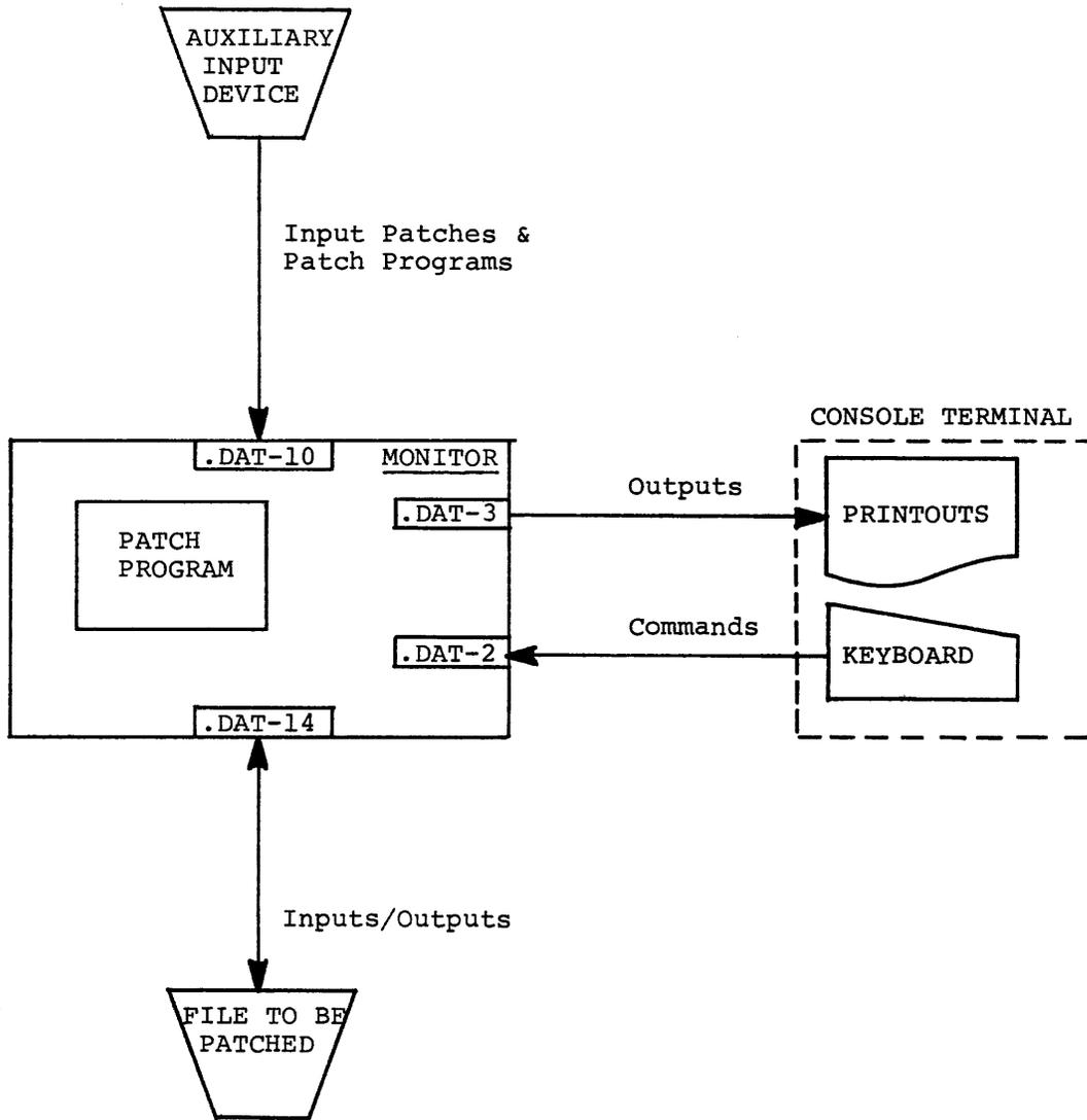
Figure 1-1 PATCH Operations, Information Flow Diagram
