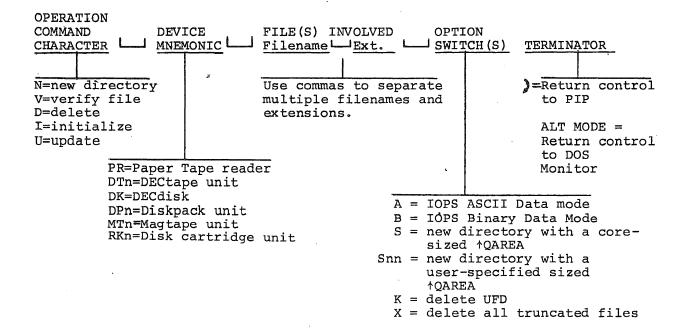
Figure 6-3 PIP Single Device Commands, General Format
