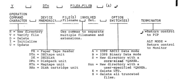
Figure 2-2. PIP Single Device Commands, General Format
