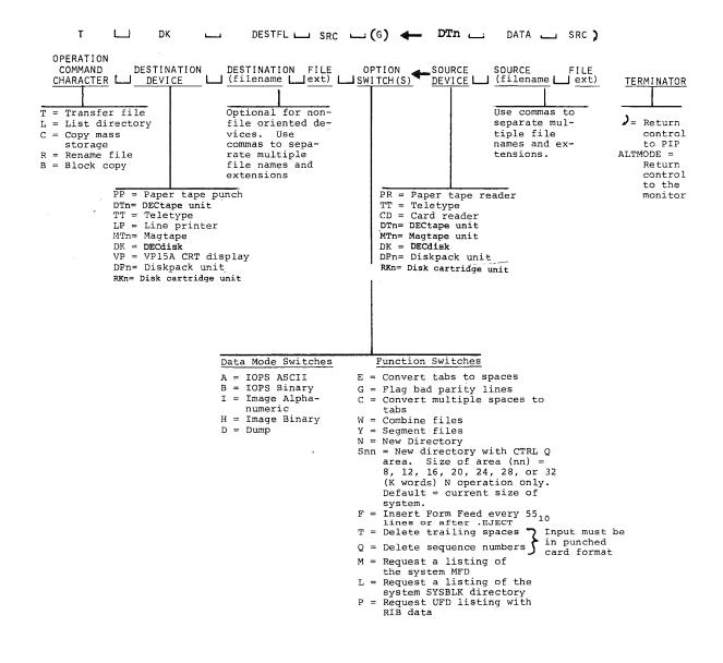
Figure 6-2 Destination/Source Command String Format
