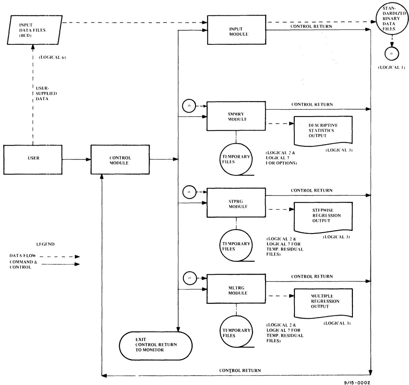
Figure 1-1 STATPAC Logic Modules, Flow Diagram
