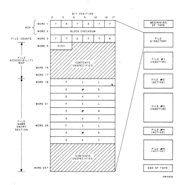
Figure 6-4a. Format of the File Directory Data Block, showing relationship of active and inactive files to file name entries and to Accessibility Map
