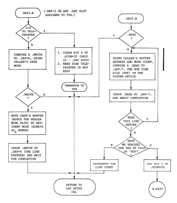
Processing for I/O Macros addressed to .DAT slots -2 or -3, or any slot assigned to TTA. Points within the Resident Monitor which transfer control to Resident BOS-15.
