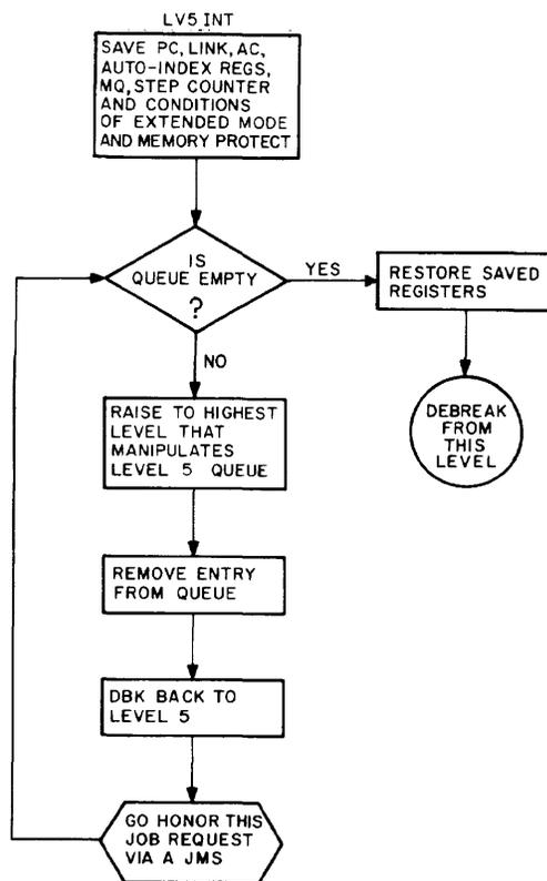
Figure 5-4 Structure of API Software Level Handler
