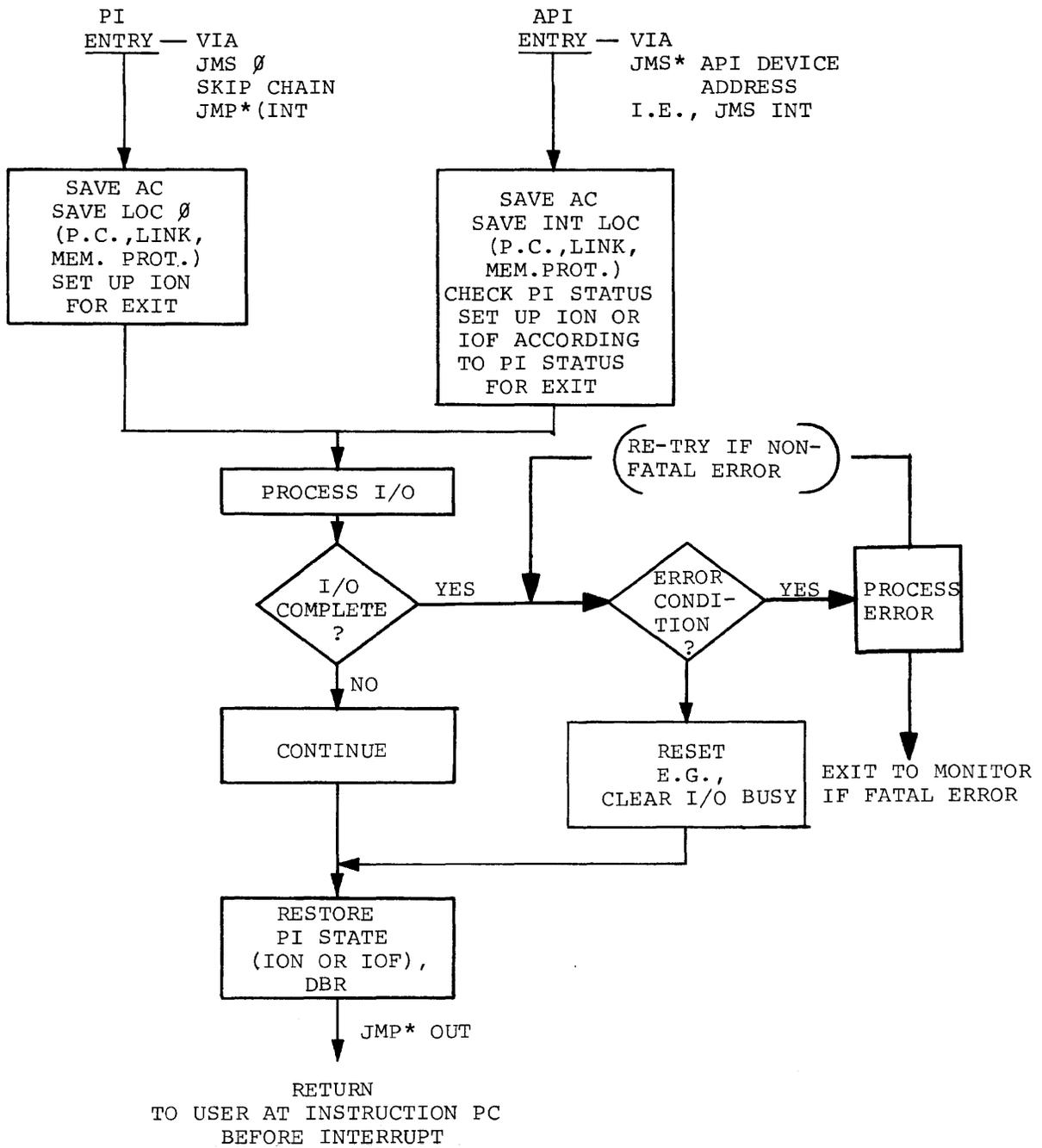
Figure 5-3, PI and API Entries to Device Handlers
