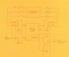
The input (I) boxes and output (O) boxes provide an interface or buffer between the 115 VAC control signals (or DC level) from the controlled device and the PDP-14 control unit.
