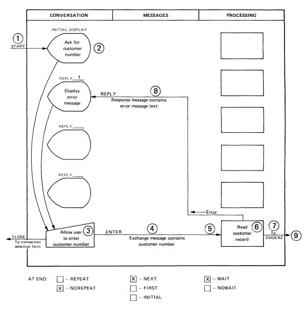
Figure 1-2 Transaction Structure Diagram for "CHGCUS"
