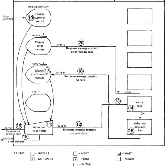
Figure 1-2 (cont.) Transaction Structure Diagram for "CHGCUS"
