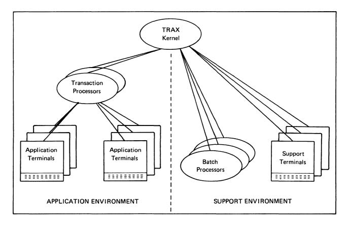
Figure 1-4 TRAX System Structure
