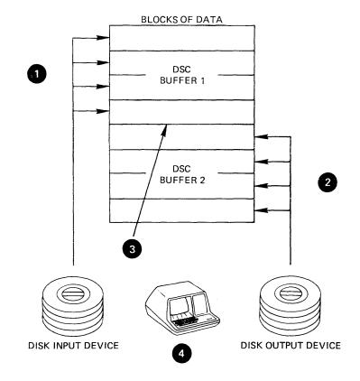
DSC reads four blocks (default) of data from the disk input device to a buffer.
