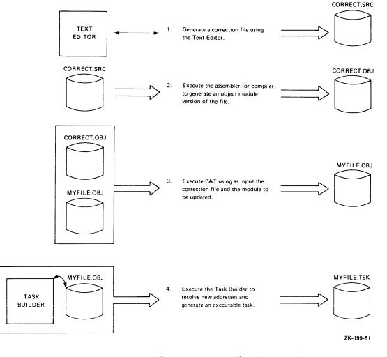
Figure 14-1 Processing Steps Required to Update a Module Using PAT
