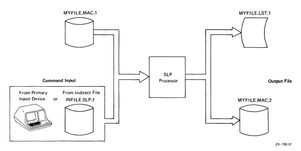
Figure 13-1 Input Files and Output Files Used During SLP Processing
