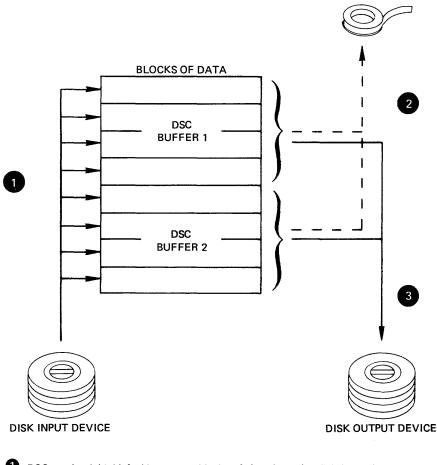
DSC reads eight (default) or more blocks of data from the disk input device to two buffers.
