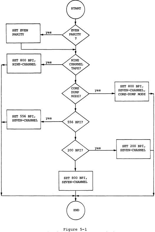
Figure 5-1 Determination of Tape Characteristics for the TU10
