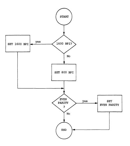
Figure 5-2 Determination of Tape Characteristics for the TU16
