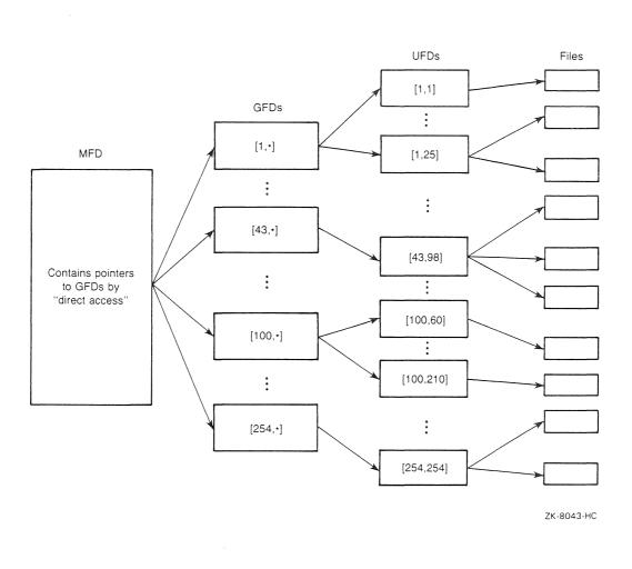
As Figure 1–2 shows, the MFD contains pointers to the Group File Directories (GFDs). The GFDs point to UFDs within each group. For example, a pointer in the MFD could access the GFD for files in [43,\*] directories, from which it could access a specific UFD, such as [43,98].
