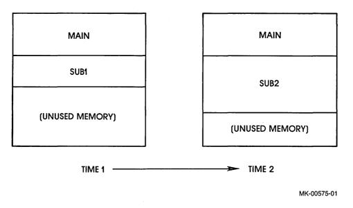
Figure 8-2: A Simple Overlay in Memory
