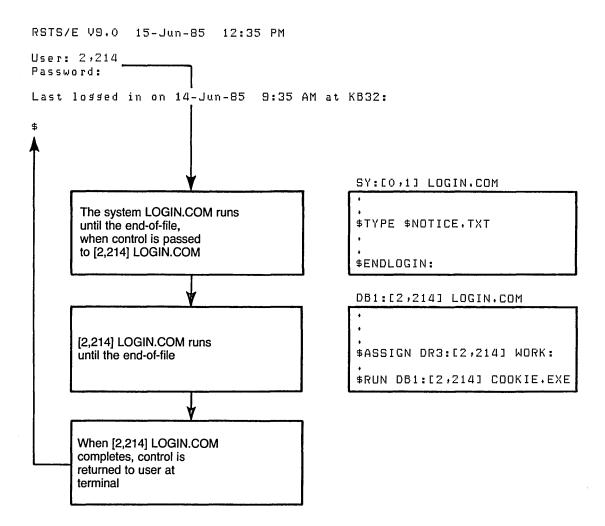
Figure 1-1: Executing System and User Login Files
