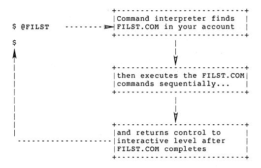
Figure 1-1: Executing a Command Procedure at Interactive Level
