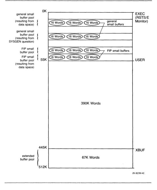
The RSTS/E monitor uses general small buffers as a temporary storage area for such things as:
