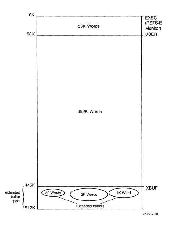
Figure 7: Extended Buffer Pool for Example RSTS/E System
