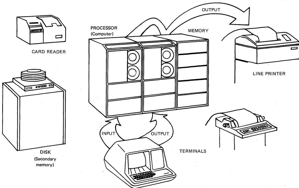
Figure 3-1 A Configuration of Devices
