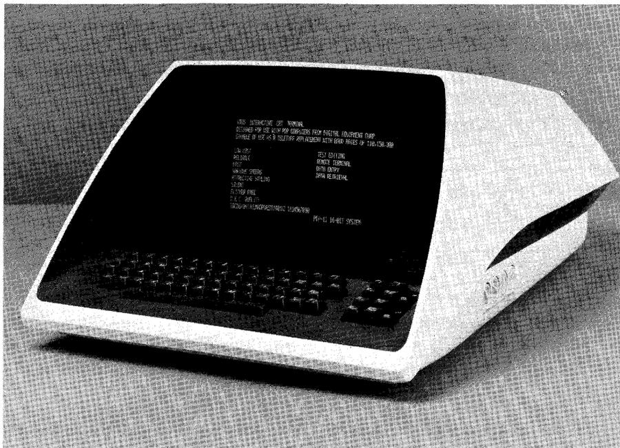
Figure 23-12 VT05 Alphanumeric Display Terminal
