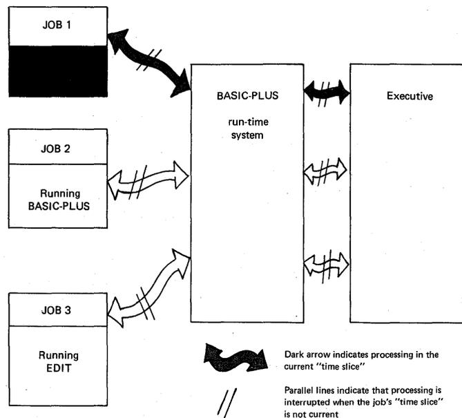
Figure 1-2 The Timesharing Process
