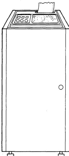
Figure 23-5 LP11 Line Printer System (80-column model)
