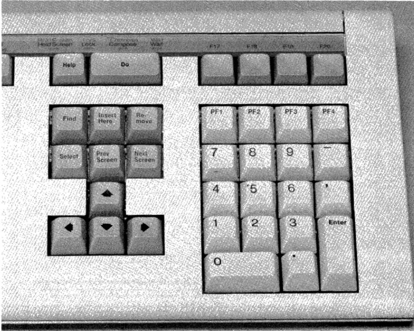
*Screen/Cursor Control Keys.* The location of the screen and cursor control keys allows fast, productive editing with the right hand, while the left hand remains in the typing area. The four keys that control cursor movement are arranged in a handy “inverted T” formation for fast cursor positioning with minimum finger motion. Each key is clearly labeled with an arrow.
