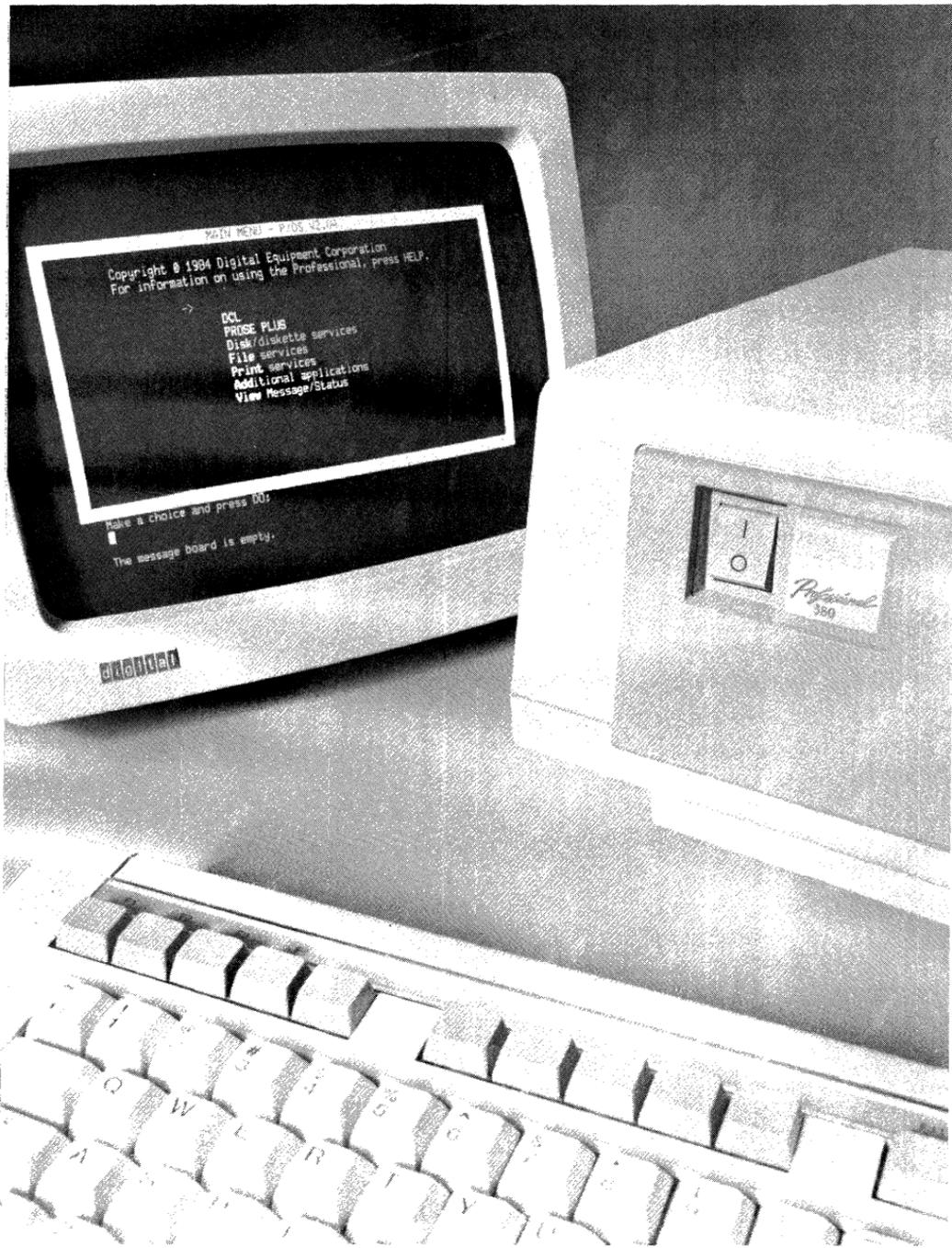
The Professional Series consists of three models: the Professional 325, the Professional 350, and the Professional 380. All feature Digital's highly acclaimed keyboard, a high-resolution monochrome or color monitor, a PDP-11-based CPU with floating-point processor, bit-mapped graphics, 512 Kbytes of main memory, an 800-Kbyte dual-diskette drive, and communications, printer, and network interconnect ports.
