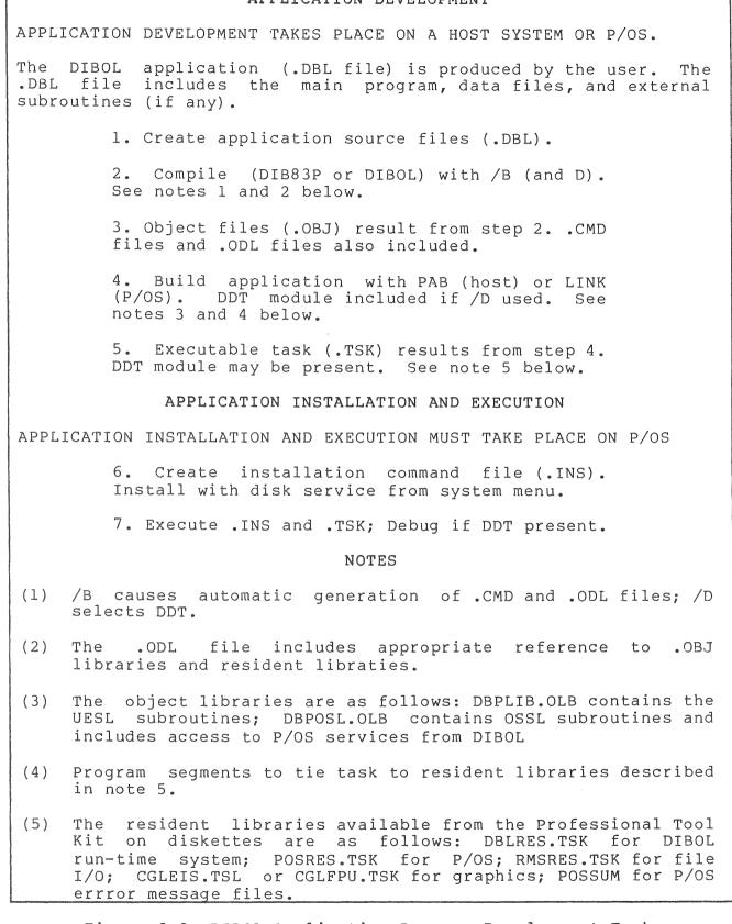
Figure 2-2 DIBOL Application Program Development Tasks
