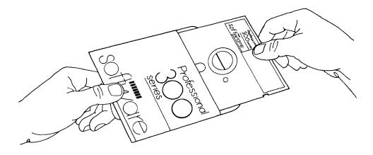
2. Push the diskette drive door until it springs open. The illustration shows how to open the door labeled 1.
