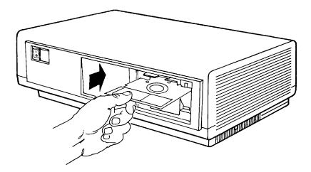
5. Press the diskette drive door closed. (Make sure the diskette is completely in before you close the door.)
