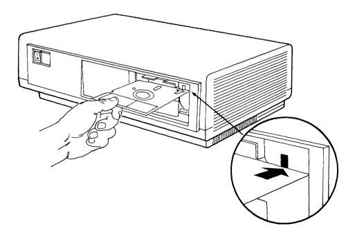
4. Gently insert the diskette all the way into the drive slot. Do not force it into the drive.
