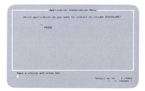
This menu lists the name(s) of the application(s) on any inserted diskettes. BIGVOLUME is the name P/OS uses for the disk.
