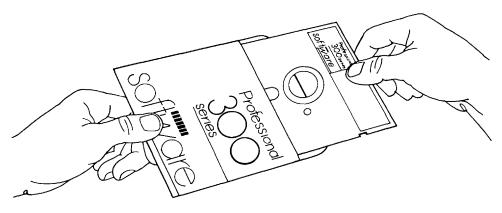
Figure 2-1 Removing a Diskette from Its Envelope
