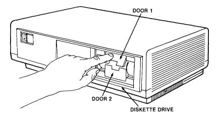
3. Match the orange arrow on the diskette with the orange stripe on the side of the diskette slot in the drive. (A diskette goes into slot 2 "upside-down" compared to the way it goes into slot 1.)
