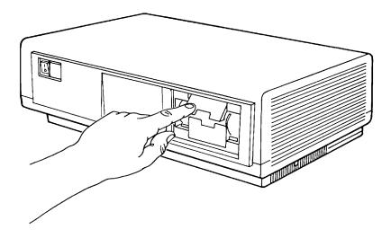
(If you put a diskette in with the wrong side up and then switch on the power, you may see a display like that in Figure 2-4. In this case, remove the diskette, and put it back in the right way.)
