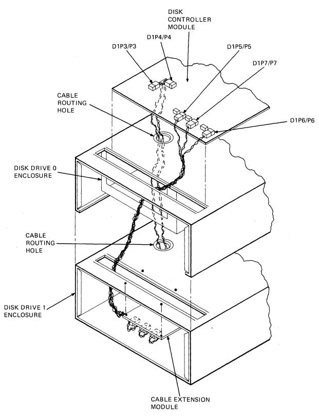
Figure 4-8 Disk Drive 1 Assembly, Cable Routing
