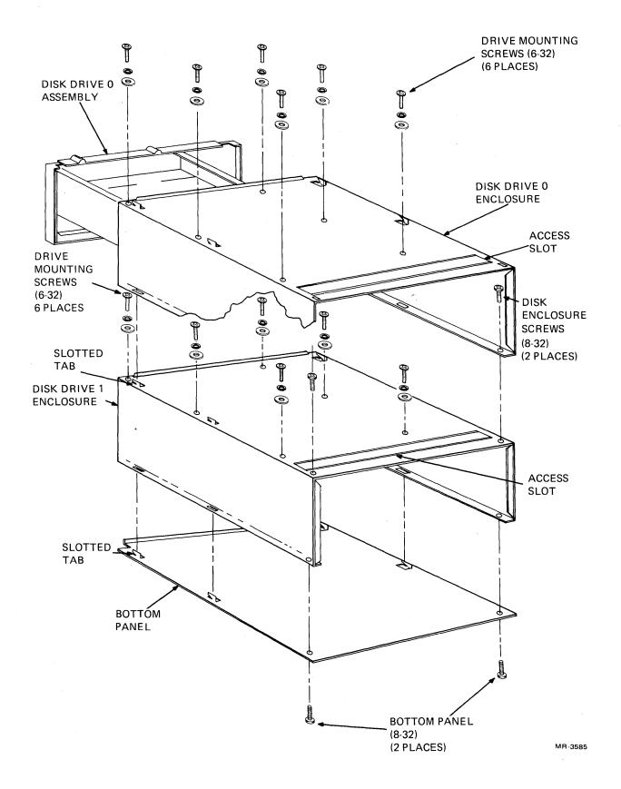
Figure 4-5 Disk Drive 1 Enclosure Mounting
