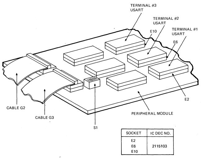
Figure 4-11 Cluster EIA Module, USART Installation
