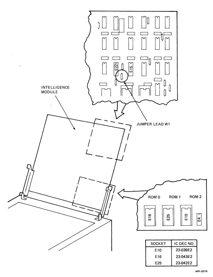
Figure 4-12 Intelligence Module, W1 Jumper Lead Location
