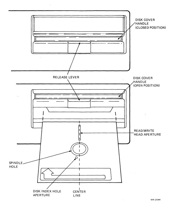
Figure 3-3 Loading the Disk into the Drive
