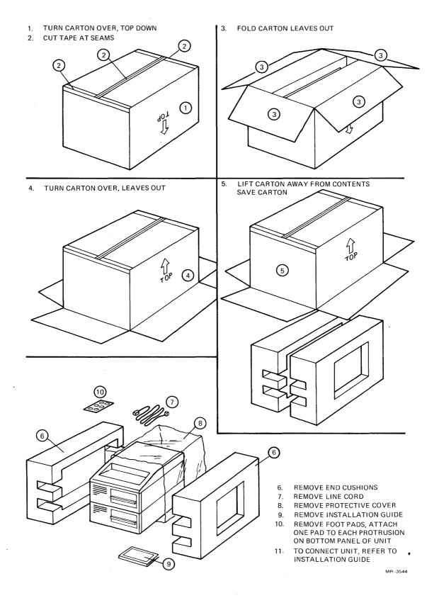
Figure 2-1 PDT-11/150 Unpacking Procedure Diagram
