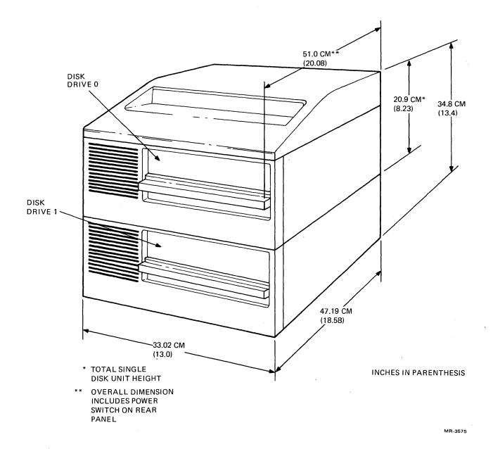
Figure 2-2 PDT-11/150 Single and Dual Disk Unit Dimensions
