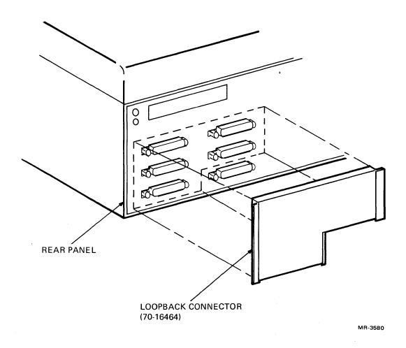
Figure 3-4 Loopback Connector Installation
