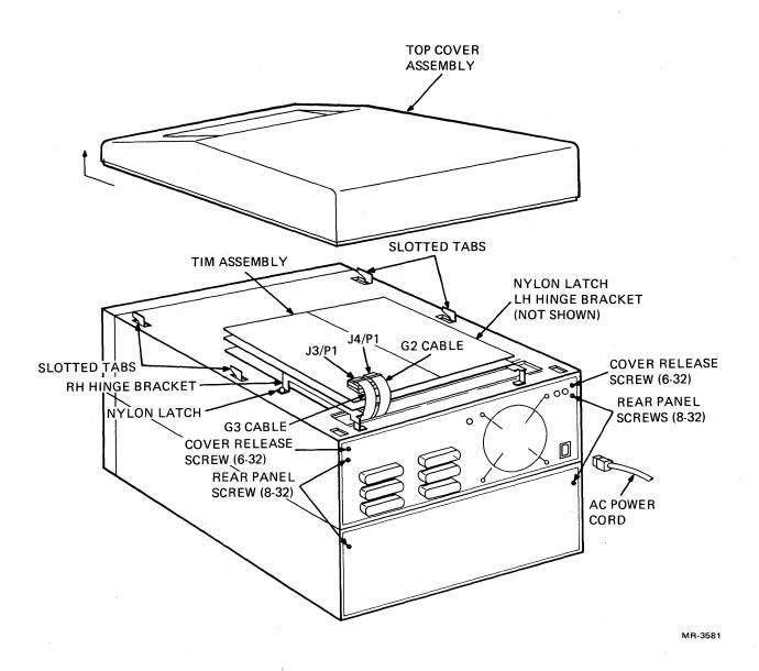
Figure 4-1 Top Cover and TIM Assembly Removal and Replacement
