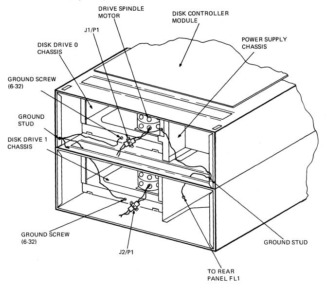
Figure 4-7 Ground Leads and ac Cable Routing
