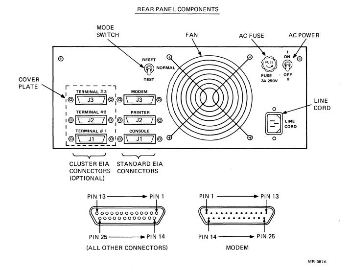
Figure 2-3 Rear Panel Components and Connector Pin Assignments
