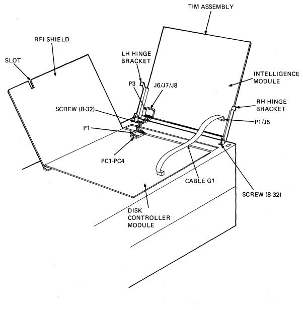
Figure 4-2 TIM Assembly Connections
