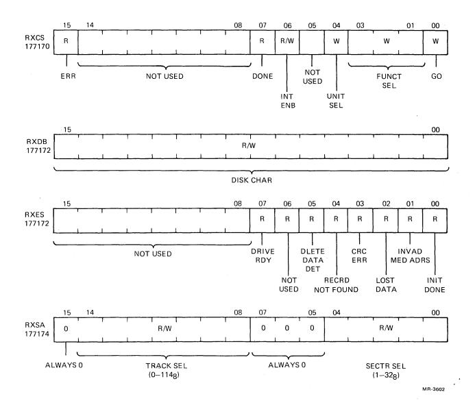
Figure 5-10 Disk Drive Interface, Register Formats
