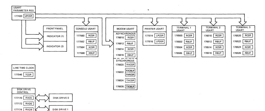
Figure 5-2 PDT-11/150 Control and Address Register, Buffer Assignments
