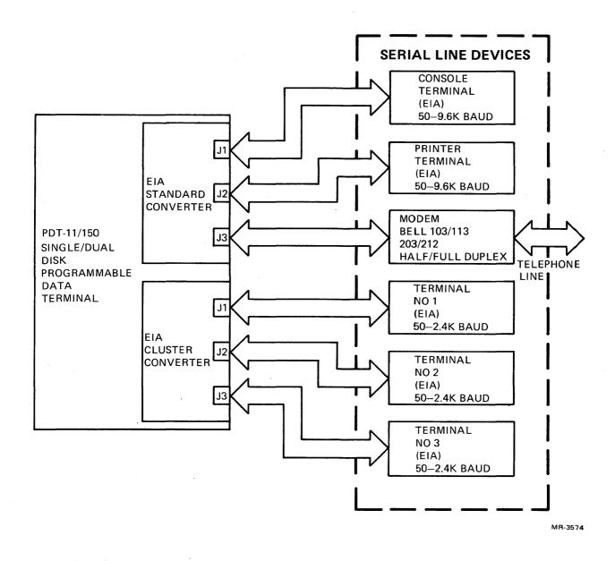
Figure 1-1 Typical PDT-11/150 Flexible Disk Operating System
