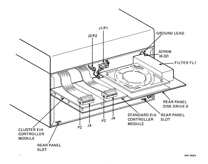
Figure 4-6 Rear Panel Removal, Disk Drive 0 Enclosure
