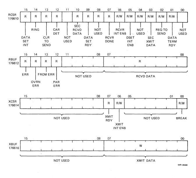
Figure 5-6 Asynchronous Communications Interface Register Formats
