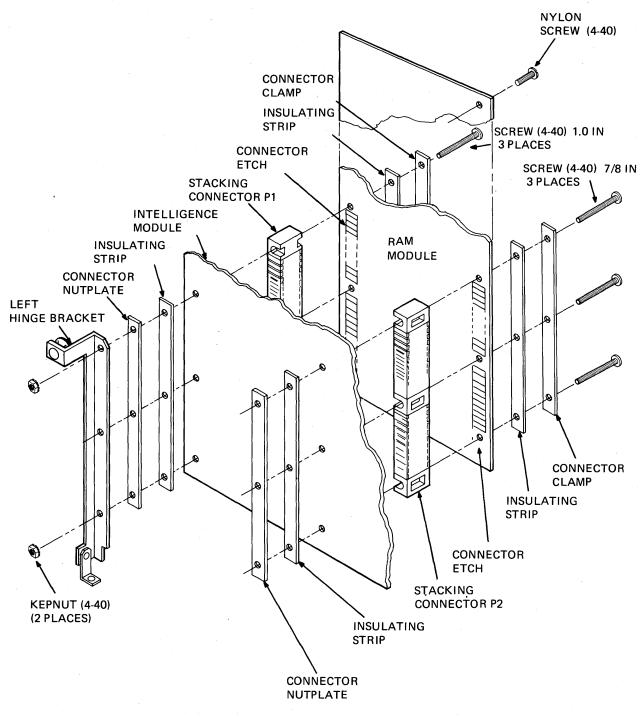
Figure 4-3 TIM Group, Assembly and Disassembly
