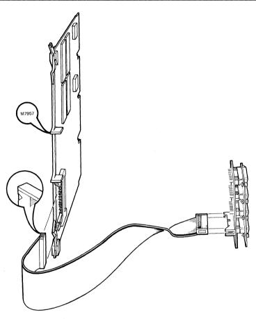
Figure 3-24 DZV11 Internal Cabling
