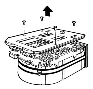
Figure 6-10 Remove the Slide Plate
