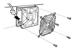
Figure 6-28 Connect the Front Fan Power Cable and Fan Guard
