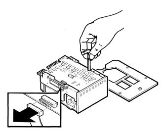
Figure 6-7 RD51 Disk Drive Allen Screws and Connector P5 Removal
