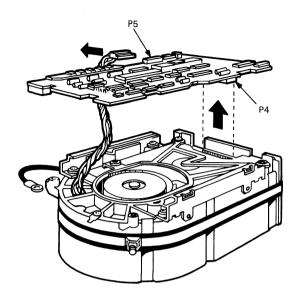
Figure 6-14 Remove the MPCB
