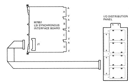
Figure 3-20 DUV11 Internal Cabling
