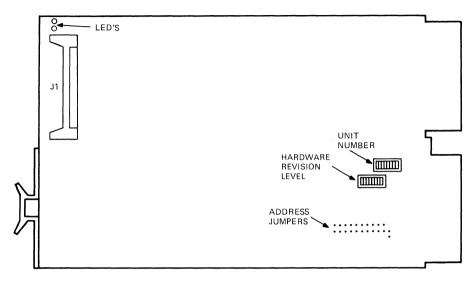
Figure 3-39 M7546 Module Layout
