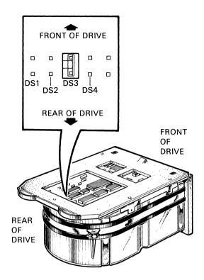
Figure 3-30 RD52 Disk Drive and Jumpers
