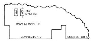
Figure 2-9 +5 VBB Battery Backup Jumper Connections
