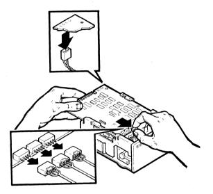
Figure 6-8 RD51 Disk Drive Connectors P6, P7, P8, and P4
