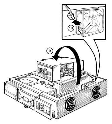
Figure 6-21 Remove Power Supply and Fan Connector
