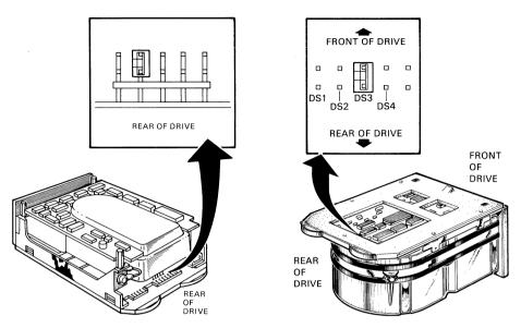
Figure 6-5 Set the RD52 Jumper Clip
