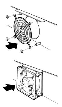
Figure 6-25 Install the Rear Fan
