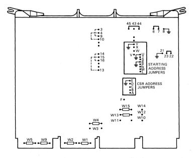
Figure 2-6 MSV11-P Module Layout
