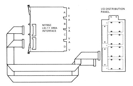
Figure 3-16 DRV11-B Internal Cabling
