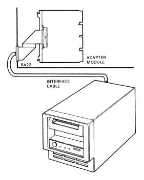
Figure 3-36 TK25 Tape Drive Subsystem
