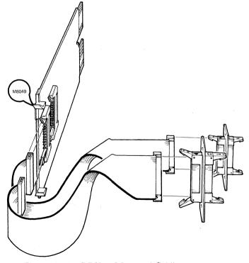
Figure 3-18 DRV11-J Internal Cabling
