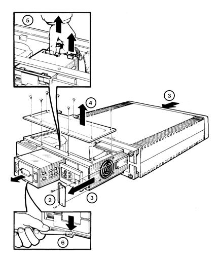
Figure 6-3 RX50 Diskette Drive Removal
