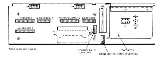
Figure 1-7 Backplane Assembly (Front View from Control Panel Side)
