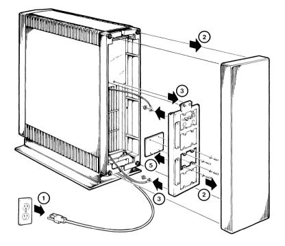
Figure 6-32 Rear I/O Insert Panel Removal
