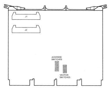
Figure 3-15 DRV11-B Module Layout
