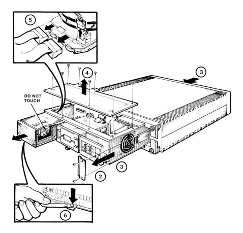
Figure 6-4 RD5n Removal (RD51 Disk Drive Shown)
