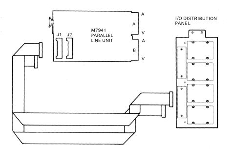
Figure 3-14 DRV11 Internal Cabling
