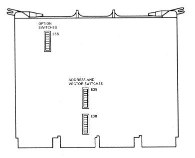
Figure 3-19 DUV11 Module Layout
