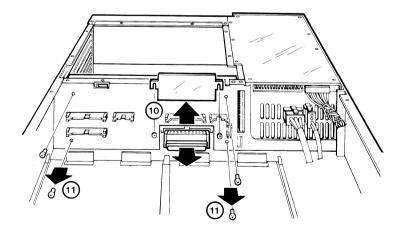
Figure 6-19 Removing the Backplane
