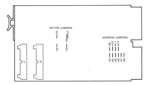
Figure 3-13 DRV11 Module Layout
