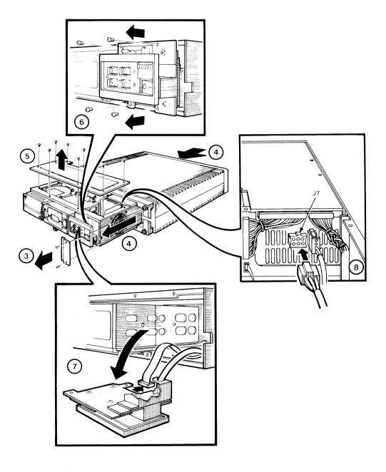
Figure 6-2 Remove the Control Panel
