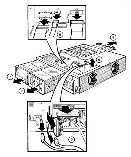
Figure 6-17 Removing Cables and Modules
