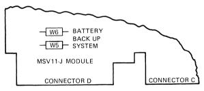
Figure 2-8 +5 V Jumper Connections
