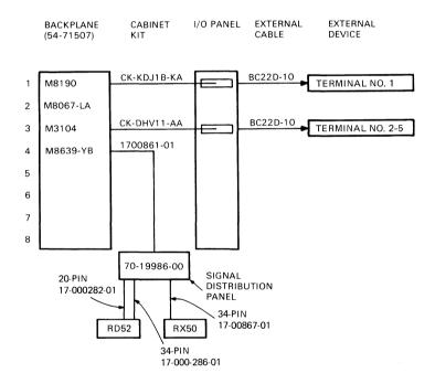
Figure 4-2 Cable Connections for the Base System
