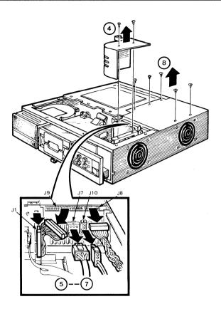
Figure 6-20 Power Supply Removal
