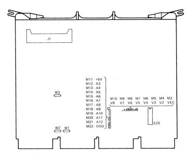
Figure 3-35 RLV12 Module Layout
