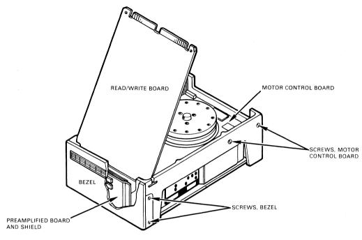
Figure 6-15 RD53 Read/Write Board Removal
