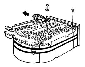
Figure 6-11 Remove the 2-Pin Connector and Screws
