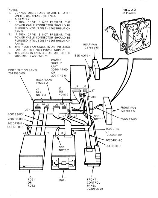
Figure 1-8 Internal Cabling in a BA23 Enclosure
