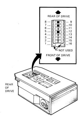
Figure 6-9 DIP Shunt Pack Setting
