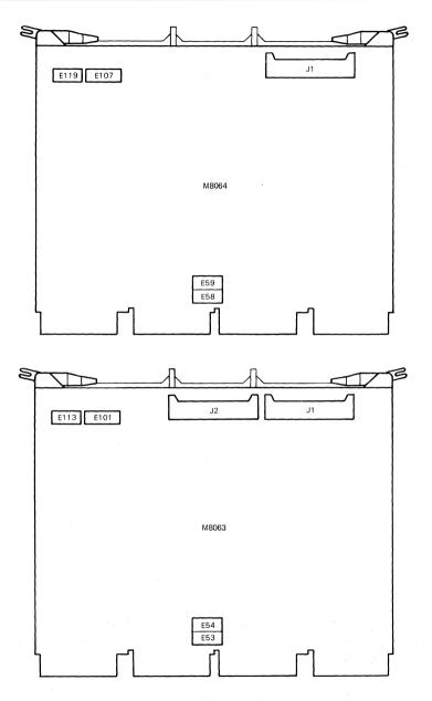
Figure 3-9 DMV11 Module Layout
