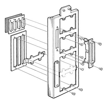
Figure 1-14 I/O Insert Panels and Adapter Plate
