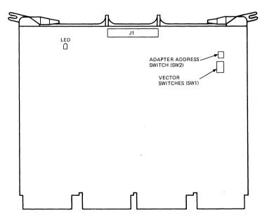
Figure 3-37 M7605 Module Layout
