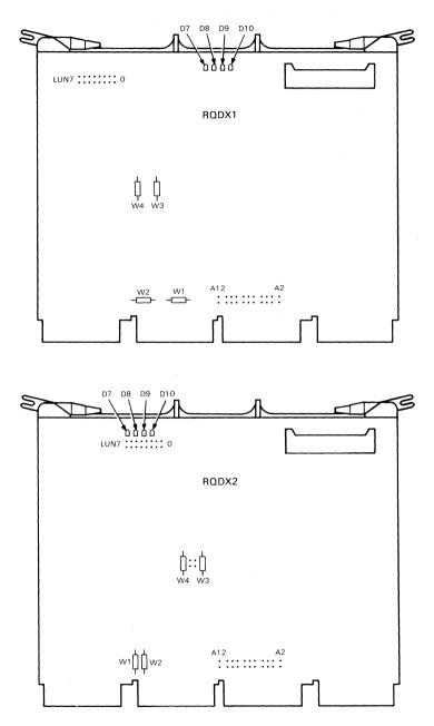
Figure 3-31 RQDX1 and RQDX2 Module Layouts
