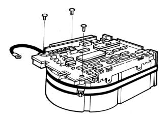
Figure 6-13 Remove Phillips Screws from Heatsink
