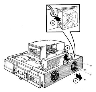
Figure 6-24 Remove the Fan from the Chassis
