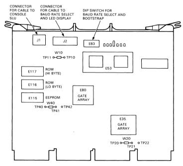
Figure 2-3 KDJ11-B Module Layout
