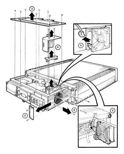
Figure 6-26 Disconnect the Front Cooling Fan
