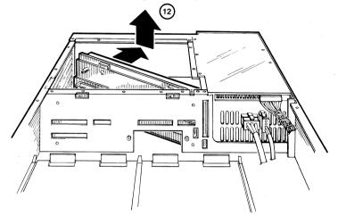
Figure 6-18 Removing Access Cover and Screws
