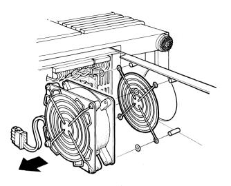
Figure 6-27 Remove the Front Cooling Fan
