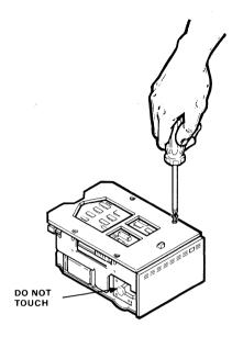
Figure 6-6 RD51 Disk Drive Skid Plate Removal
