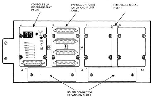
Figure 1-13 Rear I/O Distribution Panel (KDJ11-B SLU Display Panel Shown)
