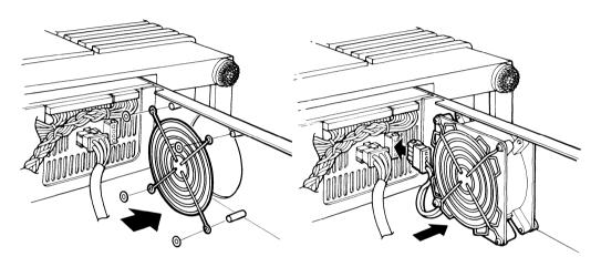
Figure 6-29 Install Replacement Fan
