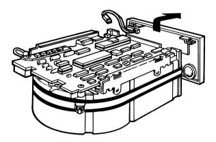
Figure 6-12 Remove the Front Bezel
