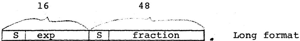
The radix point is to the right. The exponent and the fraction are 2's complement numbers. The normalization is binary.
