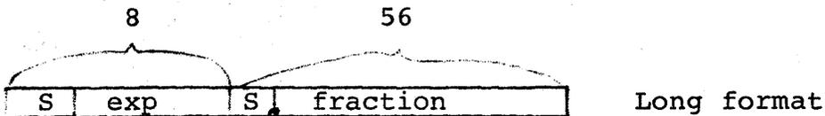
In order to get the required exponent range with the above format, quad normalization (i.e. radix = 4) has to be used. Considering the PDP-11/20 instruction set quad normalization is practically as difficult as hex normalization. Furthermore, by not having the classical layout of Figure-1 the economy of sharing some 32-bit integer with 32-bit floating point instructions is lost.
