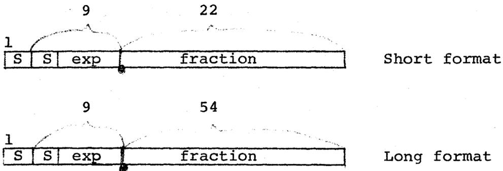
Because of the 9-bit exponent binary normalization can be used to get the required exponent range. Considering the PDP-11/20's byte oriented instruction set, packing and unpacking of this format is more difficult.
