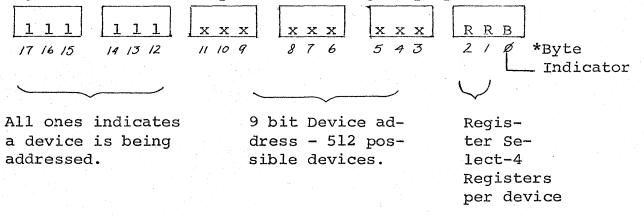
\*The Byte Indicator would be used for character oriented devices such as TTY.
