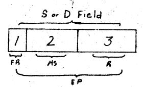
The locations of the SYP (source byte pointer) and the DYP (destination byte pointer) are determined by the contents of the EP's of the S and D fields of the instructions. The free bits "FR" are used to allow for incrementing the byte pointer.
