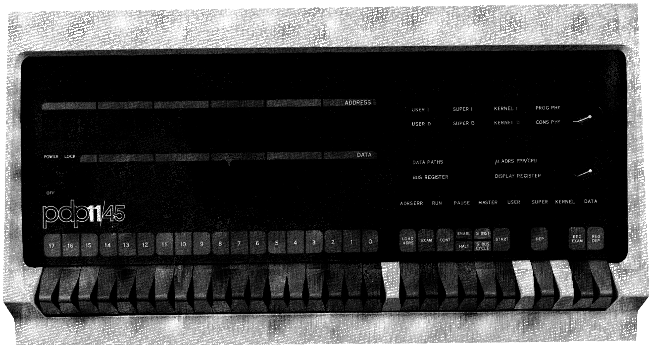
Figure 4-1 PDP-11 Switch Register Console
